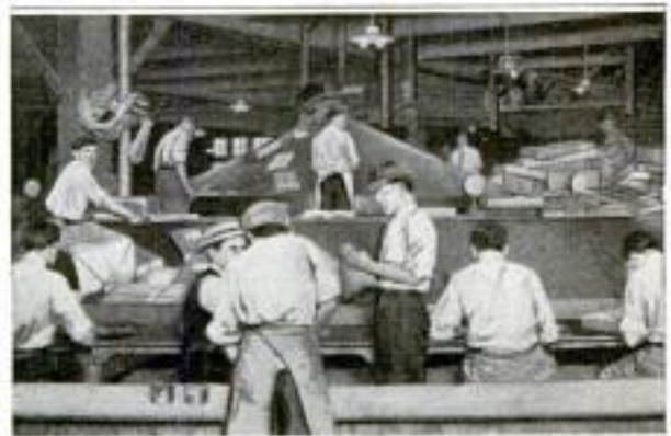
Revolving Cone Which Enables Express Clerks Rapidly to Distribute the Addressed Packages Dropped upon It, to the Proper Waybill Employes Seated at the Encircling Line of Desks
