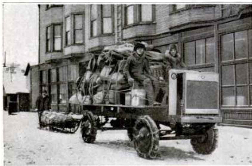
Four-Wheel-Drive Truck Employed in Nome and Vicinity in the Place of Dog Teams to Transport United States Mail. The Dog Sled at the Rear was Used as a Trailer Shortly before the Holiday Season, When the Mail Was Very Heavy
