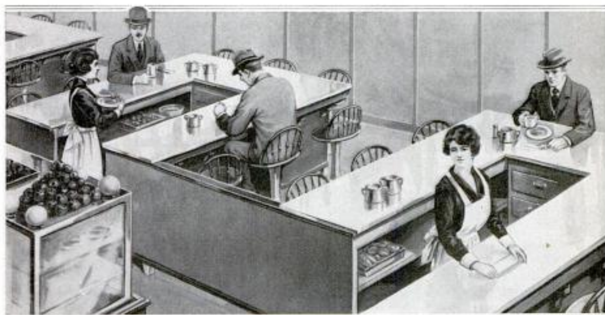
Novel Arrangement of Seats in a Chicago Lunch Room: Each Waitress Has Nine Customers to Serve and a Clear Space to Work between Them. The Plan was Designed by the Proprietor
