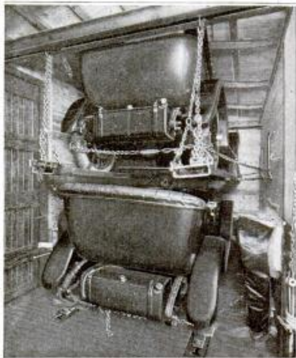
In This New Freight Car for Autos the Windlasses Seen at the Right and Left are Used to Hoist the Upper Auto onto Its Platform of Channel Irons
