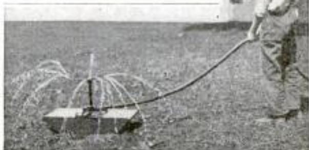
Galvanized-Iron Base for a Lawn Sprinkler: With This Sledlike Support the Sprinkler can be Drawn from Place to Place While the Water is Running
