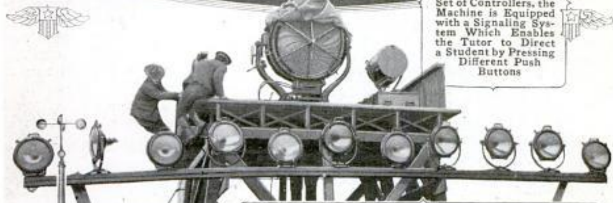
This Battery of Searchlights is an Important Part of the Equipment at Mineola. When Flights are being Made at Night the Small Flood Lights are Used to Guide the Airmen and Help Them in Making Safe Landings
