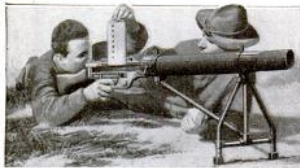
Operating a Machine Gun with New Continuous-Feed Magazine: Above, the Assistant is Seen Feeding Cartridges into the Hopper; Should the Assistant be Wounded, One Man can Operate the Gun, as in the Lower Photograph
