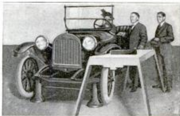
Teaching a New Owner How to Drive Her Car: Note the Series of Small Levers near the Instructor's Left Hand, Which Raise Signals at the Other End of the Table for the Pupil's Guidance
