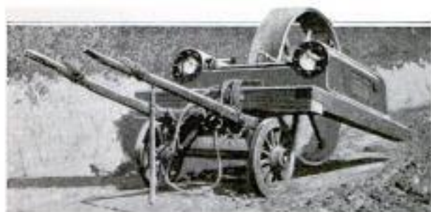
A Heavy Air Compressor being Transported through a Mountainous Region in South America, Supported by Its Own Belt Wheel and a Heavy Cart
