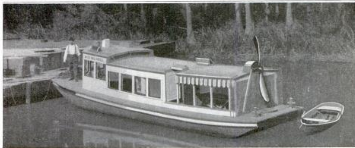
This Boat Draws Only Eight Inches and Makes a Speed of Fifteen Miles an Hour in the Shallow Streams of Texas, with the Aeroplane Propeller Seen at the Stern. The Builder is Standing on the Forward Deck
