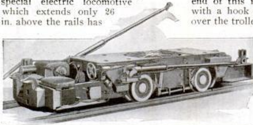
This Locomotive Weighs Two and a Half Tons, Is 26 Inches High, and Pulls a 50-Ton Load Easily. It was Built Especially for Use in a Coal Mine Whose Galleries Are Exceptionally Low
