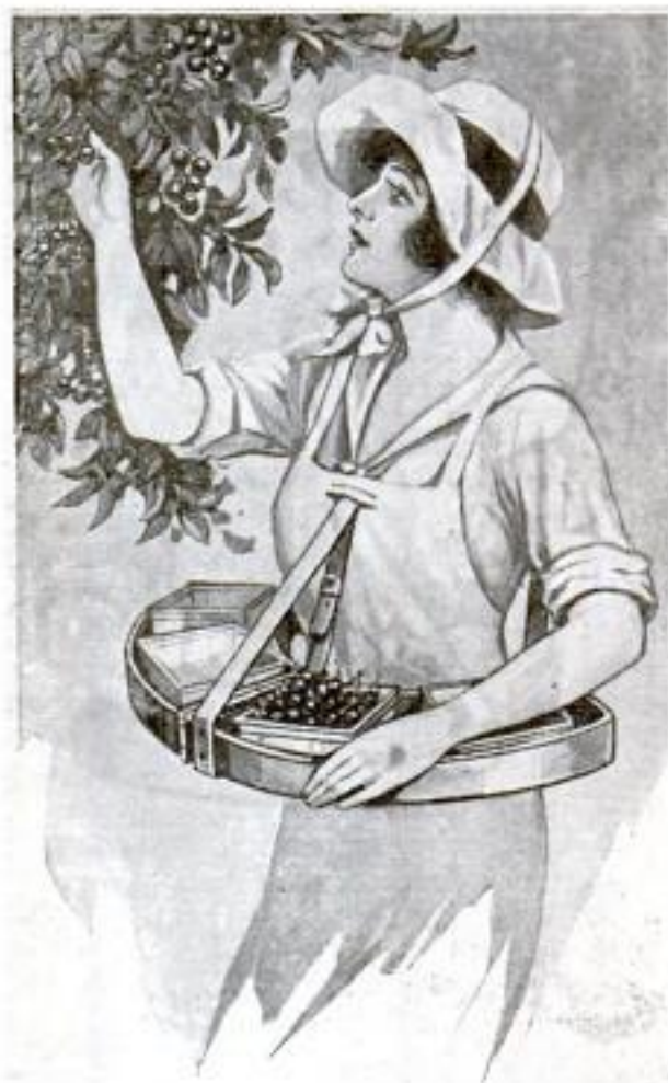
Fruit Picker's Curved Tray Having Raised Edges and Held in Place by Shoulder Straps so That Both Hands can be Used in Picking
