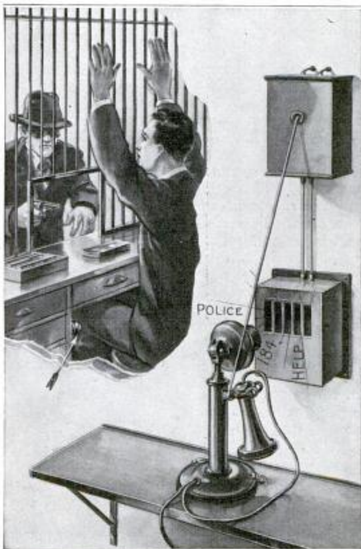
A Burglar Alarm That Talks: The Button near the Cashier's Knee Enables Him Secretly to Set the Phonographic Alarm to Operating in an Adjoining Room
