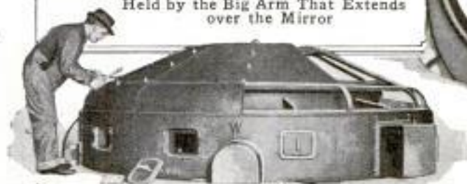
Felt and Cork Insulate the Steel Housing of the Reflector at the Base of the Telescope Tube, While Water from a Large Tank, in Which the Temperature is Automatically Controlled, is Circulated in Coils around the Mirror
