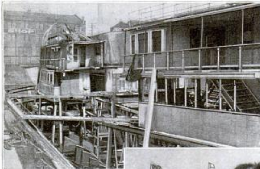
Boat Cut in Two Amidships, Preparatory to Inserting a 40-Foot Section of New Hull
