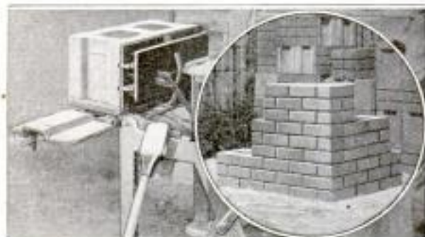
Concrete-Block Machine Having a Faceplate with Removable Ribs Which Make Each Block Appear to be Composed of Several Small Ones
