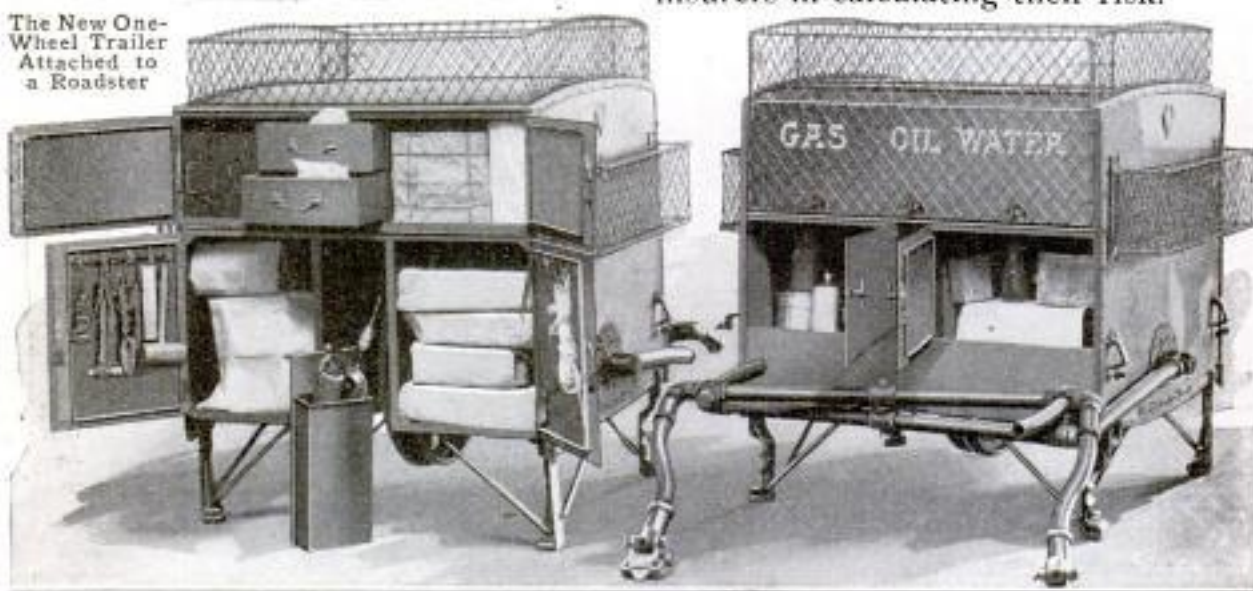
Above at the Left is Given a Rear View, and at the Right a Front View, of the Interior Arrangement of the Trailer as Outfitted with Tanks, Drawers, and Compartments for the Overland Tourist
