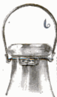
6 Patented Wire Handle for Milk Bottle That Enables Latter to be Hung Out of Reach of Animals When Delivered. Can be Made for 15 Cents a Dozen
