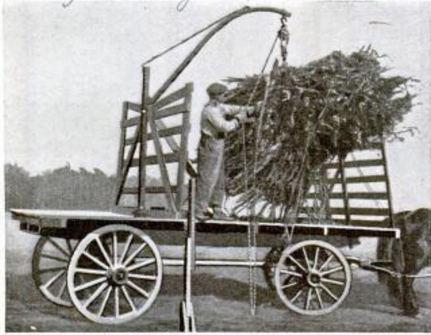
A Small Adjustable Crane with Which One Man can Load and Unload Big Shocks of Corn, Bales of Hay, and the Like, without Difficulty
