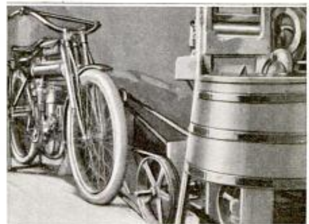
FIG. 2 The Work of Wash Day Made Lighter by the Belting of Motorcycle to the Washing Machine and Wringer
