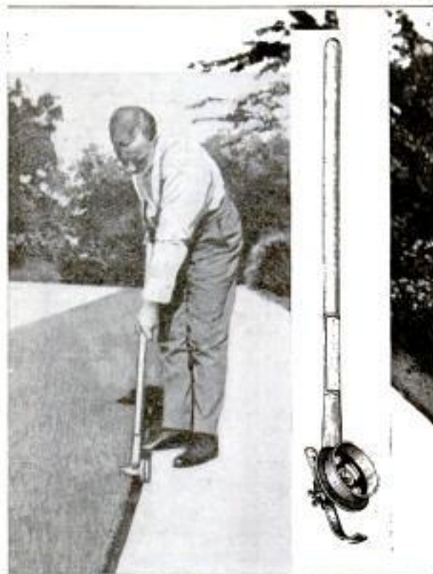
The Wheel Follows the Outer Edges of a Sidewalk so That the Knife Cuts a Straight Groove
