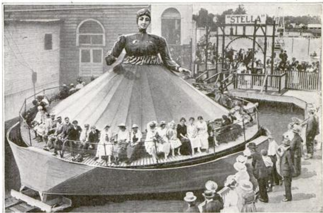
Huge Figure Called the "Tango Girl" Which Sways Its Patrons from Side to Side and Whirls Them Around as It Moves down the Track
