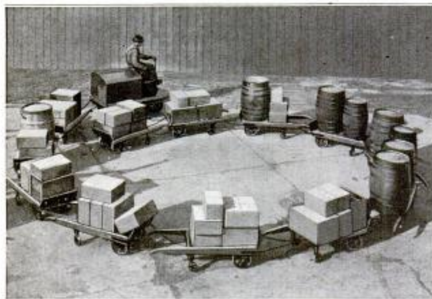
A Train Composed of Hand Trucks Equipped with Casters and Coupling Devices Which Make Each Unit Follow in the Track of the One Ahead
