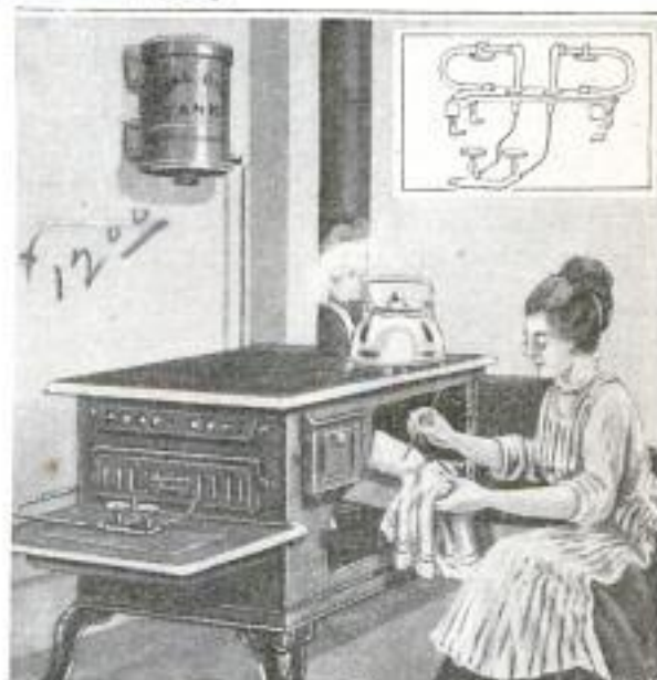
Cooking with Gas Made in a Coal Stove. The Kerosene Supply Tank is Seen on the Wall and Regulating Valves on the Ledge of the Stove. The Insert Shows Details of the Burner Set in the Fire Box.
