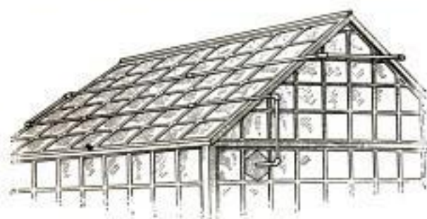
Damage to Glass Roofs was Avoided by Melting the Snow in a Heavy Snowfall as It Drifted on the Roof
