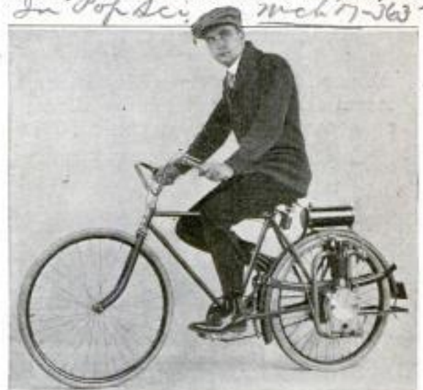
An Ordinary Bicycle Converted into a Motorcycle by Substituting a Newly Invented Motor Wheel for the Original Rear Wheel
