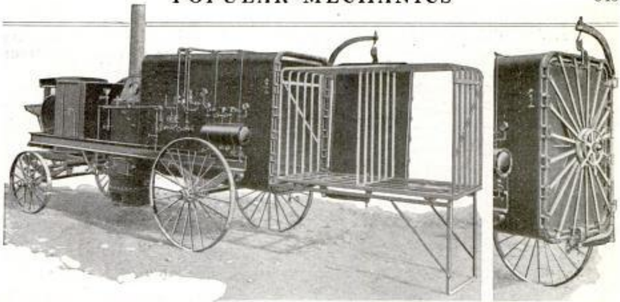
Six of These Portable Disinfesting Outfits have been Purchased for the United States Army. Either Dry Steam, or Formaldehyde and Ammonia can be Used as a Germicide. A View of the Air-Tight Door is Shown at the Right
