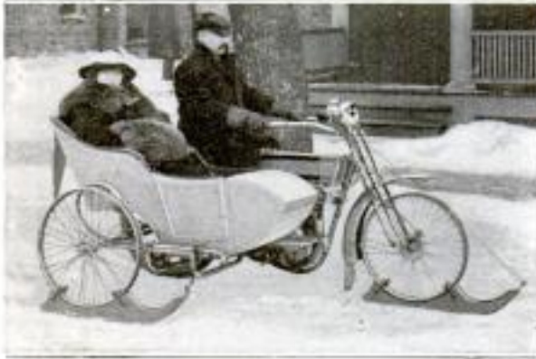
Motor Sleigh Contrived by an Inventive Canadian When the Snow Was Too Deep to Run His Motorcycle: A Neat Arrangement of Runners Bolted to the Bare Rims
