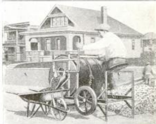
A Concrete Mixer, Having a Capacity of from Three to Five Yards of Mortar, Which is Operated by Foot Power
