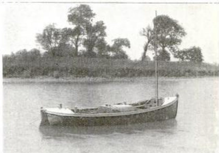
Seaworthy Motor Lifeboat Built in England and Designed More Especially for Towing than Carrying Purposes. It will be Used by an Ocean-Going Passenger Vessel
