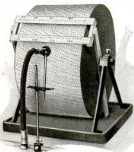
Mechanism of the Tonoscope, Showing the Revolving Screen Which Indicates the Pitch of Musical Sounds
