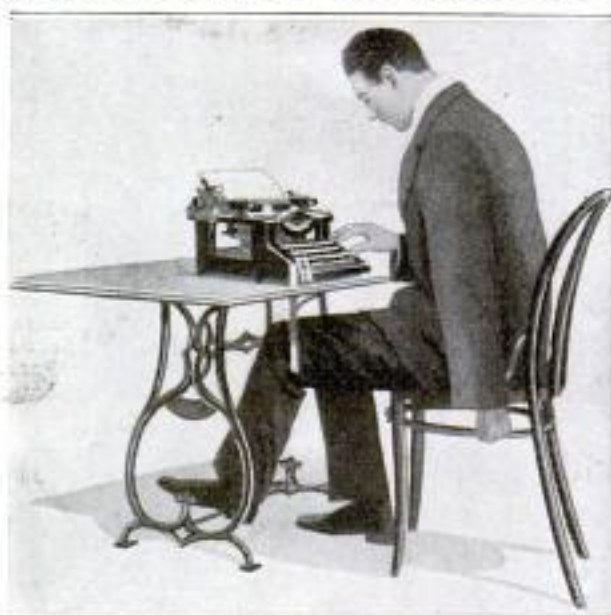
BY COURTESY OF OFFICE APPLIANCES Here Is One of the Special Typewriters That have been Devised for Crippled Men: It can be Successfully Operated with One Hand and a Leg
