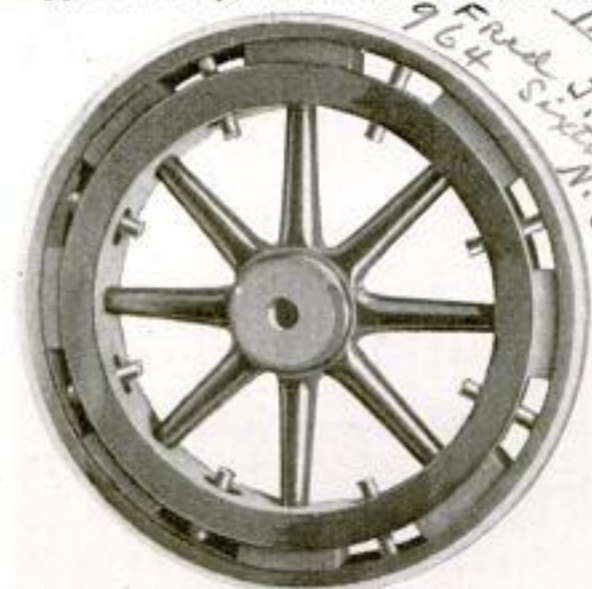
A Substitute for a Rubber-Tired Wheel Having a Rim of Steel Which Rests on Cushions Placed at the Ends of the Spokes
