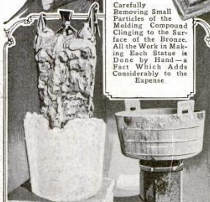
Wax Replica Covered with Molding Compound, More of Which is to be Added. After the Outer Coating has been Completed the Object is Baked and the Wax Melted Out and Replaced by Bronze
