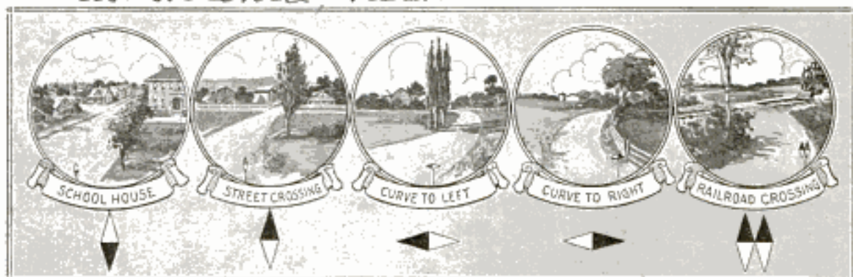
Different Ways of Mounting the Sign so as to Apprise Motorists of Just What to Expect on the Road Ahead are Illustrated beneath the Drawings Presented Above. General Adoption of the System would Eliminate the Ununiform and Confusing Devices of Various Forms Now Used
