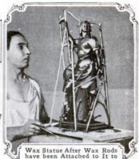
The Various Wax Parts Assembled, Forming a Duplicate of the Bronze Figure to be Cast
