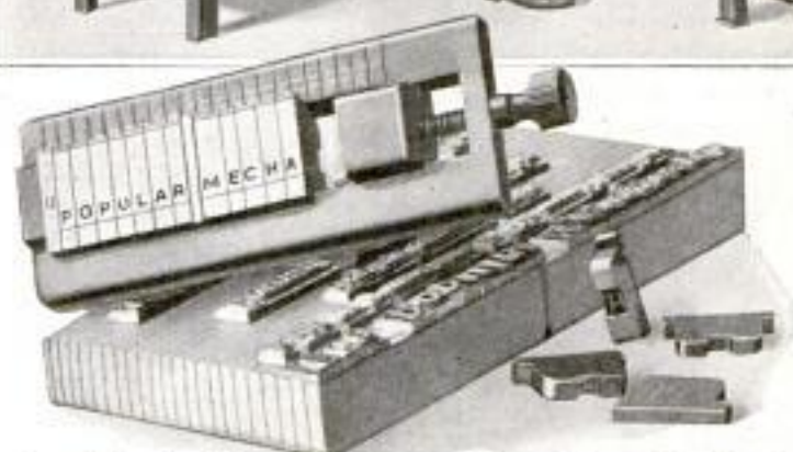
One of the New Type Machines in Use, and at the Left, the Matrix Cabinet. Below is Shown a Partly Filled Stick, Turned Over so That the Type Matter can be Read from Left to Right, Each Matrix having the Letter It Casts Stamped on the Back. Beneath It is a Form Made Up of Slugs Cast by the Machine
