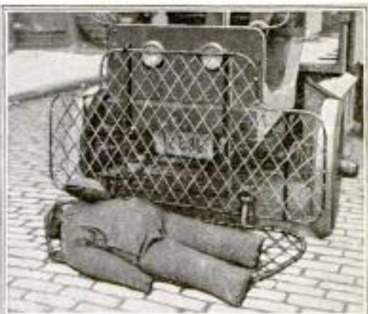
Manual Pickup of a Prostrate Man-Size Dummy in Official Test of New Safety Fender for Motor Trucks in New York. The Fender can be Operated by the Driver, but Also Works Automatically. When Not in Use, It Folds Up, as Seen at the Left
