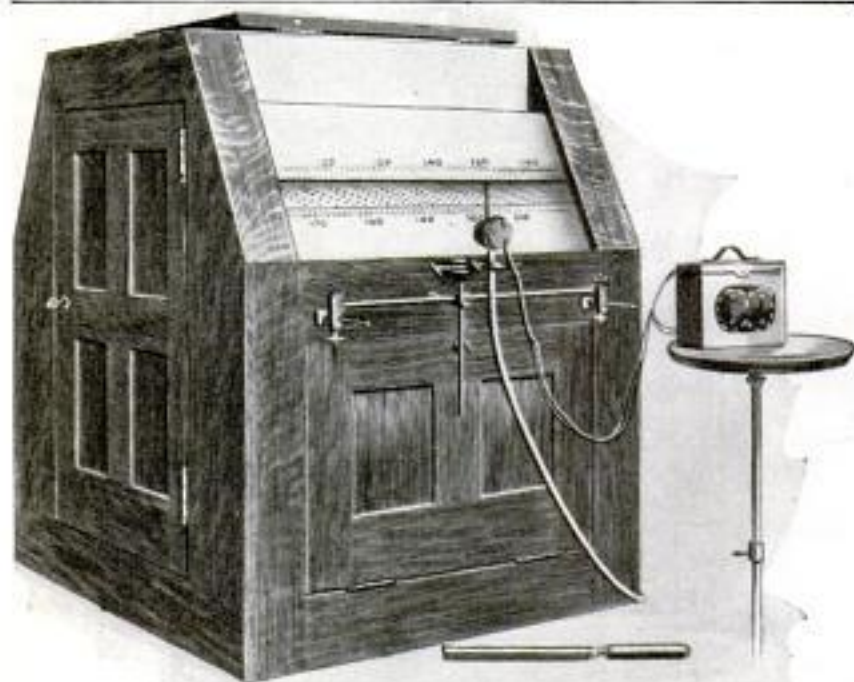
Improved Model of the Tonoscope, by Which the Deaf may Teach Themselves to Sing and Play Correctly, without an Instructor
