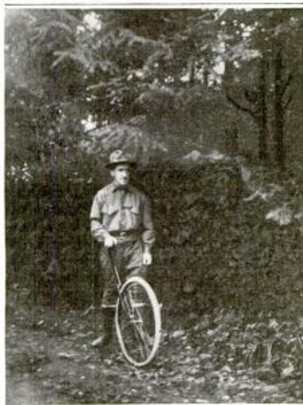
A Bicycle Wheel Equipped with a Handle and Cyclometer, with Which a Forest Ranger can Measure More Trail in the Same Time, than Two Men with a Chain, and can Do It More Accurately
