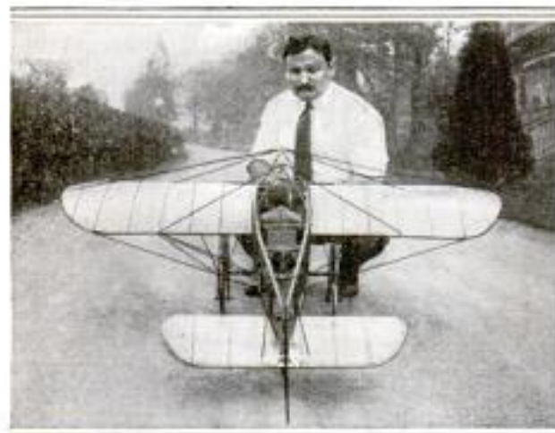
Two Views of a Model of the Monoplane in Which Blériot First Crossed the English Channel: The Machine Is Five Feet Long and Five Feet Wide and Weighs Eight Pounds without the Motor
