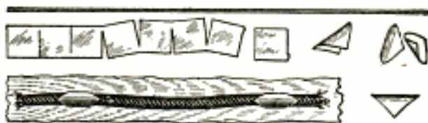
The Strip is Cut into Squares Which are Folded and Driven into the Support, Binding the Wire
