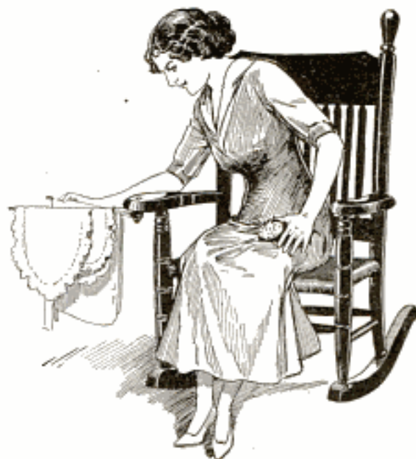
The Swinging Rack Folds under the Arm of the Chair When Not in Use
