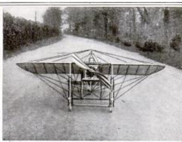
Two Views of a Model of the Monoplane in Which Blériot First Crossed the English Channel: The Machine Is Five Feet Long and Five Feet Wide and Weighs Eight Pounds without the Motor
