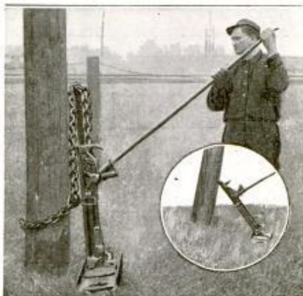
Telephone, Trolley, or Lighting Poles are Pulled or Straightened in a Few Minutes by the Aid of This Pole Jack
