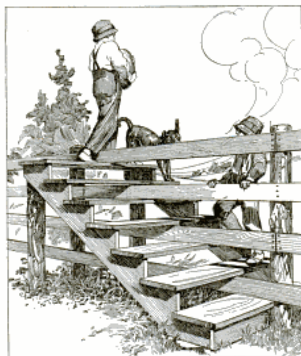
The Stairs Built into the Fence Provides a Convenient Method of Climbing over the Barrier
