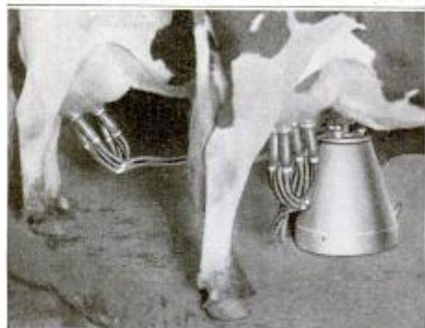
One Man can Milk 18 to 30 Cows an Hour with This Double-Unit Milking Machine, Which is Operated by a Vacuum Pump
