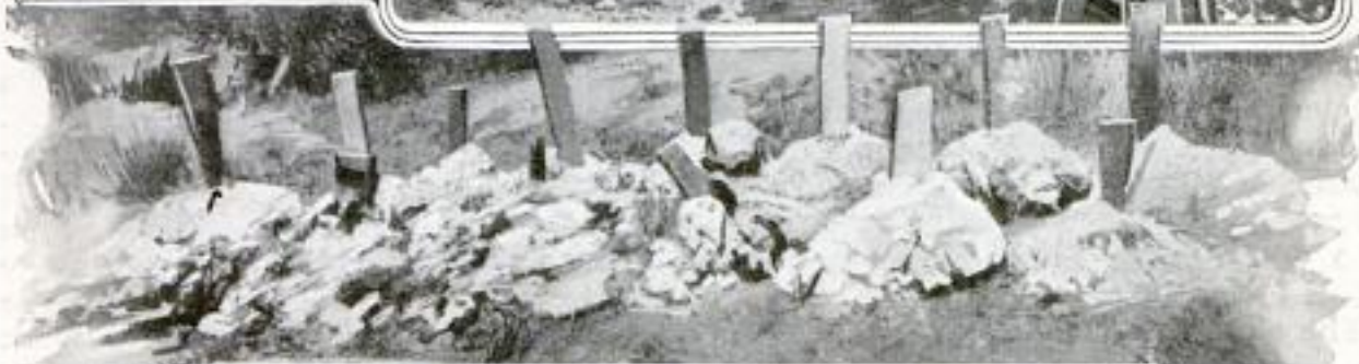
Samples of Earth, Rock, and Ore from One of the Bores; Specimens are Taken Every Five Feet as the Drilling Progresses, and Marked with Paddles on Which the Depths are Recorded. When Traces of Ore are Struck, Samples are Taken Every Three Feet
