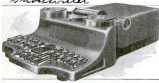
A Machine Which Writes Shorthand: The Code Used is so Simple That One can Learn to Read It in a Few Minutes. The Characters are Printed on a Paper Ribbon, a Word to a Line
