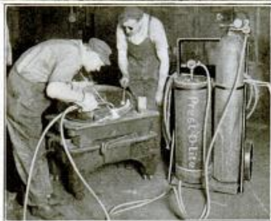
Above shows the Prest-O-Lite Process as used for making an "on the spot" repair in shops of P. F. Collier & Co., New York City, publishers of "Collier's Weekly."
