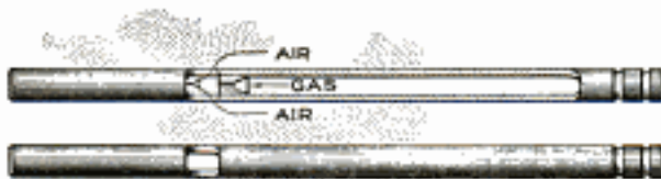
The Use of This Easily Made Blowpipe Obviates the Difficulty of One Operated by the Breath
