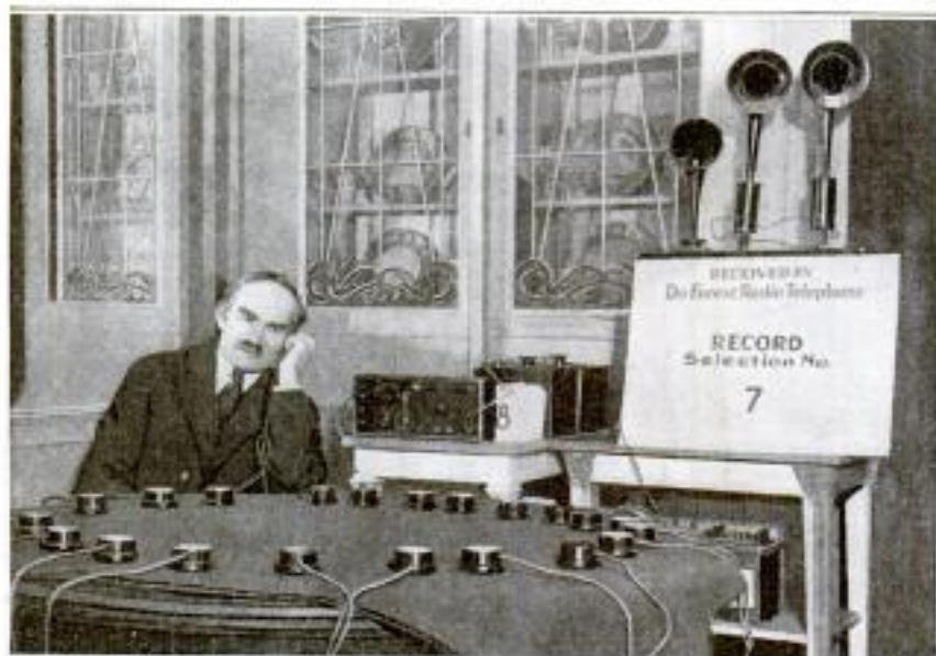
Dr. Lee de Forest and His Wireless Telephone Apparatus Which was Used in Entertaining a Company of Banqueters Recently. With This Equipment Selections Played on a Phonograph in a Distant Studio could be Heard Distinctly
