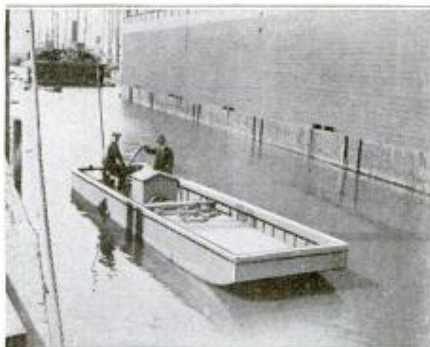
A Boat Having a Propeller Located in a Tunnel Chamber: When Carrying a Load of 6,000 Pounds It Draws But 15 Inches of Water
