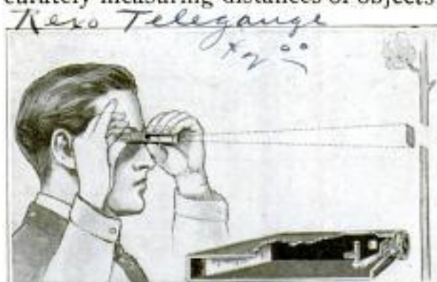
When the Two Images Seen Coincide, a Pointer in the Thumbscrew Indicates the Distance
