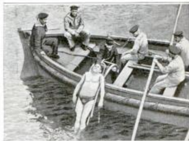
Taking a Drowning Person from the Water with a Rescue Ladder, Easily Hoisted by Its Towline and Pulleys
