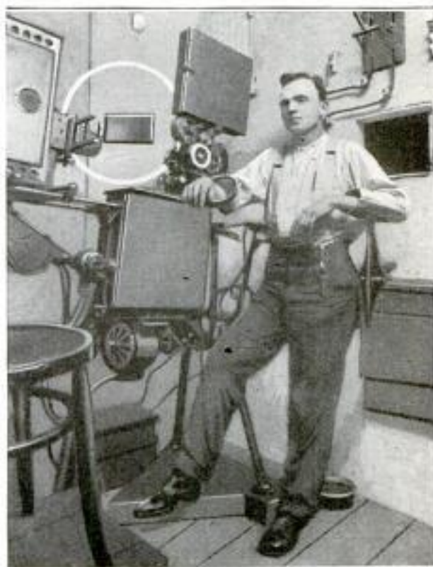
A Colored-Glass Screen Fastened to the Front of the Lamp House Enables the Operator to Watch the Beam of Light, Where It Strikes the Film, without Eyestrain
