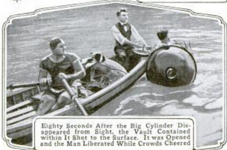
The Vault is Intended as a Nonsinkable Depository for Registered Mail, Jewels, and Valuable Articles Owned by Steamer Passengers. The Illustration Shows What would Happen if a Ship So Equipped should Founder
