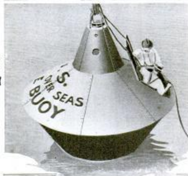
Below: Steel Top-Shaped Buoy Which can Shelter 40 Persons and Also Enough Provisions to Supply Them Several Days. Above: View of the Life Buoy, Showing Anchor That Serves as a Ballast and Is a Means of Keeping the Buoy Upright in the Roughest Sea
