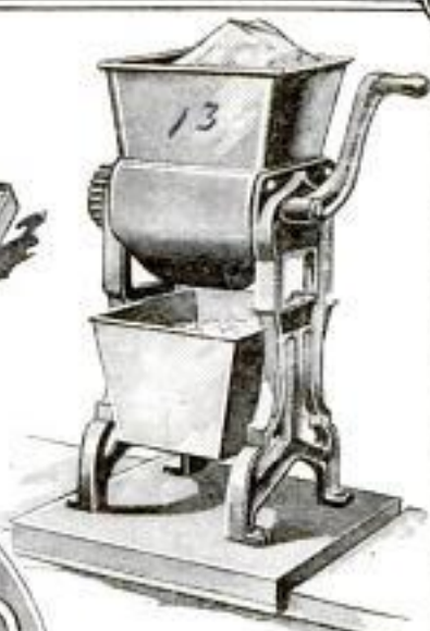
Machine Cuts Ice in Small Diamond-Shaped Pieces for Table Purposes without Wasting It or Chilling One's Hands
