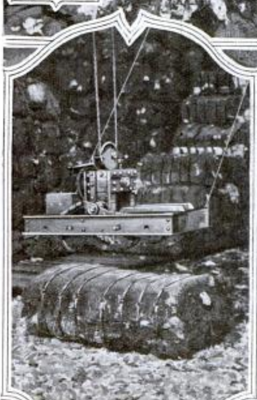
The Grappling Section of the Overhead Conveyor About to Pick Up a Bale That has been Withdrawn from Pile at Left
