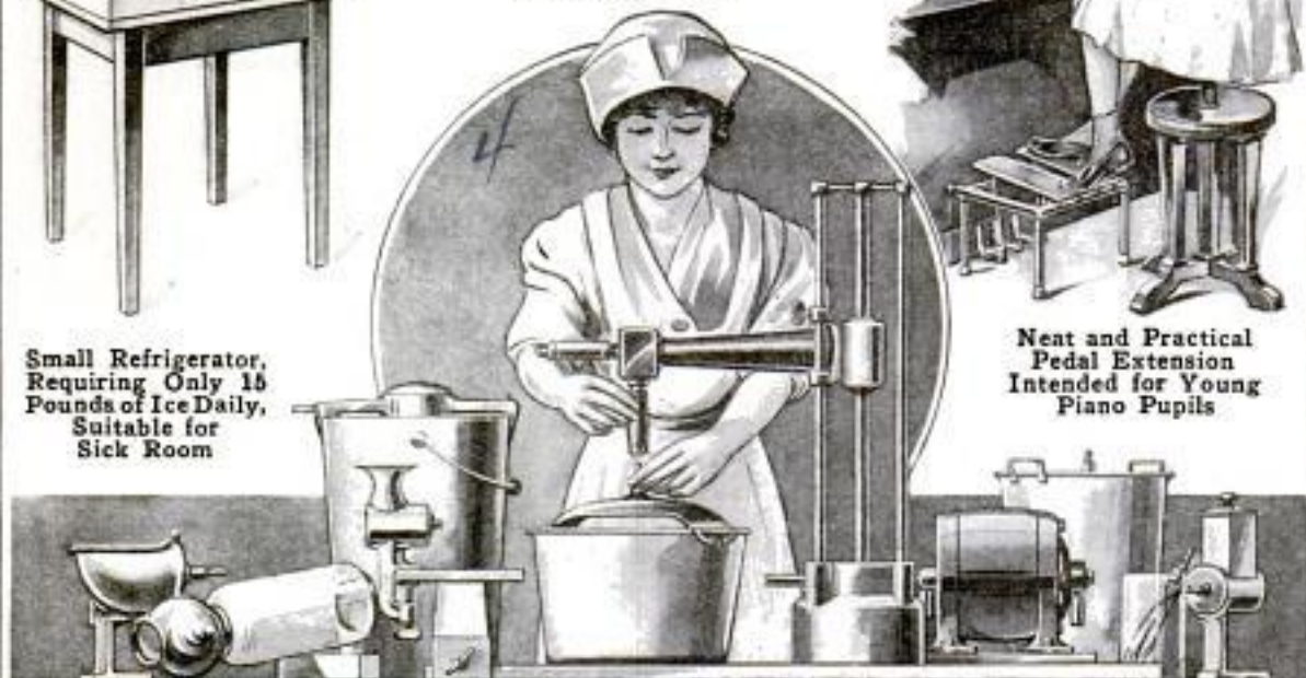
By Removal of Cranks All Hand-Operated Kitchen Appliances are Driven Electrically with This Power Plant
