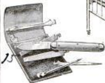
Pocket Tool Kit, Consisting of Knife, Chisel, Gimlet, Screwdriver, File, Reamer, Bottle Opener, and Rule
