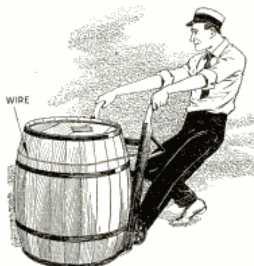
The Hoop Prevents the Load from Tipping off the Truck
