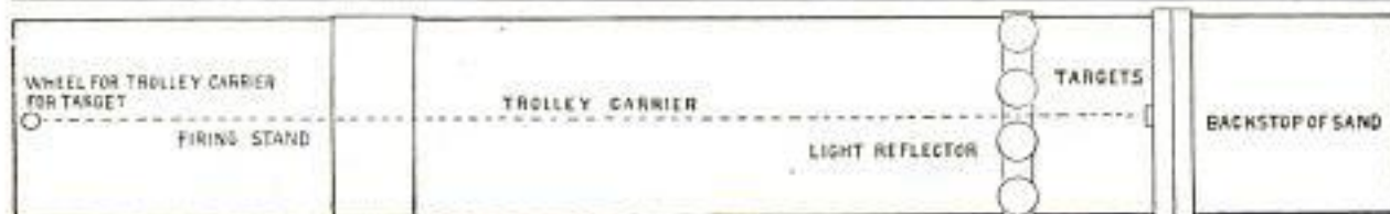
The Target in This Rifle Range can be Drawn Up to the Marksmen, Thus Making It Unnecessary to Walk Out in Front of the Firing Stand to Determine the Score
