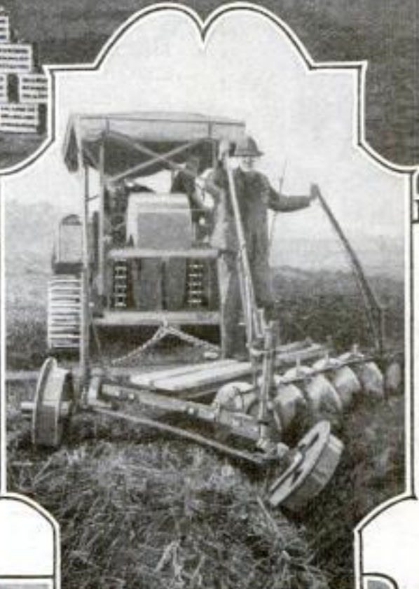
A Five-Gang Plow, Hauled by a Caterpillar Tractor, Cultivating Some of the Reclaimed Muck Soil Which has Recently been Cleared of Timber
