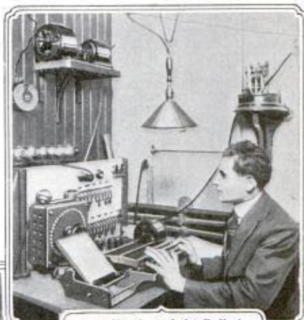
Any Number of the Bulletin Machines, Situated Miles Apart, may be Operated Simultaneously by This Keyboard
