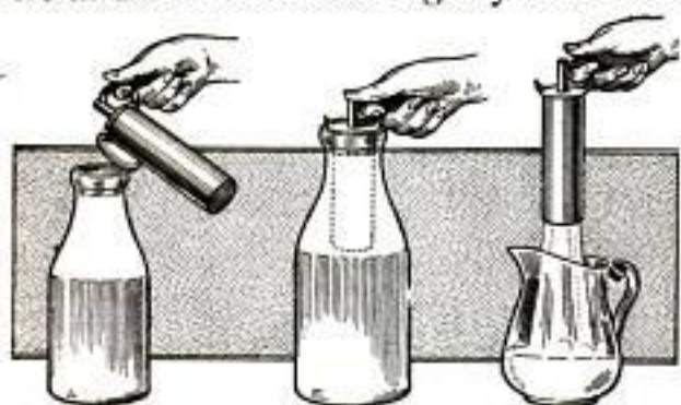
A Simple Utensil with Which Cream may be Removed from a Milk Bottle without Mixing the Cream with the Milk
