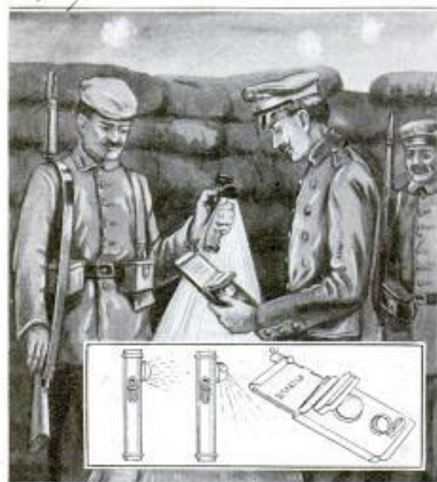
A Pocket Flash Light Used by German Soldiers, the Bulb, Lens, and Reflector of Which Move in Unison with the Hood When It is Drawn Up or Down, and a Combination Pocket Lamp and Holder for Compass, Maps, and Dispatches, Used by German Officers
