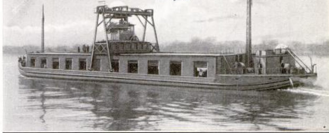
The "Inco No. 1," the First of a Large Fleet of Motor-Driven Steel Barges with Which It is Expected to Restore Shipping on the Mississippi River
