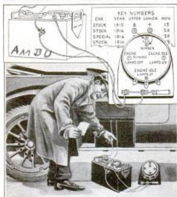
Determining the Class of Trouble Present in the Electric System of a Car by Using the "Fault Finder"
