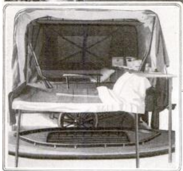
The Automobile Trailer Ready for Campers, with Canopy Folded Back, Showing Two Beds, Table, and Shelf
