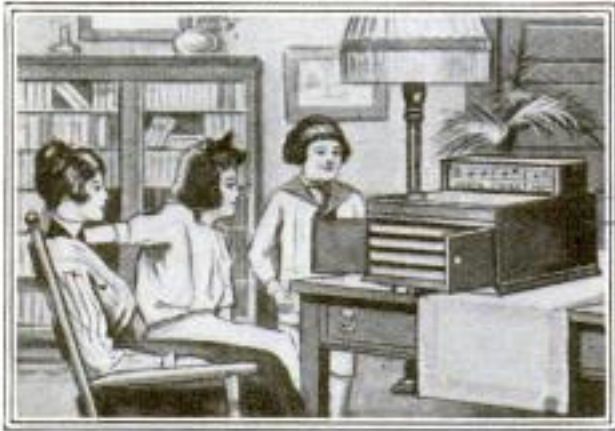
The Music and Words of a Selection Appear on the Tape Which Moves from Right to Left in Synchronism with the Record as This is Played
