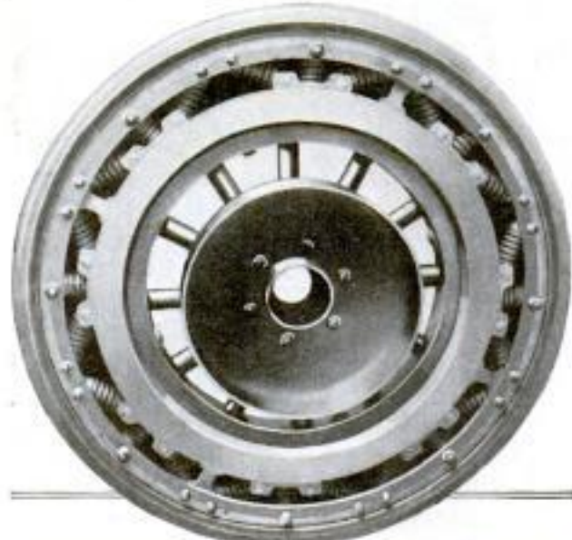
This Resilient Rim can be Fitted to Any Wheel by Shortening the Spokes and Reducing the Diameter of the Felly
