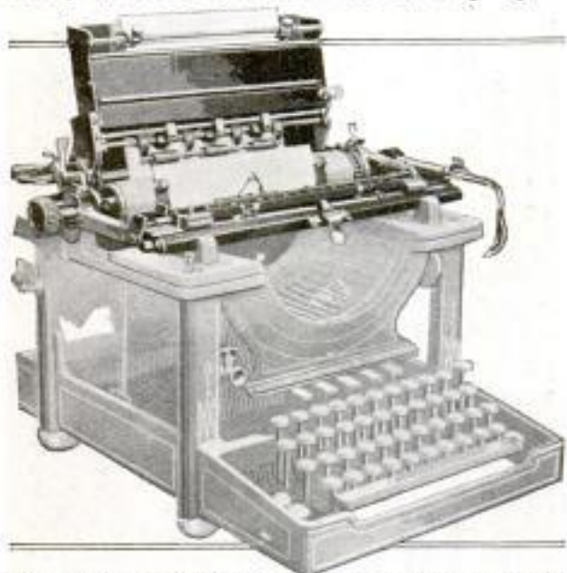
With This Attachment Envelopes or Cards are Fed to a Typewriter Automatically so That an Operator can Address Several Times as Many Pieces as by the Old Method
