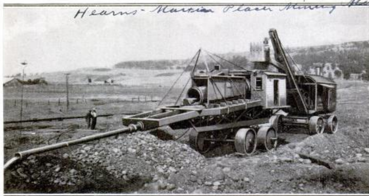
This Machine, Which Uses a Comparatively Small Amount of Water, Works Placer Deposits Profitably Where Streams Are Scarce
