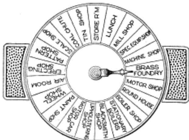
When the Foreman Leaves His Desk He Indicates Where He may be Found
