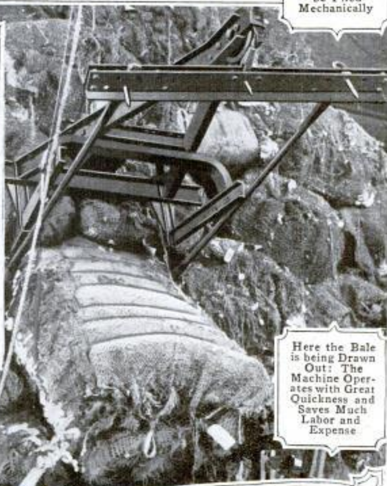
Raising a Bale Preparatory to Conveying It to Another Compartment Where It will be Piled Mechanically
