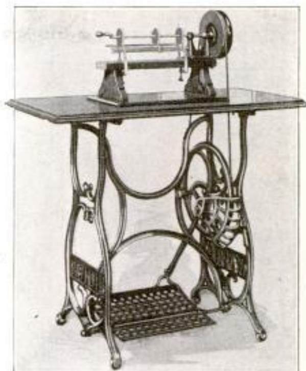
A Device, Mounted on a Sewing-Machine Frame, on Which Bandages of Various Widths can be Wound
