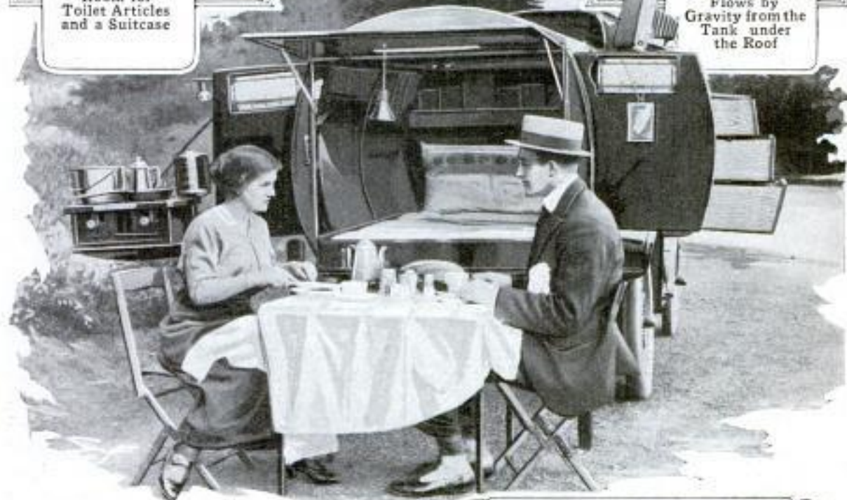
"All the Conveniences of Home"; The Collapsible Automobile Camping Outfit Showing the Berth Made Up, the Chest of Drawers, the Kitchen Equip- ment, and the Dining Arrangement. Below: The Camping Outfit Closed
