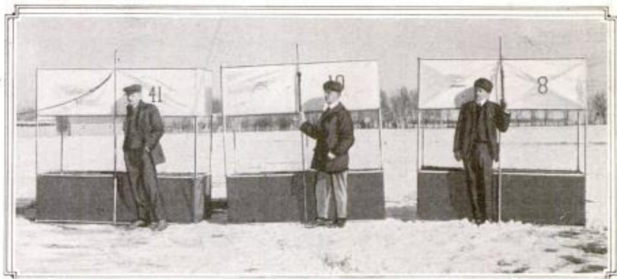
String of Three Kites Used at the Nebraska Aerological Station: The Cloth at Top of Each is White and That at the Bottom Black. Thus They Are Visible Whether Flying against a Light or Dark Cloud
