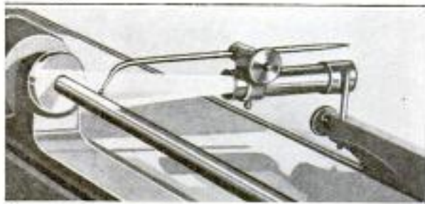
When the Point of the Needle Comes in Contact with a Raised or Irregular Place on a Piece of Work a Connection is Made and the Tiny Lamp Ignited
