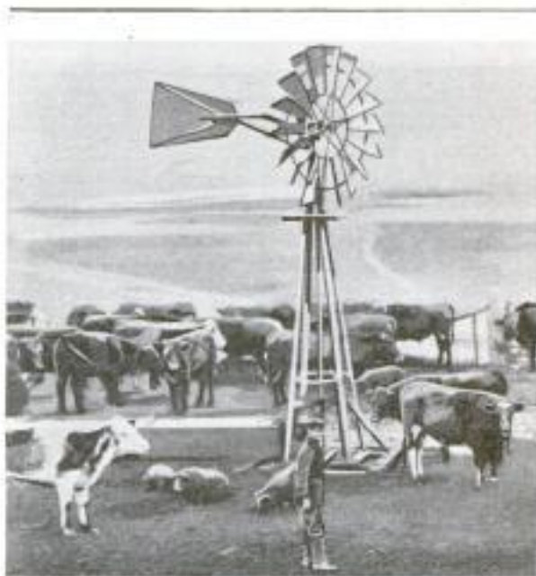
The Windmill is Mounted on Skids and may be Moved from One Point to Another without Difficulty
