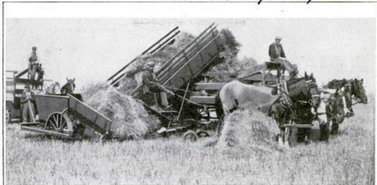
With This Grain Loader Fewer Wagons are Needed to Supply Grain to a Threshing Machine and No Laborers are Required to Pitch Bundles onto the Wagons
