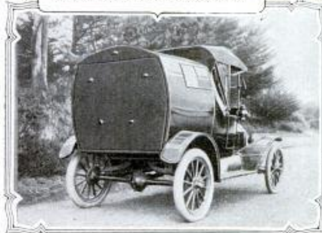
"All the Conveniences of Home"; The Collapsible Automobile Camping Outfit Showing the Berth Made Up, the Chest of Drawers, the Kitchen Equip- ment, and the Dining Arrangement. Below: The Camping Outfit Closed
