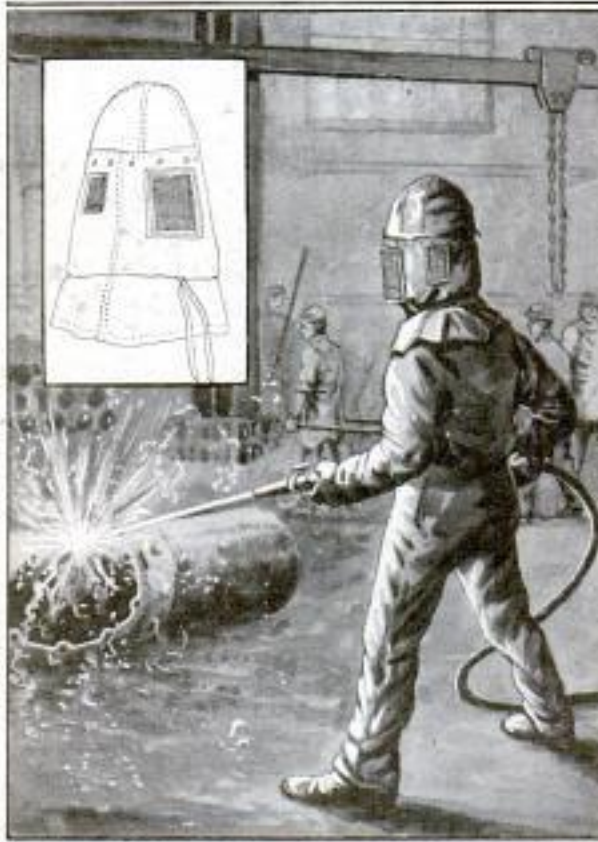
By Wearing the Mask over the Head a Sand Blaster Escapes Much of the Danger of His Work
