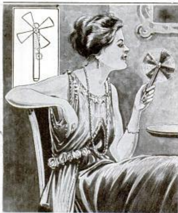
By Turning the Wheel under the Thumb the Radiating Blades of This Mechanical Fan can be Made to Revolve Rapidly
