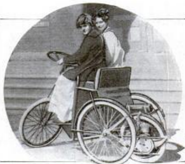
This Vehicle is Constructed Chiefly from Parts of Old Bicycles and will Carry Two Passengers at the Rate of Seven Miles per Hour on Level Roads
