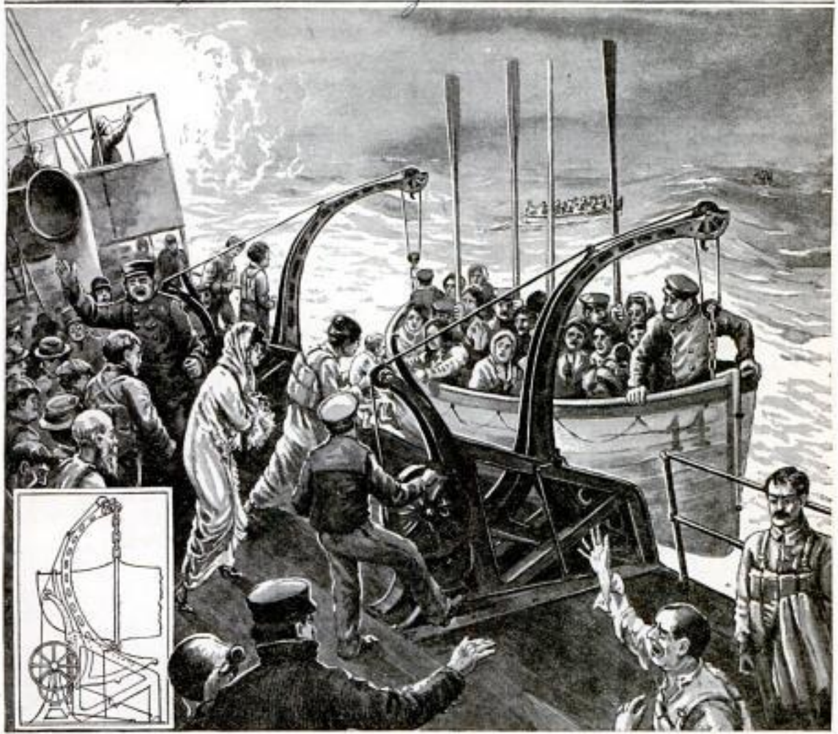
Automatic Davit Lowers Boatload in Less than One Minute's Time through Aid of Quadrant Arms Supported upon Rocker Base
