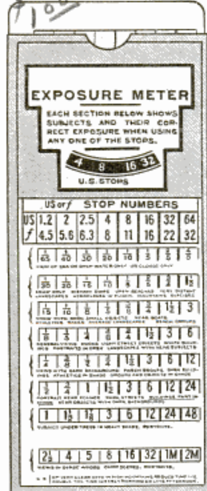
The Device Gives the Time Necessary for All Classes of Subjects with Any Stop Desired, Enabling a Beginner to Make Good Photographs
