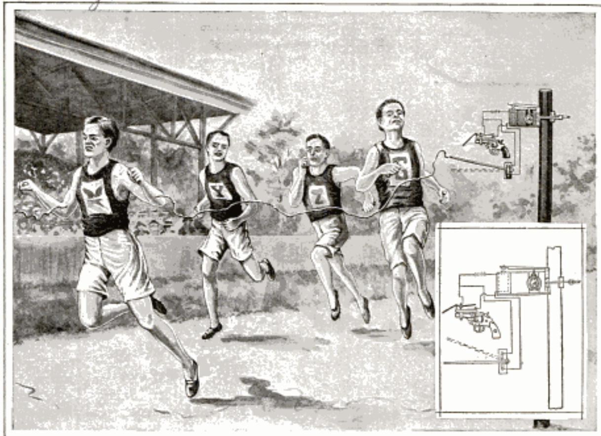
Either Firing a Revolver or the Impact of a Racer will Operate This Automatic Timer
