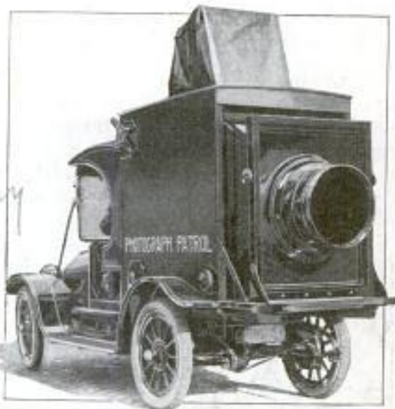
The Camerallike Body of This Car Is a Fully Equipped Dark Room, Which Frequently Saves Newspaper Photographers Valuable Time by Enabling Them to Develop and Print Exposures While Returning to the Office. The Roof Serves as a Platform from Which to Take Photographs
