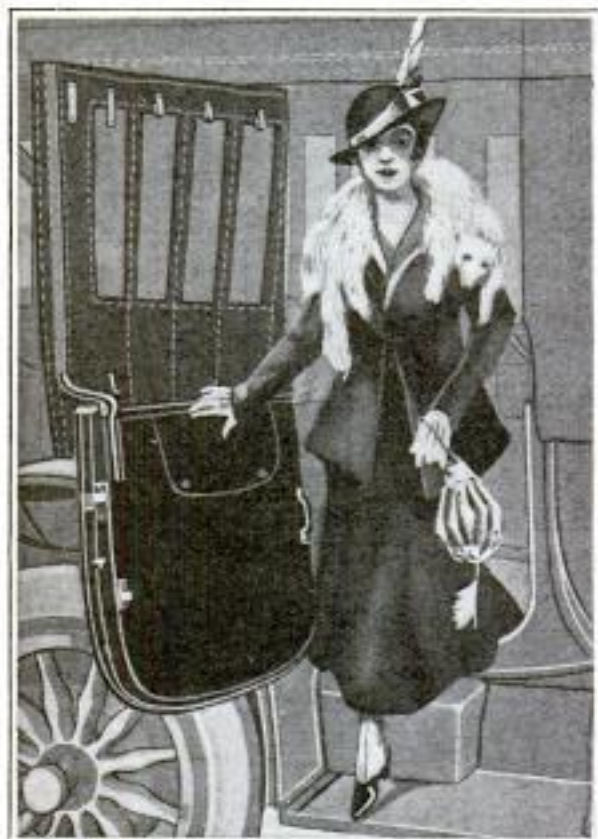
New Storm Curtain for Automobile Use is Fastened on Brackets to the Door, Allowing Easy Entrance and Exit
