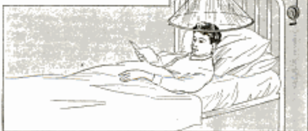
Ice Packed in the Hollow Walls of the Cylinder Cools the Atmosphere without Creating a Draft
