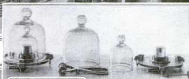
The Two Standard Kilogram Weights: The One under the Glass Domes is Used Only to Check the Accuracy of Working Standard beside It
