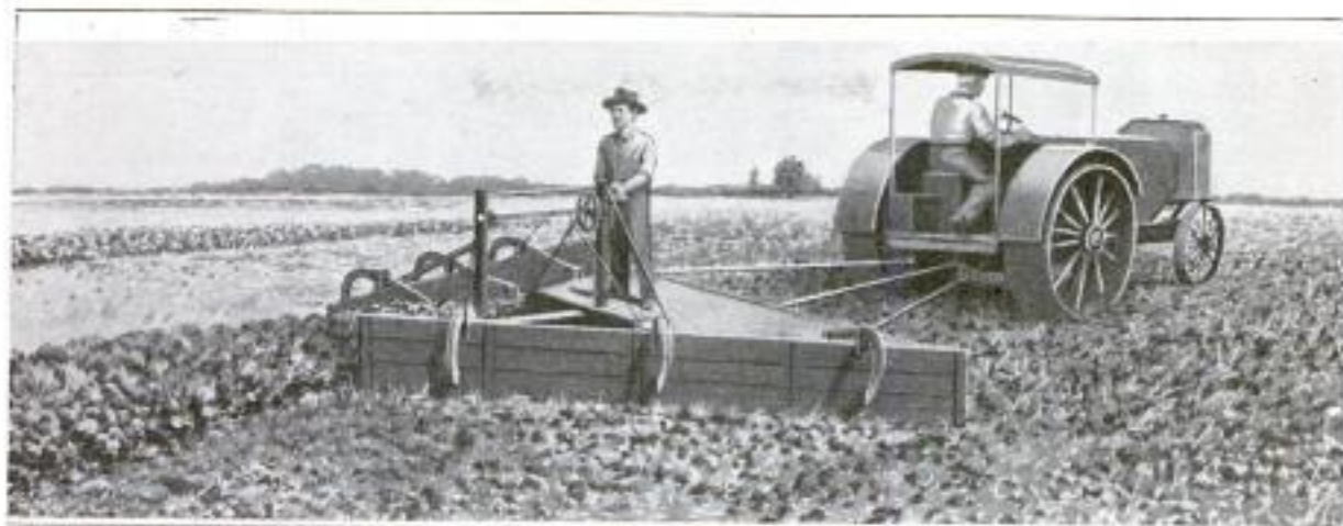
Close View of the Grader, Showing Its Construction. The Machine Throws Up a Two-Foot Levee at One Operation While Traveling Two Miles an Hour
