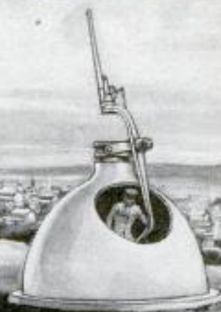
Below Construction and Operation of Aerial Defense Battery is Illustrated. The Pointer and Sights Are in Alinement, and by Moving the Former in Unison with Reversed Image Appearing on Glass, Gun is Made to Follow Target
