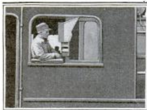
With This New Shield in Place an Engineer can Watch the Rails without Facing a Sleet or Cinder-Laden Wind. The Diagram Shows the Principle of the Device and the Manner in Which It is Constructed
