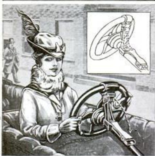
With the Lock Engaged a Car can Only be Driven or Towed in a Circle
