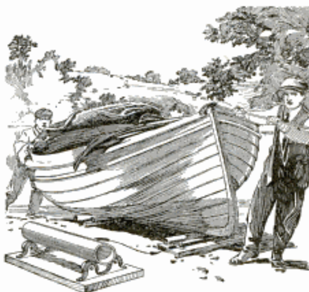
Inverted Truck Casters Placed on a Plank in Position to Hold a Length of Pipe
