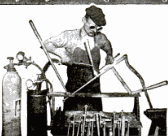
Welding frame of automobile top by oxy-acetylene process. Done quickly, and secures neat finish and quality of joint impossible by any other process.
