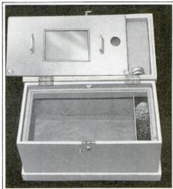
Cats, Dogs, or Other Small Animals can be Killed Humanely in This Chest, Which Has Separate Compartment for the Anesthetic
