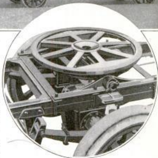
By Means of This "Fifth Wheel," Which Has Several Distinctive Features, a Two-Wheel Trailer can be Easily Attached to or Detached from a Motor Truck
