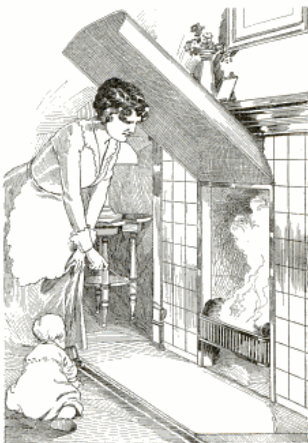
A Hinged Fire Screen That cannot be Forgotten and the Fire Left Unprotected
