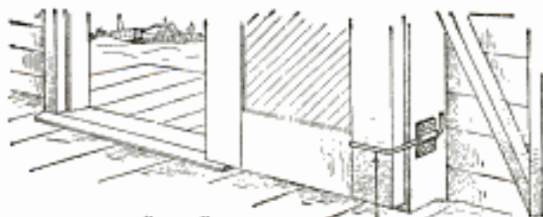
Holder Made of a Rod to Keep a Large Door Open against a Strong Wind
