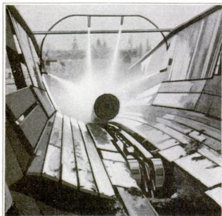
Logs are Given a Shower Bath to Dislodge Stones That might be Imbedded in the Bark and Hence might Shatter the Saw When It Strikes Them
