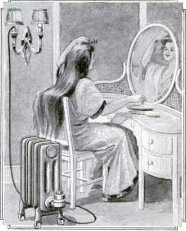
These Electric Radiators are Filled with a Commercial Fluid in Which is Submerged an Open Resistance Coil. Current is Secured from an Ordinary Light Socket
