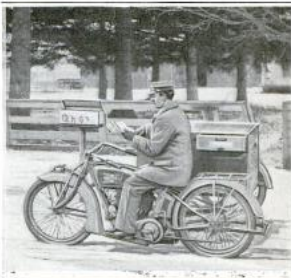
The Sidecar of This Motorcycle Has Several Compartments and is Designed Especially for Rural-Mail Carriers
