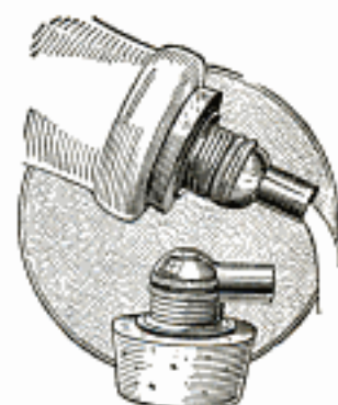
Air-Tight Stopper Designed for Milk Bottles
