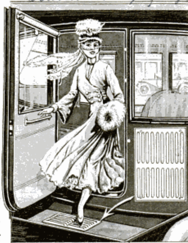
Besides Cleaning the Soles of the Shoes, the Mat Provides an Excellent Foothold Which Lessens the Danger of a Person Slipping When Stepping on the Runboard
