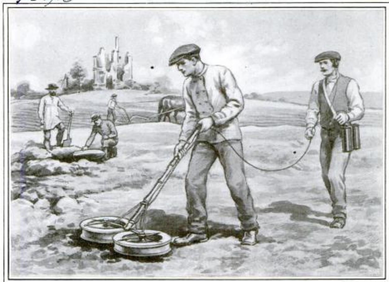
This Instrument Detects the Presence of Shells or Other Metal Buried in the Soil, Thereby Enabling the Farmer to Remove Them before Tilling a Field
