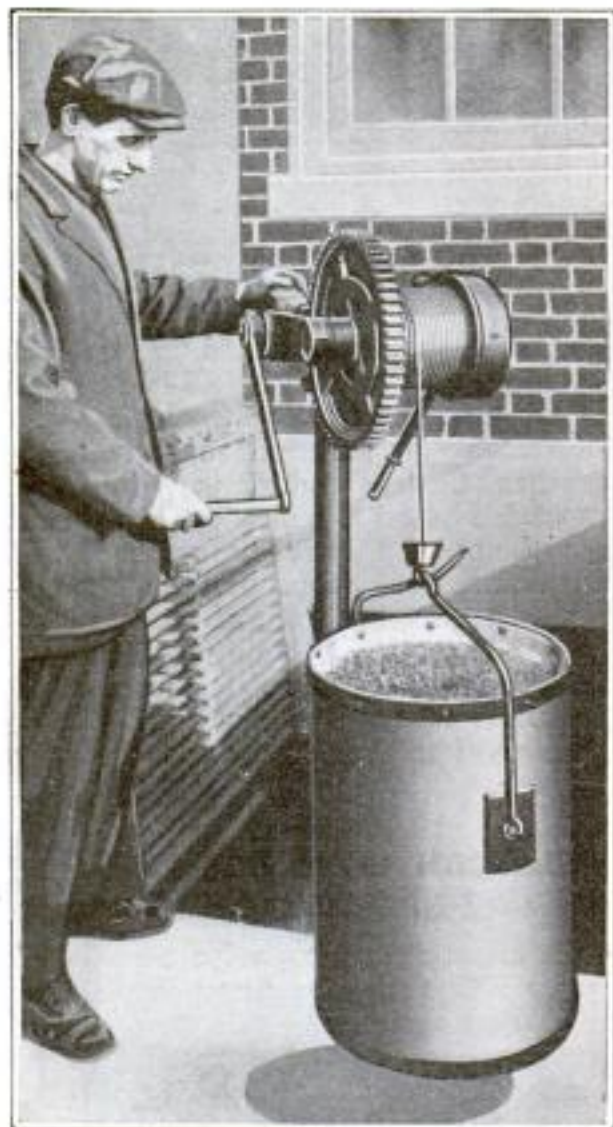
Hand-Operated Elevator Lifts Objects from Basement
