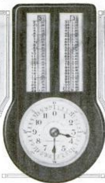
Dial and Price-Computing Scales on the Top Surface of the Machine: The Rollers Automatically Adjust Themselves to Receive Goods of Different Thicknesses
