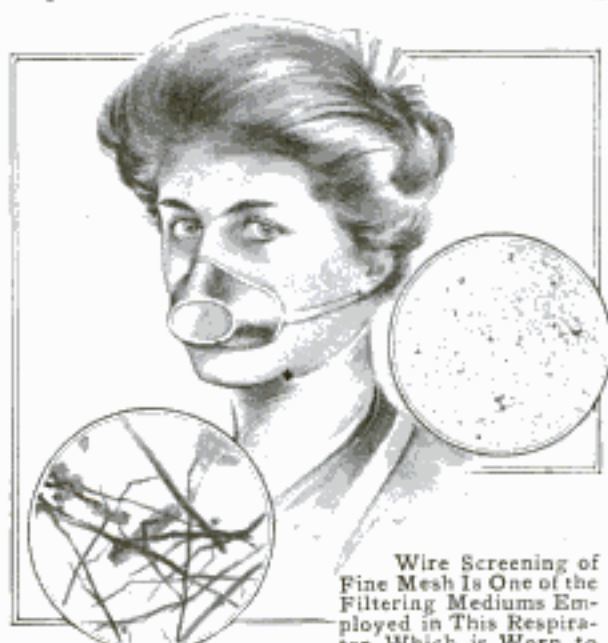
Wire Screening of Fine Mesh Is One of the Filtering Mediums Employed in This Respirator, Which is Worn to Safeguard against the Inhalation of Dust in Factories, the Character of Some of Which is Shown, Highly Magnified, in the Two Inserts
