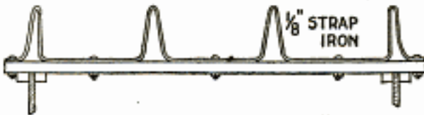
The Racks Form Three Divisions in Which to Lay the Pipe to Prevent Rolling
