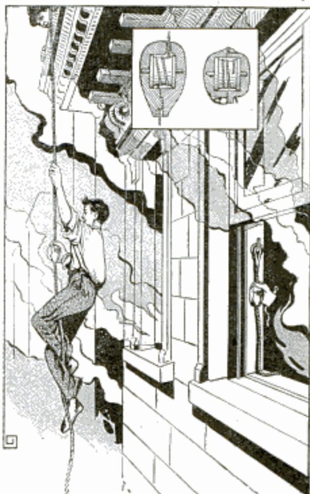
User of New Fire Escape Holds to Pulley in Sliding to Ground
