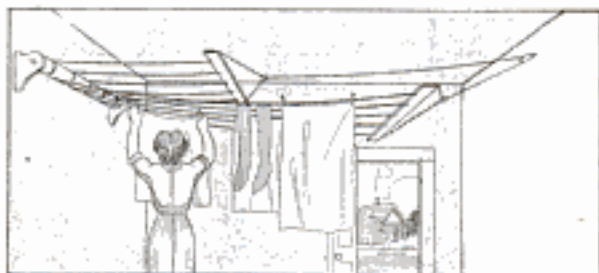
This Clothes Drier Consists of Five Lines That are Spaced Apart by Wooden End Pieces
