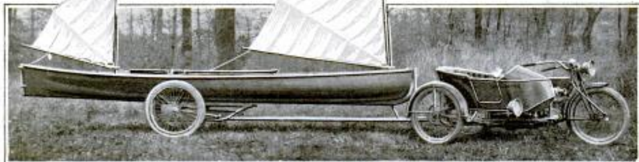
By Providing Permanent Posts to Which They may be Leashed, the Masts may be Taken Down Quickly for Portages, as is Shown in the Photograph at the Left. Below, the Sails are Raised to Show the Manner in Which the Masts are Held by the Uprights
