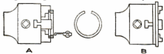
A Ring Placed Back of a Disk being Worked in a Chuck to Keep the Surface True
