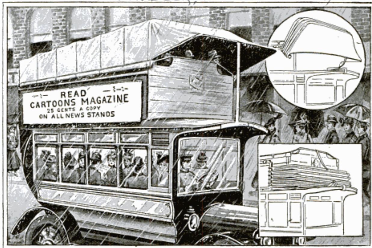
Collapsible Canvas Hood is Arranged to Cover a Vehicle in Time of Storm or Hot Weather
