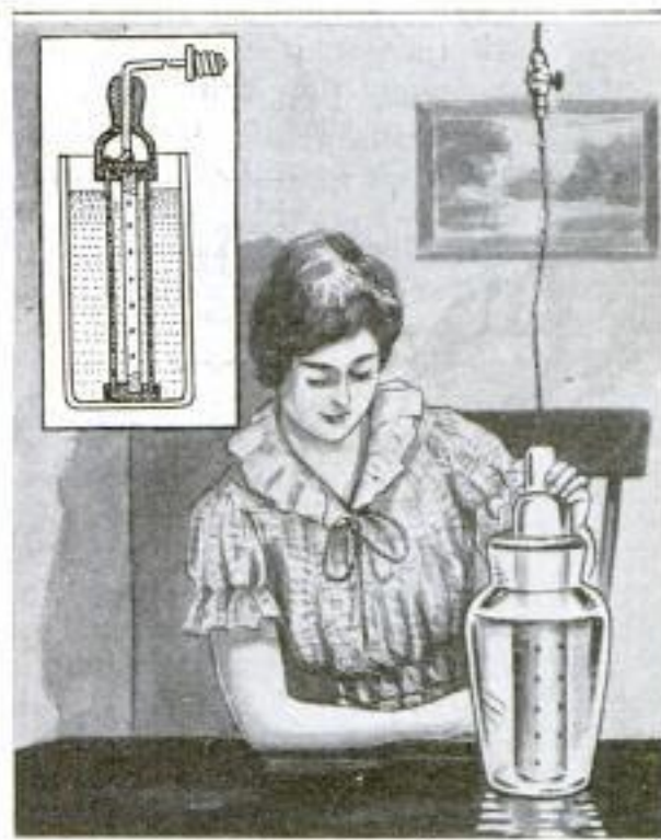
Apparatus Which Utilizes Electrolytic Action in Purification of Water
