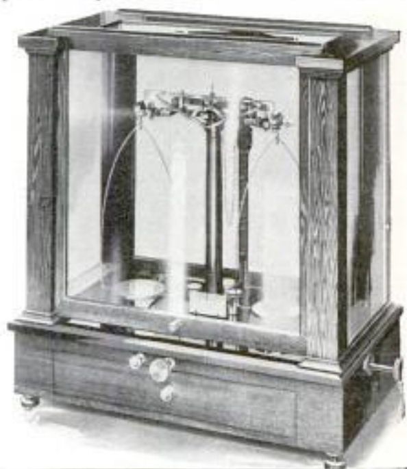
Analytical Balance Uses Chain Instead of Scale Weights
