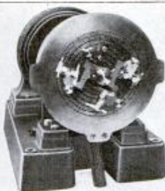
The Above Instrument, a Distributor, Makes the Multiplex Operation Possible. It Is by Using an Apparatus of This Kind at Each End of a Line that the Signals Rendered by Different Transmitters are Directed to the Proper Receivers. At the Right Is a Perforator
