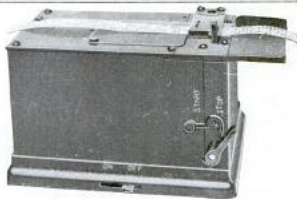
Extending from the Perforating Machine, Shown at the Right of the Instruments Grouped Above, Is a Transmitting Tape Which is being Fed into a Sender. Next to the Letter Is a Receiver Which Prints the Messages Ready for Delivery in the Form Shown at Left
