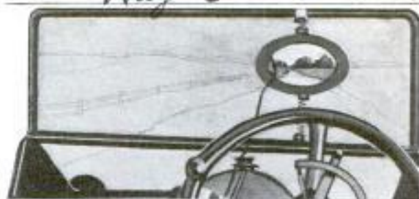
Heat from the Coil Clamped on the Windshield Keeps Glass from Freezing Over in Winter
