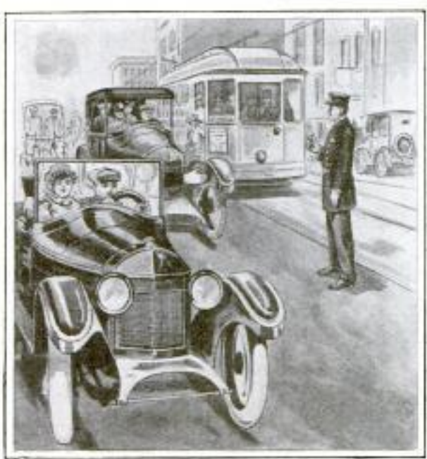
The Indicator Hand is Operated by Pulling a Cord Extended to the Steering Wheel
