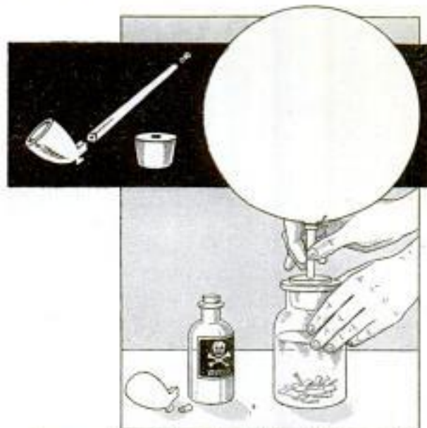
Apparatus for Filling Toy Rubber Balloons with Hydrogen Gas to Make Them Fly to a Great Height
