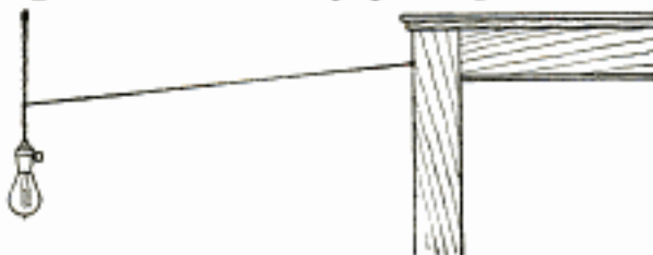
The Cord Fastened to the Door Casing is Easily Located and Followed to the Lamp
