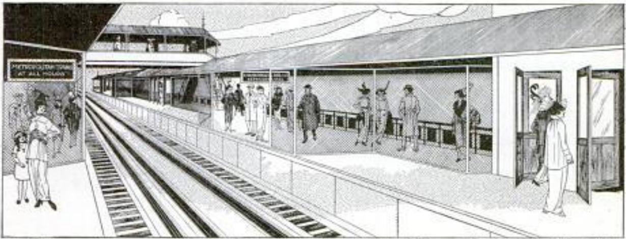
How Platform of Elevated Road may be Easily Adapted to the Use of Proposed Pay-as-You-Enter Trains
