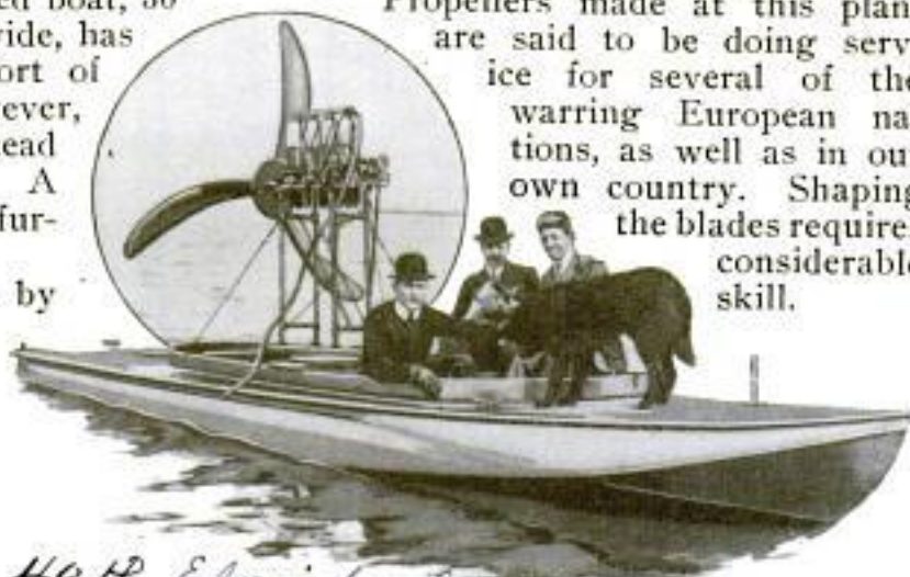
"Water Skimmer" is Used as Tester for Aeroplane Propellers
