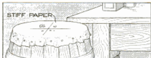
The Paper Stretched over the Barrel Top was Cut after Feeding the Rats on It for Some Time
