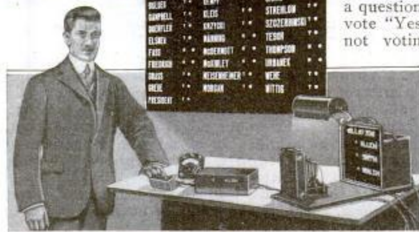
Model of Voting Device to be Considered by Congress: Shows the Inventor, Desk Push Button, Speaker's Meter, Indicator Board, and Photographic Paraphernalia
