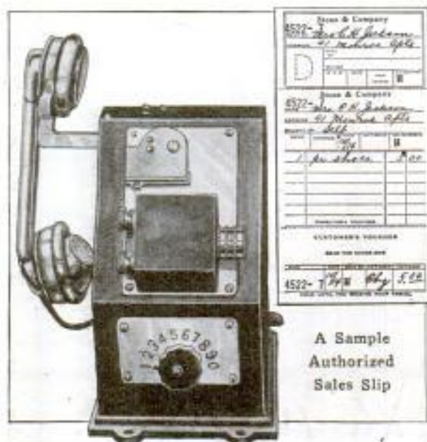
Stamping Machine and the Telephone a Clerk Uses to Call Up Credit Department: The Lower Dial on the Machine Selects the Particular Operator Desired
