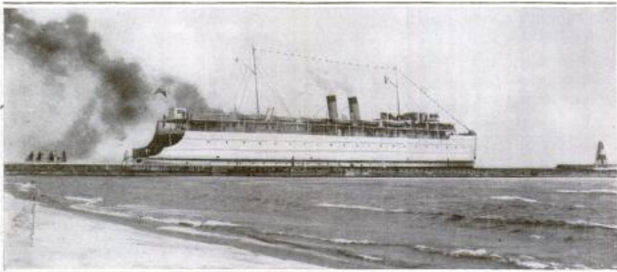
This Car Ferry, the Largest on the Great Lakes, Is Capable of Carrying 30 Railroad Cars and 1,000 Passengers
