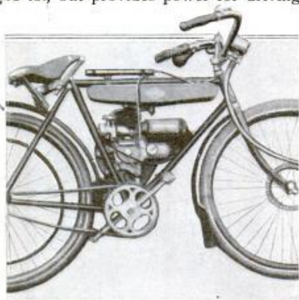
This Motor can be Fitted to Any Diamond-Shaped Bicycle Frame; Power is Transmitted through a Hoop-Shaped Belt Pulley Attached to the Spokes of the Rear Wheel
