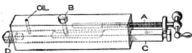
Screw-Feed Chamfering Tool to Fit in the Tool Post of a Lathe, Planer, or Shaper
