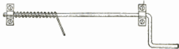
A Copper Wire Wrapped around and Soldered to a Straight Rod for a Lead Screw
