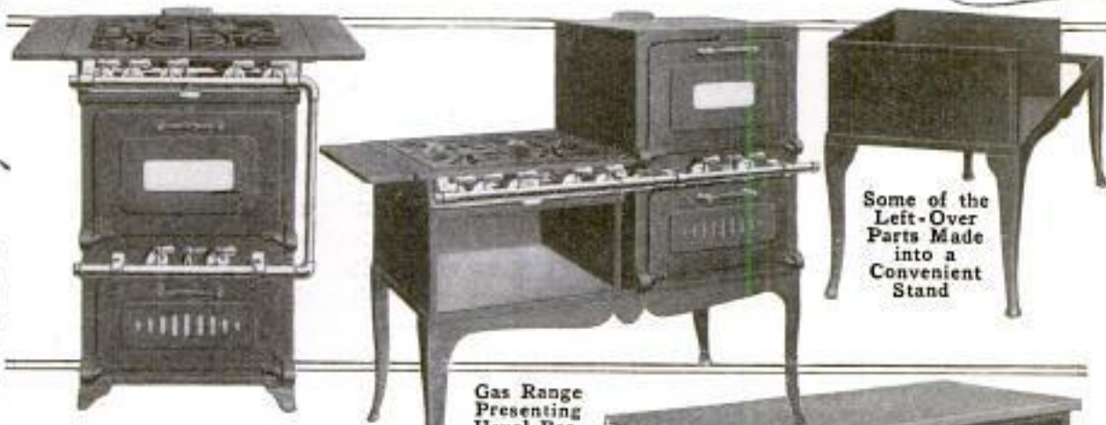
Same Oven Units, Cooking Top, Burners, and Extension Shelves Made into a Double Oven
