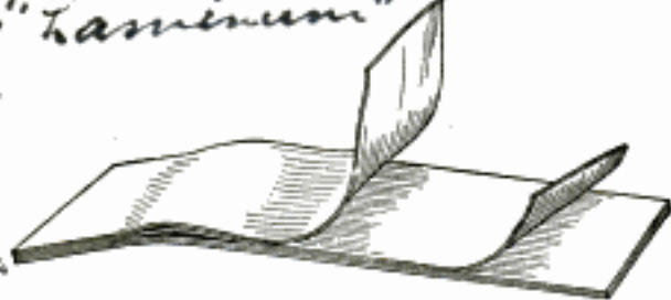
Shim Block Made of Thin Strips of Metal Held Together by a Metallic Binder
