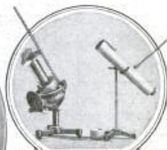
Two Instruments for Measuring Direct Heating Effect of Sun's Rays
