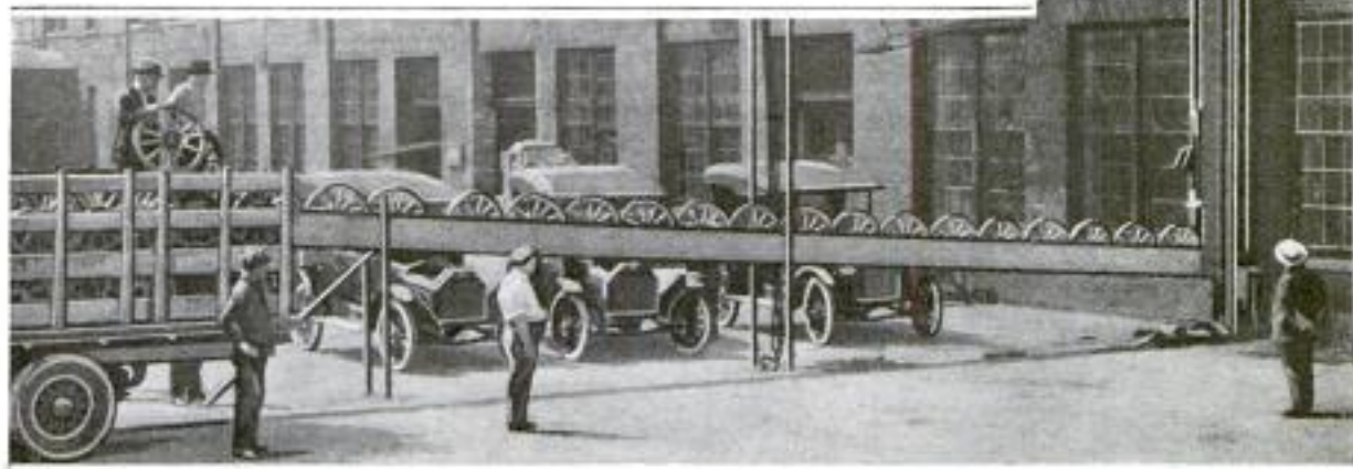
Auto Wheels Roll into This Plant: The Elevator on the Right Lifts Them to the Top of the Building Where They Roll on Farther to Their Respective Autos
