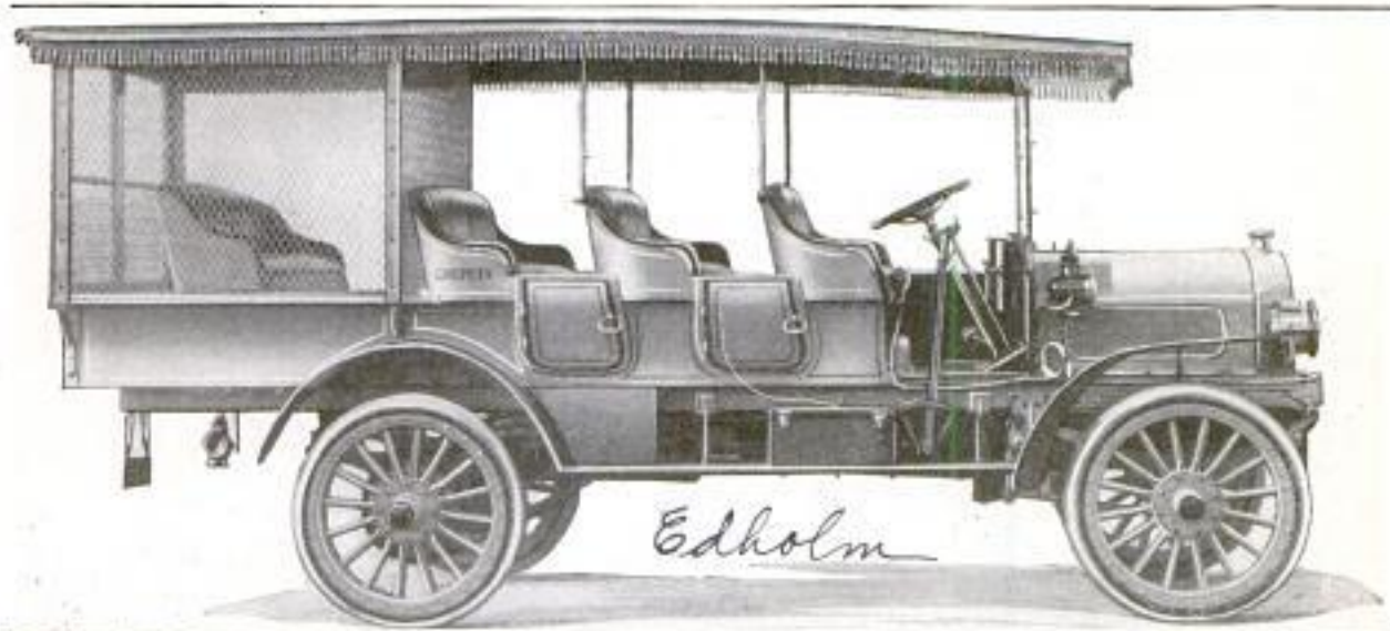
Motor Stage in Service in Colorado: As a Protection against Robbery, the Mail, Express, and Other Valuables are Carried in the Wire-Mesh Cage at the Rear
