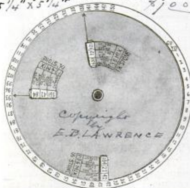
In Using This Scale for Computing Concrete, the Slot Corresponding to the Required Mixture is Set Opposite the Quantity of Concrete to be Mixed, and the Proportions of the Ingredients are Read through the Slot
