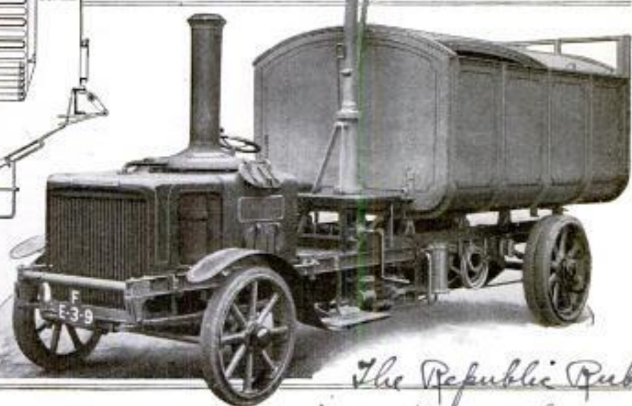
Two Views of Self-Dumping Steam Truck. Recently Brought Out in England, Which Uses Coke as Fuel
