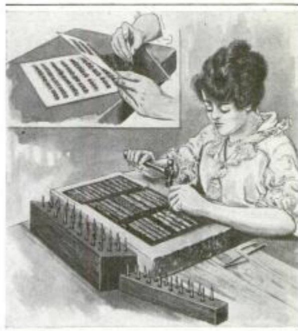
Making "Punched Plate" Negatives from Which Music is Printed
