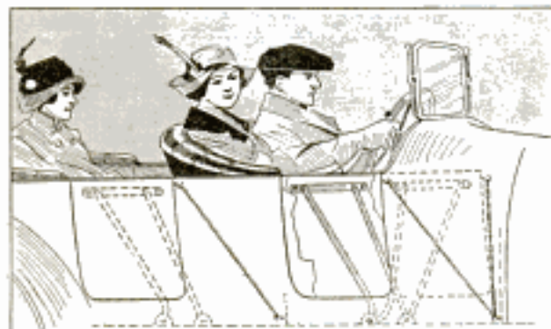
This Motor-Car Door Disappears When Opened
