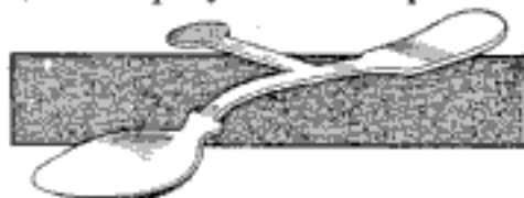
The Projection Keeps the Spoon from Entering the Mouth When Taken in the Left Hand
