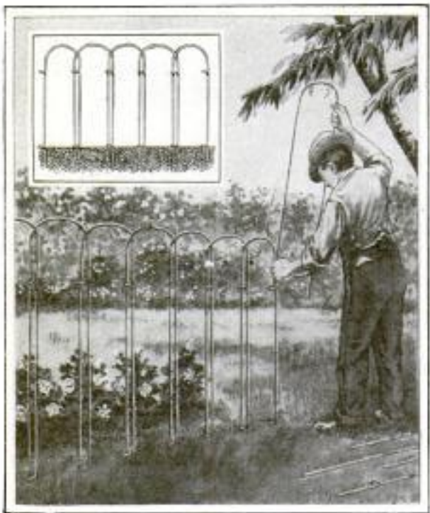
Fence Made Up of U-Shaped Wire Sections, Designed for Quick and Easy Erection
