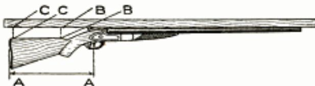
The Measurements are Taken of the Drop at the Comb and Heel, and of the Stock from the Butt to the Forward Trigger
