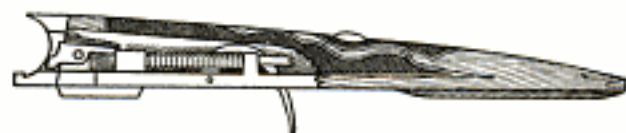
The Shells are Started About One-Quarter Inch in the Regular Way Before the Ejector Kicks Them Out
