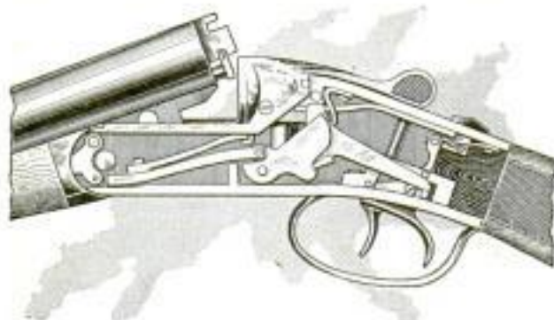
A Hammerless Gun with Roller Bearings to Overcome the Short Leverage and Make It Open and Close Easily
