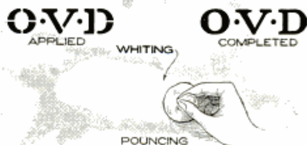
The Stencil as It is Cut; after Applying; Completed Letters; Sized and Pounced
