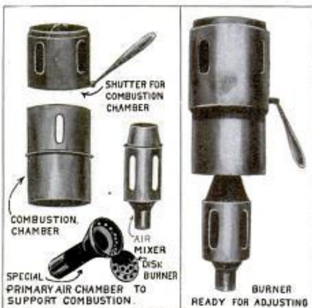
The Various Parts of the Device are Shown and Identified at the Left, While at the Right Is the Burner Assembled
