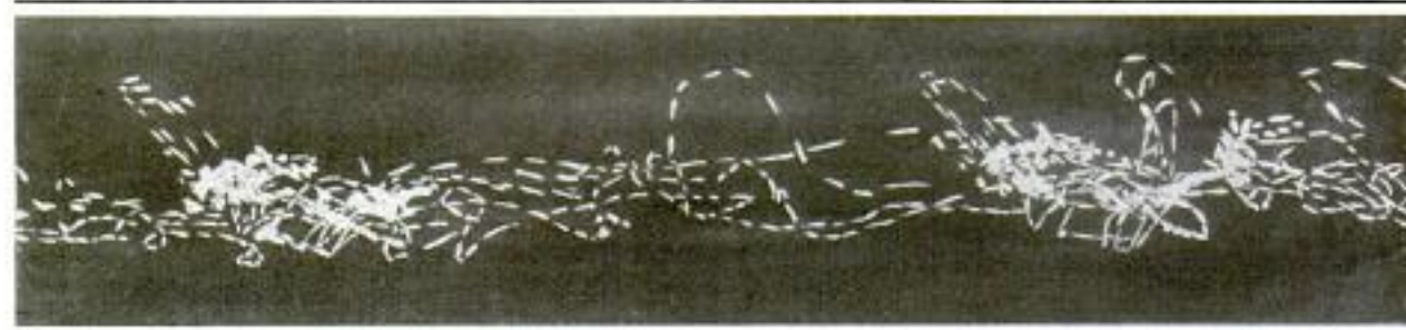
Record Made by the Cyclegraph: The Tangled String of Dashes Shows the Trail of the Workman's Hand as He Manipulates the Machine
