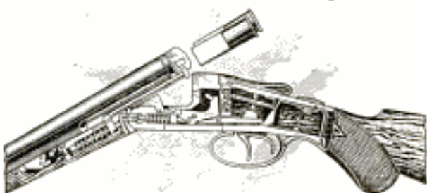
The Cocking Hook Is an Ingenious Device, with Variations Used on Different Makes of Arms
