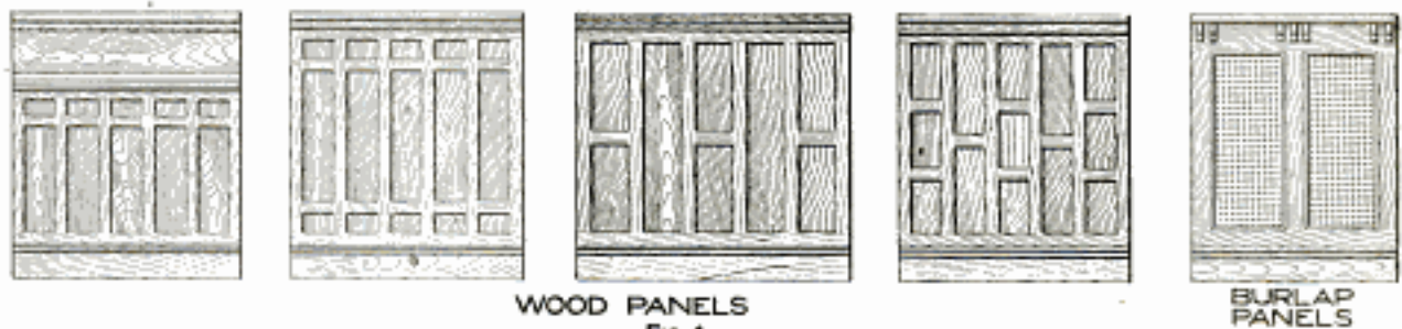
Designs for Wood and Burlap Panels: Where Wood is Used for the Panel It must be Made of Three-Ply Veneer to Prevent Warping by the Changes in Weather
