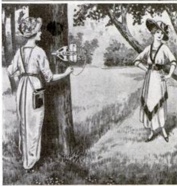
By Pressing a Small Lever the Prongs Fasten Themselves into Any Wooden Object
