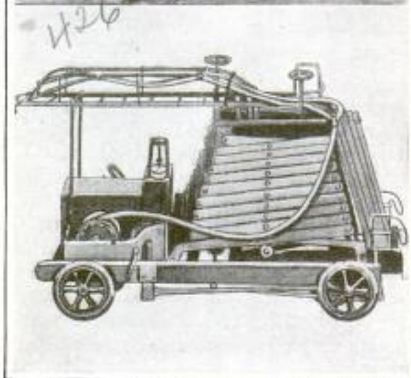
The Tower may be Elevated to a Height of 100 Feet in One Minute's Time. Its Appearance When Collapsed is Shown Below
