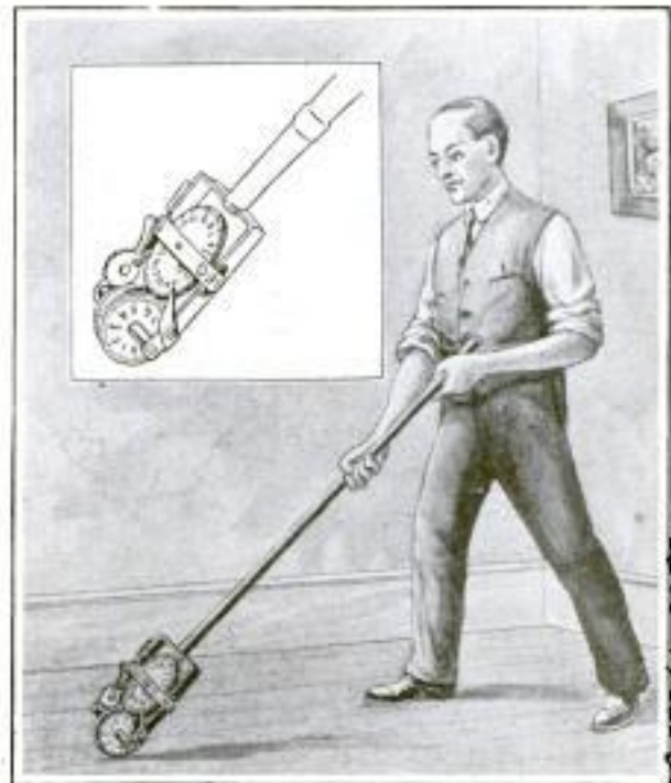
The Device is Especially Useful for Measuring Curved or Irregular Outlines, but may Also be Employed on Straight Lines as Shown Here
