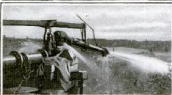
Using Hydraulic Giant for Stripping the Earth from Mineral Deposits at a Mine in Canada: This Machine Throws a Five-Inch Jet under a Pressure of 200 Pounds to the Square Inch
