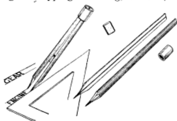
Two Pencils Joined Together with Ferrule on Upper Ends, and Sliding Wedge to Draw Parallel Lines
