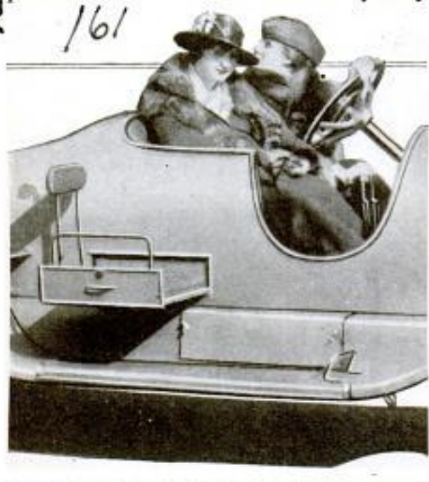
The Drawer Seats at the Sides are Pushed Out of View When Not in Use
