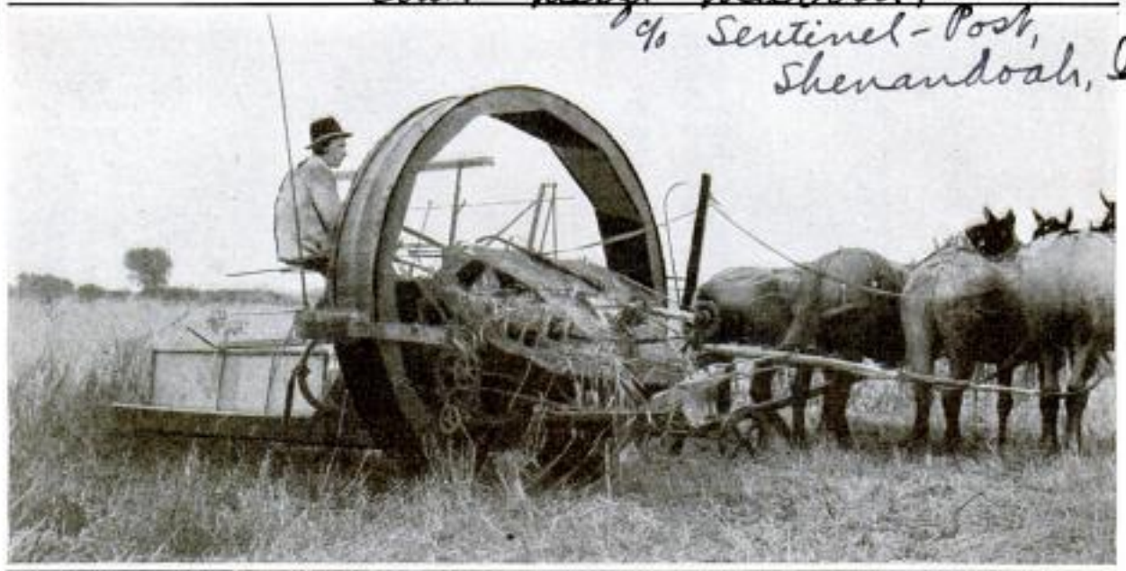
The Large Hoop Forms a Track for the Bull Wheel and Prevents the Binder from Sinking into the Soft Ground
