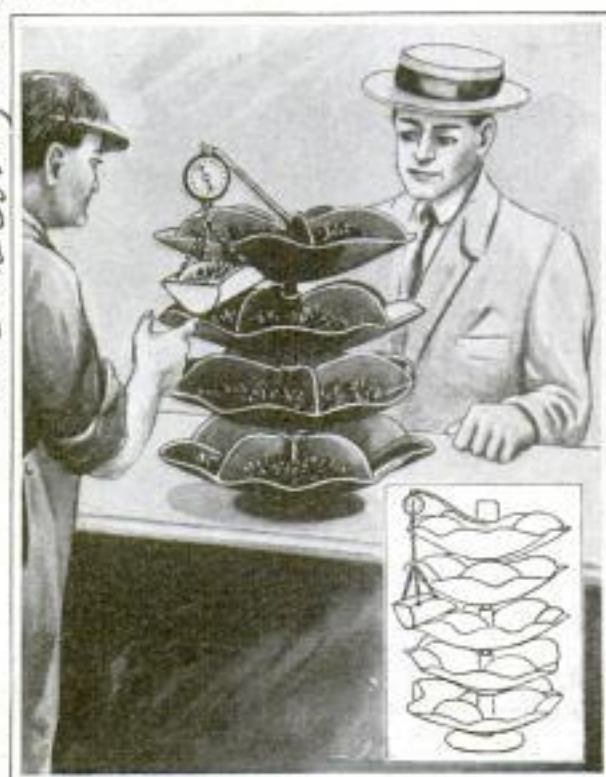
The Bin Is Particularly Convenient because Its Capacity Allows It to Hold a Large Assortment of Nails and Bolts
