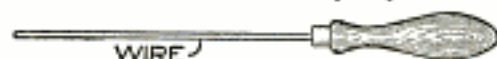
The Tool will Pick Up a Drop of Oil and Deposit It Where Wanted
