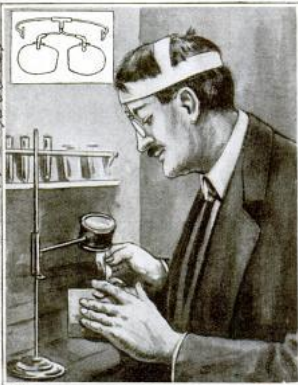
The Glasses are Suspended before the Eyes from a Bandagelike Headgear
