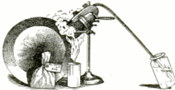
Separating the Gold and Mercury by Heating the Amalgam in an Iron Retort
