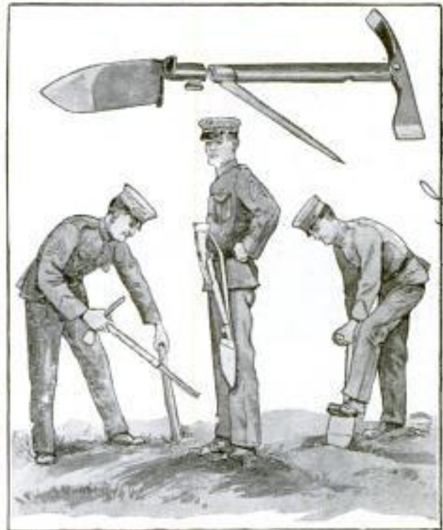
The Intrenching Tool and Several of the Ways in Which It may be Used
