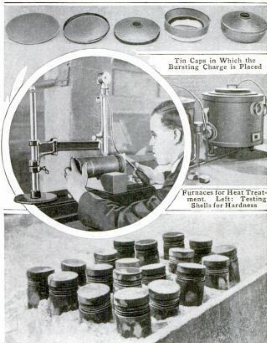
As Soon as the Nose of the Shrapnel Shell has been Pressed into Shape It is Treated by a Bath in Quicklime
