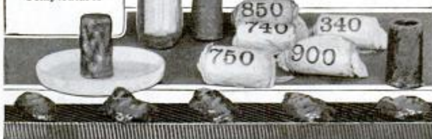
Different Forms in Which the Metallic Salts are Used in Determining High Temperatures
