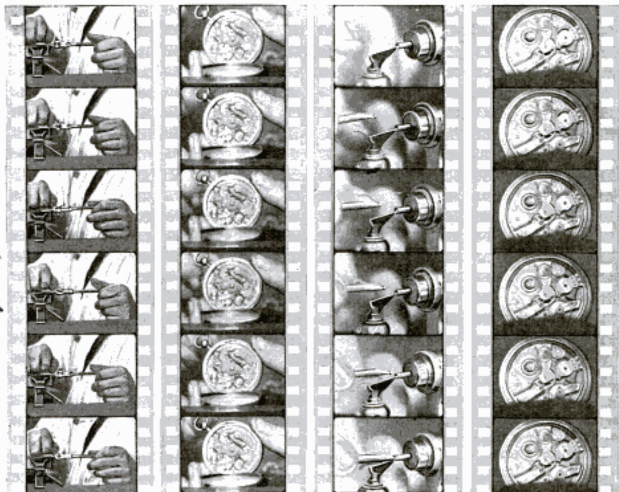
From Left to Right These Films Show: A Delicate Job of Filing; Mechanism beneath Dial of Repeater of "Gooseneck" Type; Mounting a Jewel; Bell and Hammer Mechanism of a Repeater or Striking Watch
