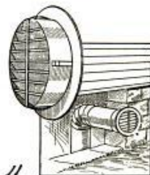
11 Air Strainer for Furnace Duct
