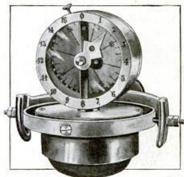
Vertical Compass of French Invention Designed for Use of Aerial Navigators
