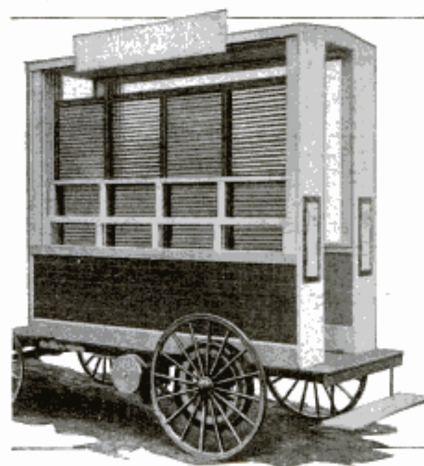
With This Device for Displaying Equipment for Sleeping Porches, the Sash Move Up and Down Automatically As the Wagon Moves Forward
