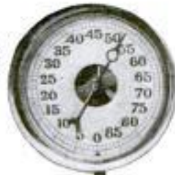
With This Device the Train is Made to Run Constantly at the Speed for Which the Pointer on the Dial is Set
