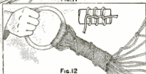
Fig. 11 The Gauge Board is Again Used for the Long Loops at the Finishing End, Then the Cords are Wound
