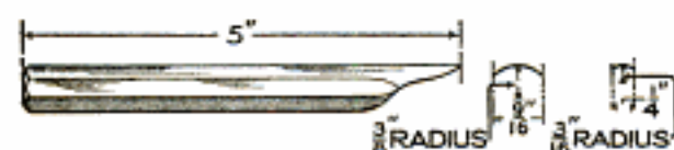
The Curved Edge of the Chisels Makes It Easy to Cut a Curved Opening
