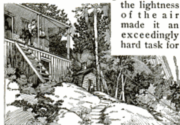
A Cableway Run from a Mountain Lodge to a Stream Below on Which a Trolley is Operated with a Windlass, to Obtain Water
