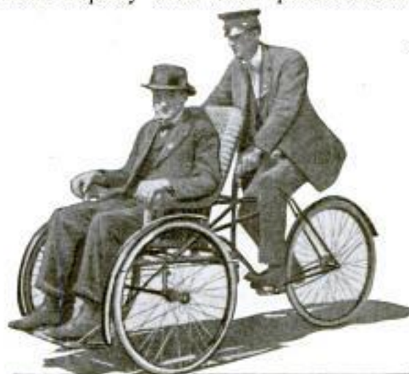
PHOTO BY ROCKWELL FEATURE SERVICE Combination Wheel Chair and Bicycle Which is being Used in Carrying Patrons about the Exposition Grounds at San Francisco
