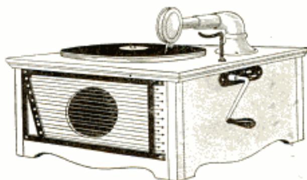
The Harp Strings Vibrate in Sympathy with the Tones Sounded by the Phonograph
