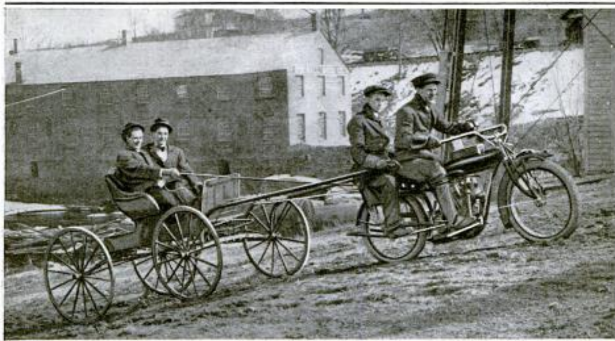
Twin-Cylinder Motorcycle Pulling an 1,188-Pound Load up a 24-Per-Cent Grade
