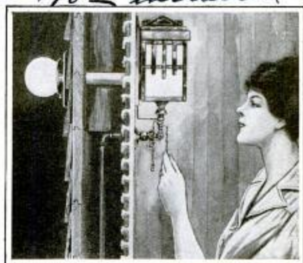
Some of the Horizontal Rays from This Lamp Pass through the Tube to the Globe Outside, Illuminating the Porch as Well as the Hall
