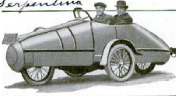
Odd-Appearing Car Which can be Turned Completely Around in Its Own Length
