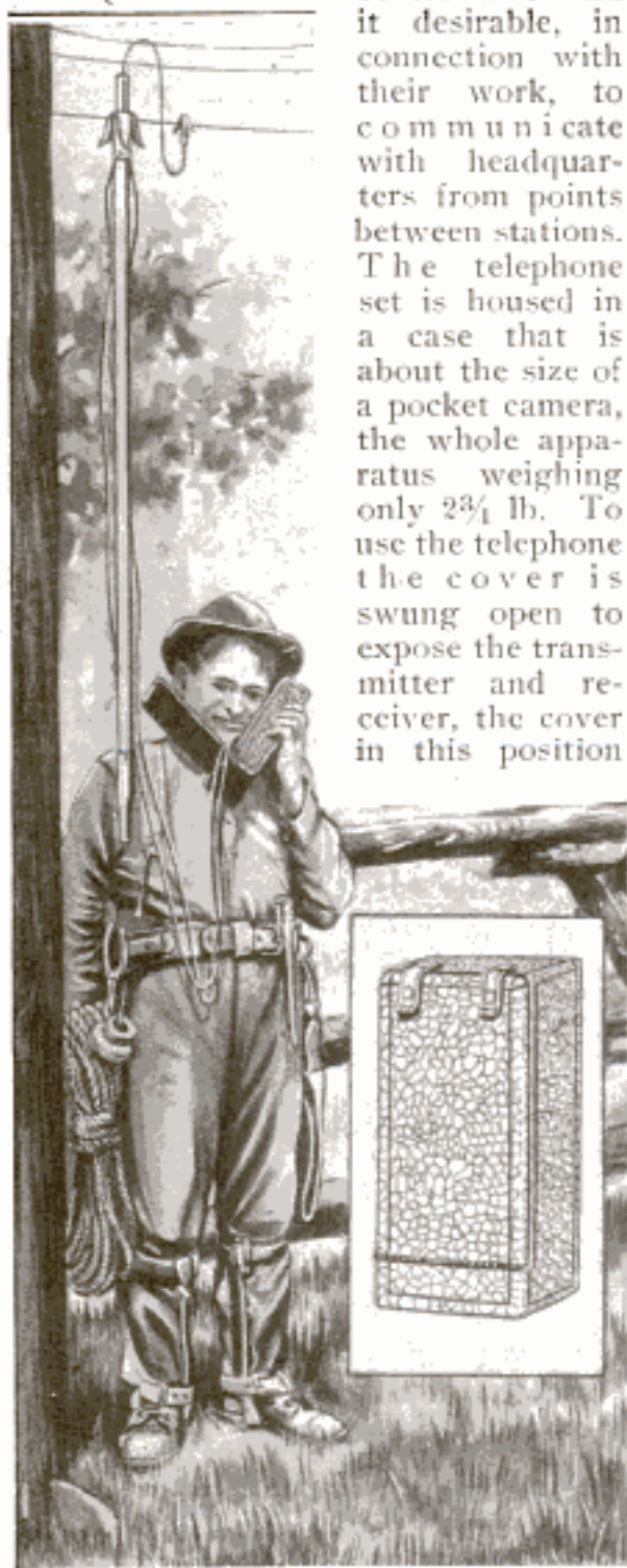
Talking with Headquarters by Means of the Pocket Telephone: This Instrument is Easily Connected with the Telephone Line, and, When Closed, Is About the Size and Shape of a Pocket Camera
