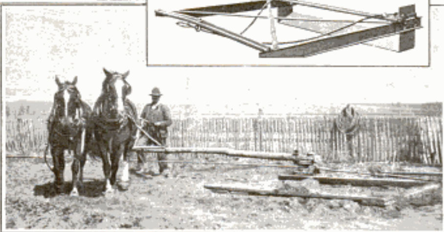
Apparatus Installed in Forest-Service Nursery for Loosening Seedling Trees for Field Planting
