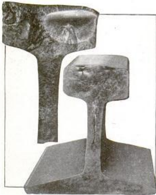
Rails That Broke as the Result of Transverse Fissures: The Nucleus from Which the Fault Spread in All Directions can be Seen in Each of the Rails
