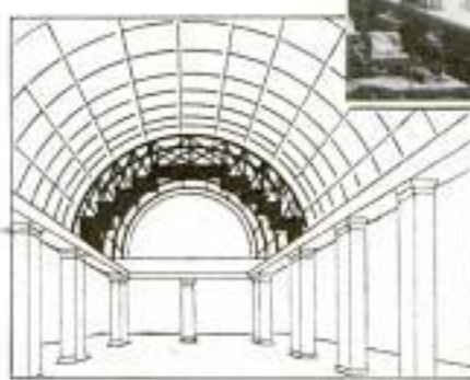
The Picture at the Top Shows the Traveling Crane with Electric Lift, Used in Cleaning Windows; Arched Crane for Cleaning Skylight Shown at Left
