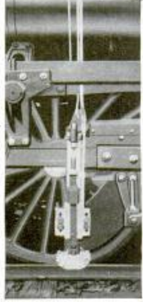
How the Ramp and Contact Shoe are Arranged in a New Automatic Train Stop
