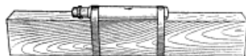
A Bottle Filled with Water and Tied to a Straight Piece of Wood for a Level
