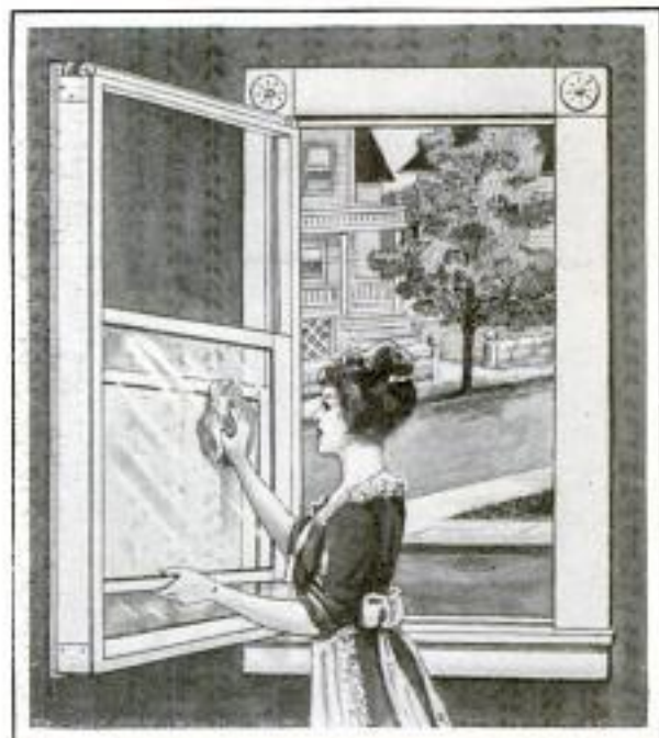
By Means of the Double, Hinged Frame This Window can be Swung Either Inward or Outward
