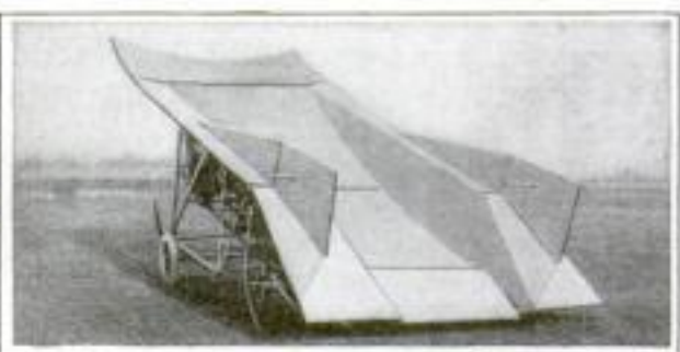
The "Uniplane" Shown Above Has an Elevator at the Rear and Rudders on Top
