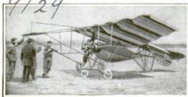
This Monoplane Has Wings with Channeled Under Surfaces and is Made of Aluminum and Steel
