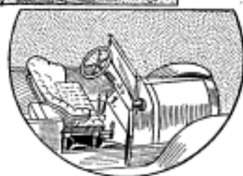
This Automobile Seat Is Adjustable to Suit the Driver
