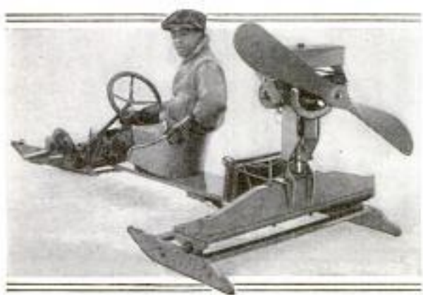
Homemade Ice Boat Driven by a Three-Horsepower Motor
