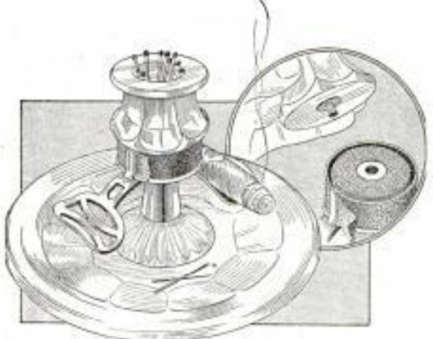
How the Continuous Roll for Striking Safety Matches is Inserted in a Match Holder
