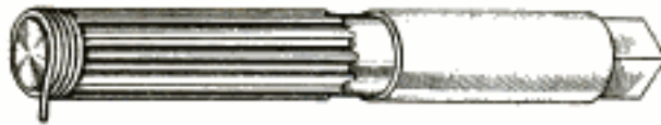
The Cutters are Ground Down and Then Wrapped with Fine Wire and Soldered
