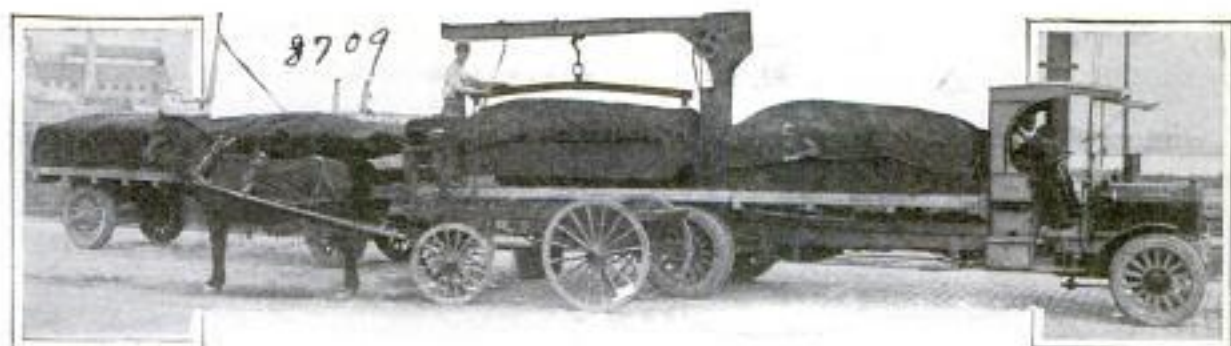
This Garbage Truck is Equipped with a Two and One-Half Ton Crane with Which the Loaded Boxes are Lifted from the Garbage-Collection Wagons to the Deck of the Truck
