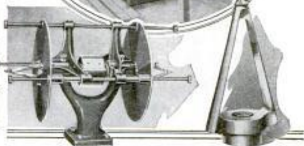
Machine That Distributes Cans to Filling Machines. Small Machine Shown at Bottom Is a Cabbage Corer
