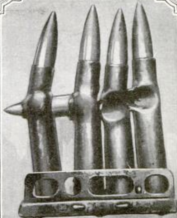
This Shows a Clip of Cartridges, Carried by a British Soldier in His Bandolier, Which was Pierced by a Bullet during an Engagement
