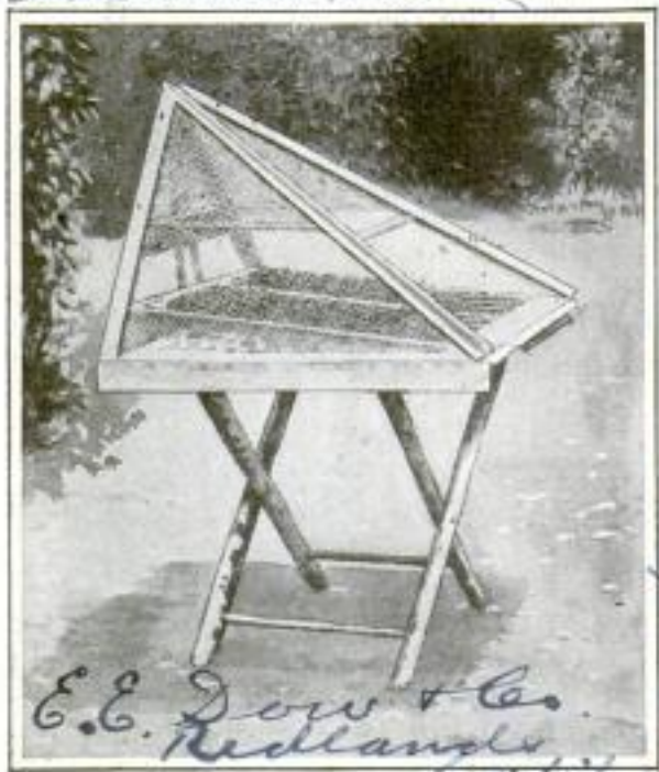
This Cheap but Efficient Fruit Drier Exposes the Fruit to the Sun on Three Sides
