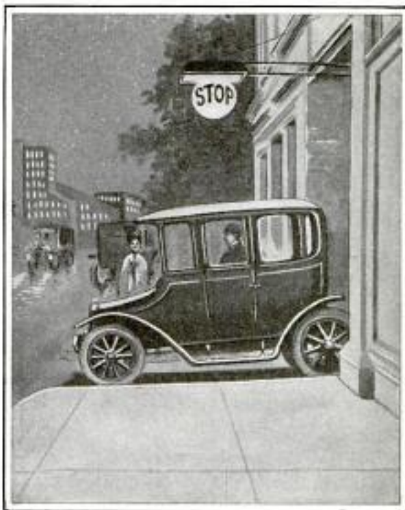
Red Lamp with Automatic Gong Warns Pedestrians When Car is Coming from Garage
