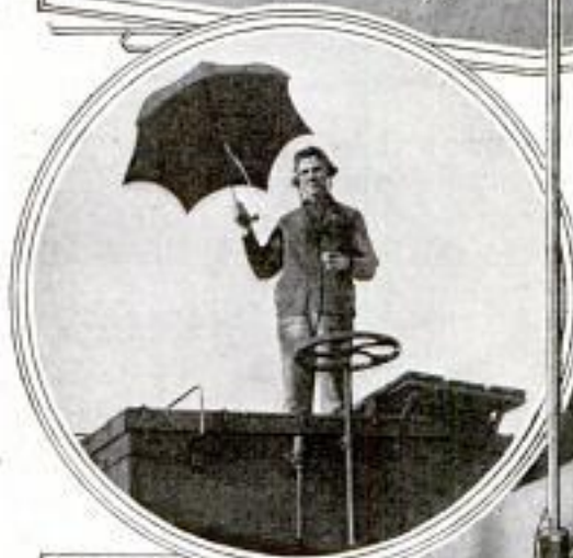
With the Ribs of the Umbrella Acting as Antennae, This Brakeman is Receiving a Wireless Message from a Station Located Several Hundred Feet Away
