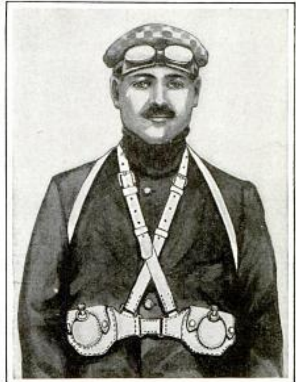
Aeronautic Watches Carried in Cases Which Strap about the Body of a Pilot
