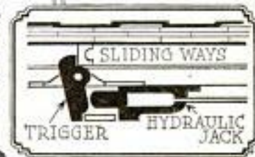
Steel Launching Trigger Held in Place by Hydraulic Jack. When This is Released the Ship Begins to Slide to the Water
