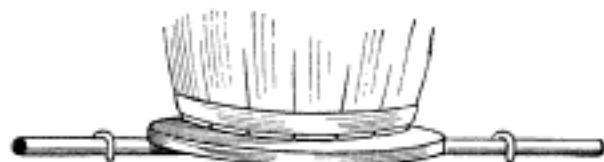
A Tipping Base for Use in Jostling Down Small Parts in Barrels and Boxes for Shipment
