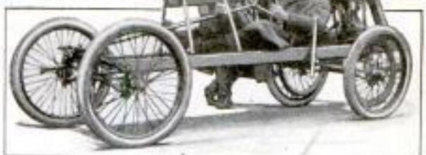
This "Wind Wagon," Made Up of Motorcycle and Cyclecar Parts, is Capable of Making 25 Miles an Hour
