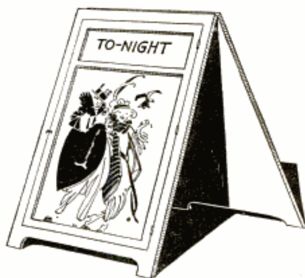
The Outer Surface of the Board Has a Hinged Skeleton Door to Hold the Poster
