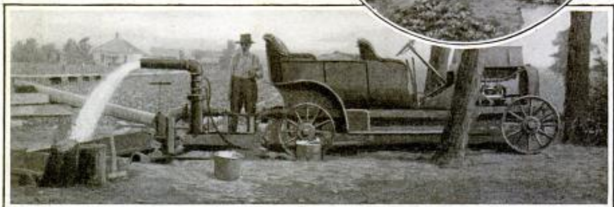
Irrigating a Celery Field by Pumping Water from the Ground with a Motor Car
