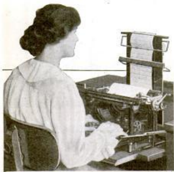
The Notebook is Raised or Lowered One Line at a Time by Means of the Lever at the Right of the Operator
