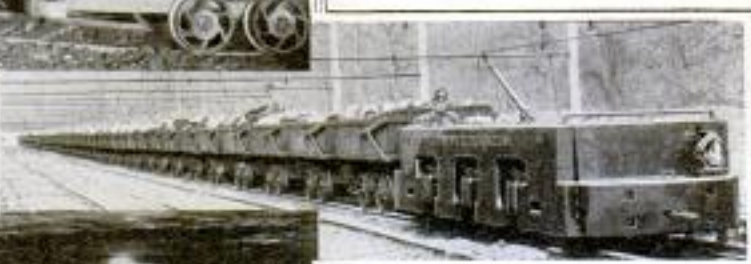
This 25-Ton Electric Locomotive Handles the Entire Output of the Mine against a Grade of 132 Feet to the Mile
