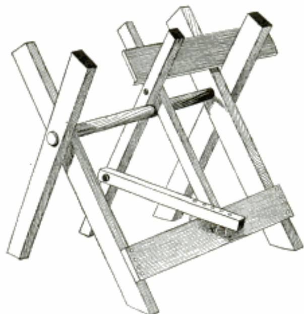
Sawhorse Attachment That Provides a Way of Holding Any Short Length of Wood
