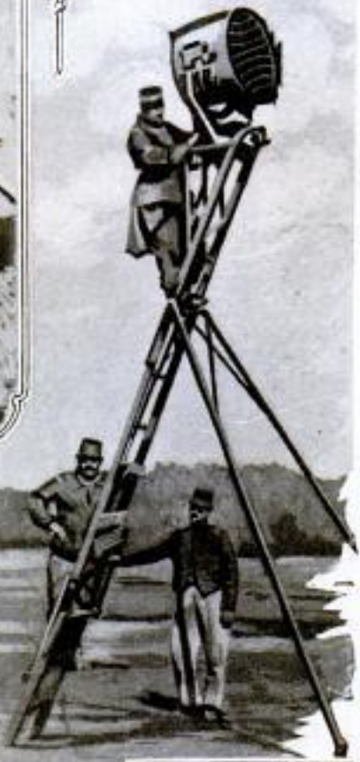
Ladder-Tripod Mounting for Searchlight. The Motor Car Carries an Electric Plant Supplying Current to the Arc
