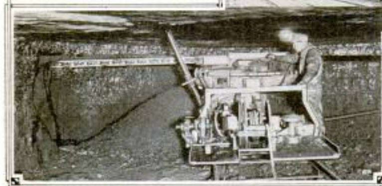
Overcutting Machine in Operation
