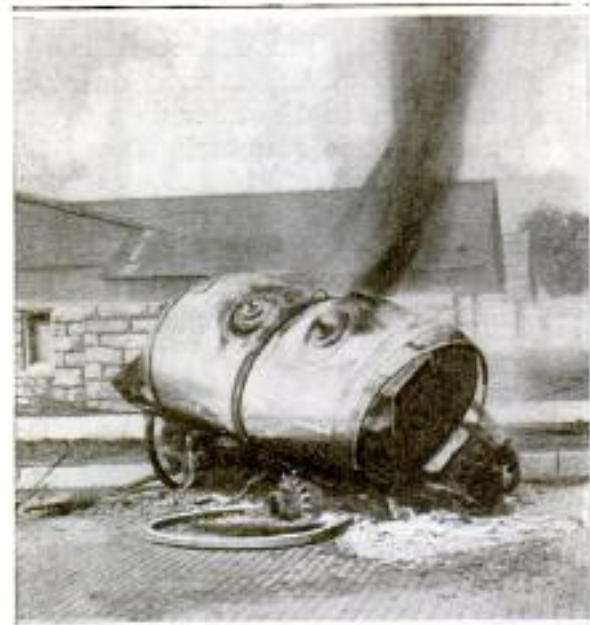
This Oil-Tank Wagon was Set on Fire by a Match Applied to the Gasoline Drippings
