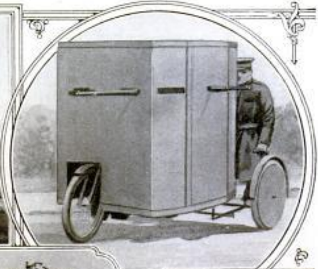
This Armored Motorcycle and Sidecar, One of the New Types of War Vehicles in Use in Europe, Carries Two Riflemen and a Driver, and Travels at High Speed
