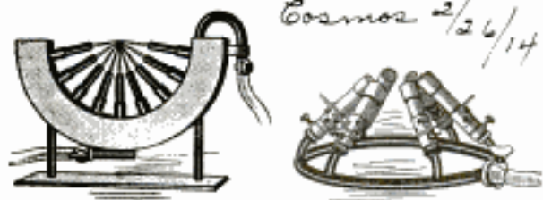
New Form of Bunsen Burner Has Flames Converging
