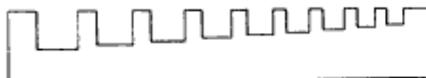
Gauge Made of Sheet Brass Having Slots Corresponding in Length and Width with the Caliper-Layout Measurements
