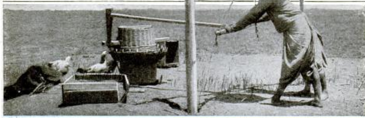
This Machine for Grinding Rice is of a Type That has been in Use by the Natives of Siam for Centuries. The Rice is Ground between Two Roughly Hewn Stones. One being Rotated Back and Forth by the Bamboo Arm Slung from the Wooden Support
