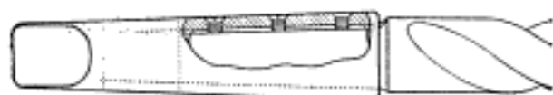
VIEW SHOWING DRILL IN SOCKET A Socket for Holding a Drill That Has Its Shank Twisted or Broken Off
