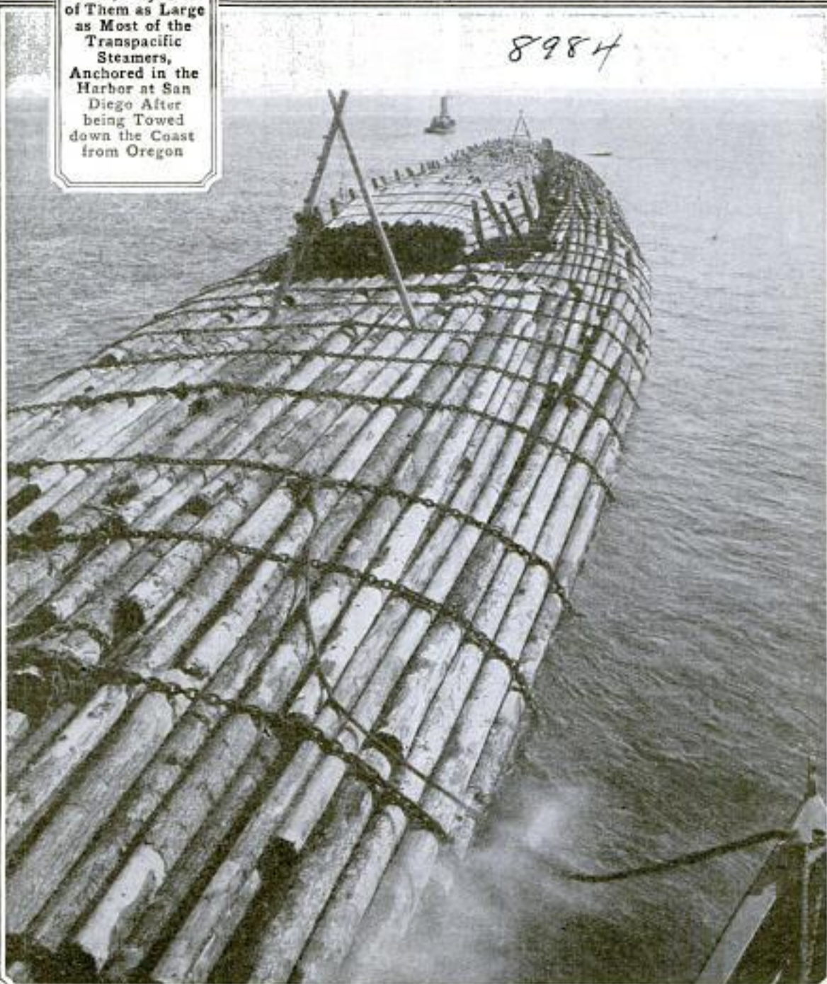
One of the Great Rafts, Bound Together by More Than 100 Tons of Steel Chain, being Drawn into Port. Twenty-Nine Such Barges have been Piloted down the Coast in the Last Few Years
