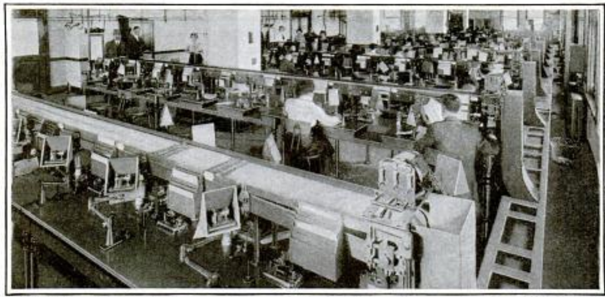
In This Telegraph Office the Messages, as Fast as Received and Typewritten, are Tossed on the Moving Belt and Conveyed to the Distributing Table. From the Latter the Messages are Distributed by Pneumatic Conveyors to the Different Divisions Where They are Handled by Girls on Roller Skates
