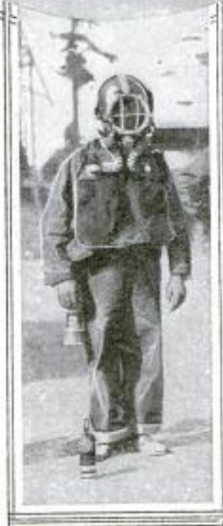
Mine-Rescue Worker Equipped with Oxygen Helmet and Ready for Work, Shown Below
