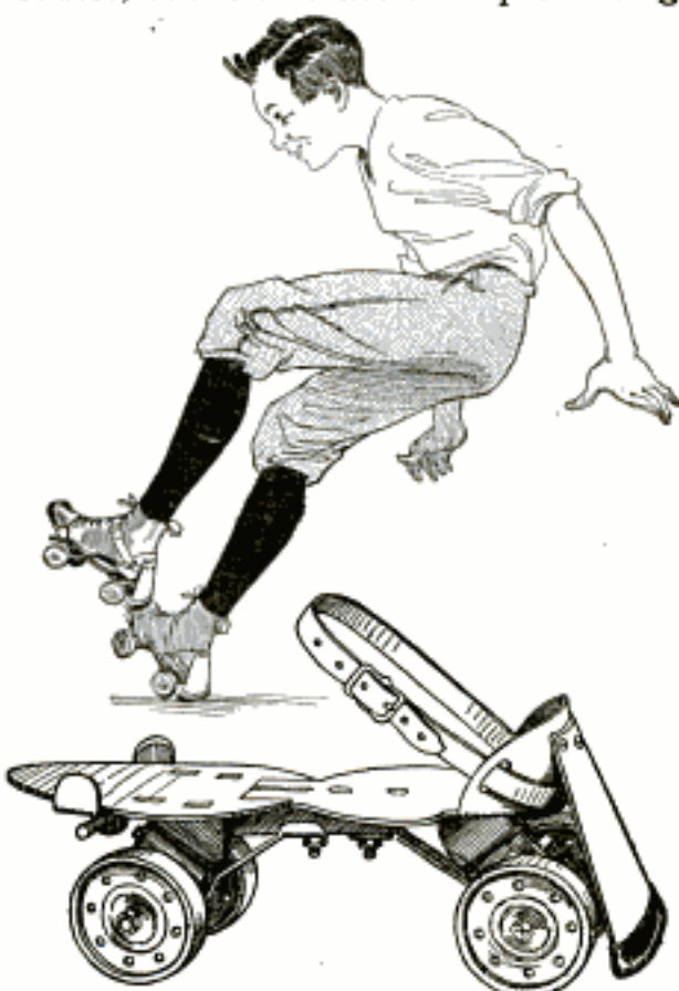
When the Roller Skate Tips Backward the Rubber Tip Comes in Contact with the Floor and Acts as a Brake
