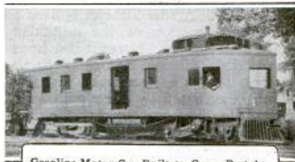
Gasoline Motor Car Built to Carry Freight and Express on a Minnesota Railroad
