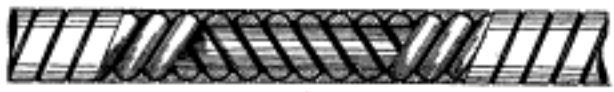
This New Flexible-Shaft Casing Bends Readily, but Flies Back to a Straight Line the Instant the Bending Force is Removed
