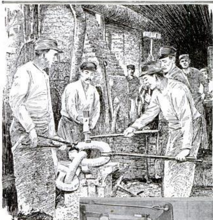
Links for the Chain Cables of Seagoing Vessels are Made by Hand from Iron Rods 32 Inches Long and Nearly 2\frac{1}{4} Inches in Diameter
