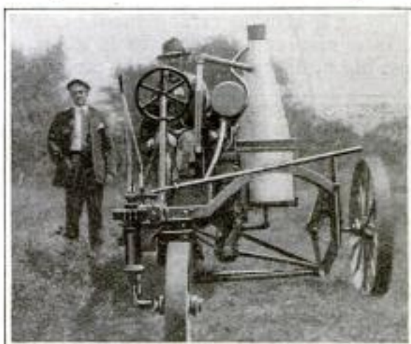
Gasoline Mowing Machine Which may be Used Also for Plowing or Cultivating
