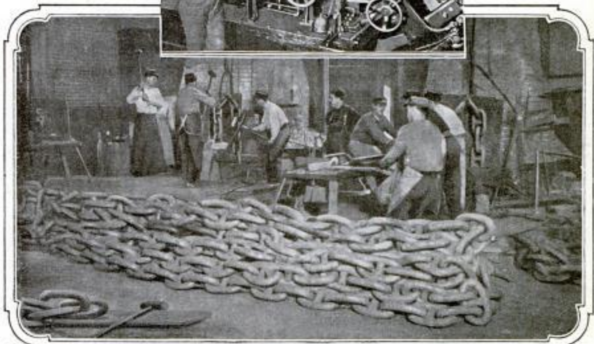
Scene in the Blacksmith Shop of a Chain-Making Establishment: The Completed Chain Shown in This Picture is Made to Withstand a Breaking Strain of from 250 to 375 Tons
