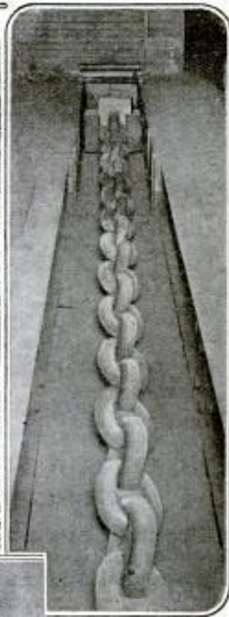
Chain in Steel Trough Ready for the Breaking Test. View of Testing Machine at Left
