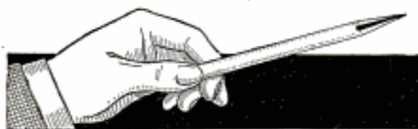
A Notch Cut in the Tapered Part of a Wood Stick Forms a Substitute Pen
