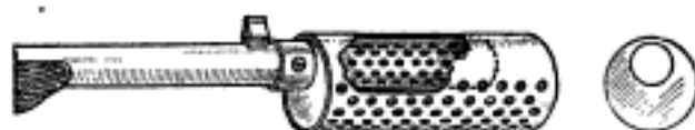
Rifle Silencer Made of Two Pieces of Perforated Steel Tubing of Different Sizes
