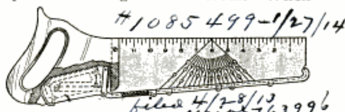
This Saw is Equipped with a Folding Shield for Protecting the Teeth, and is So Made That It Comprises a Protractor, Rule, Straightedge, and Try-Square
