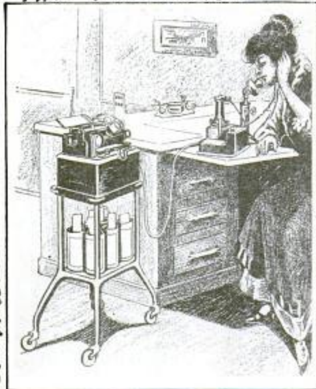
Telephone Recording Apparatus as Used with an Ordinary Desk Telephone
