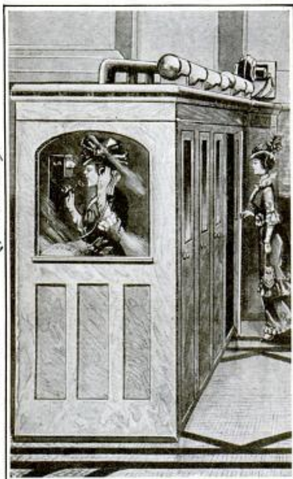
A Complete Change of Air in These Telephone Booths is Made Each Minute
