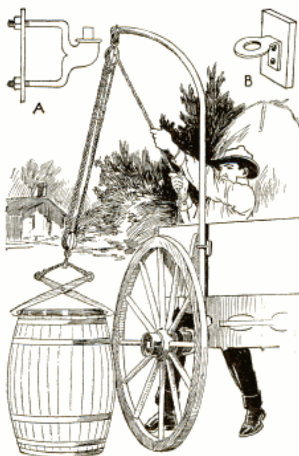
Wagon Crane Made of a Length of Gas Pipe with a Block and Tackle Attached
