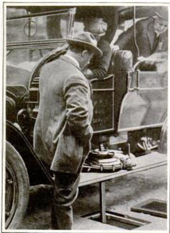
With This Device, Run by the Transmission of an Automobile, a Gate Valve Requiring 307 Turns is Opened or Closed in 10 Minutes
