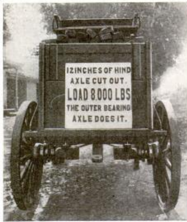
This Wagon, with Axle Equipped with Outer Bearing, Carried a Load of 8,000 Pounds with the Center of the Axle Entirely Cut Away
