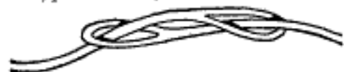
An Endless Thong is Made with Eyes Cut in the Ends of the Leather, and Each Part is Run through the Eye of the Other
