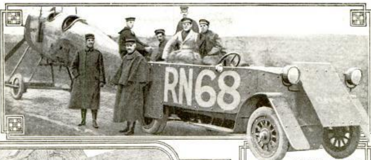
A British Armored Motor Towing an Aeroplane Body. The Initials "O. H. M. S." on the Front Stand for "On His Majesty's Service"
