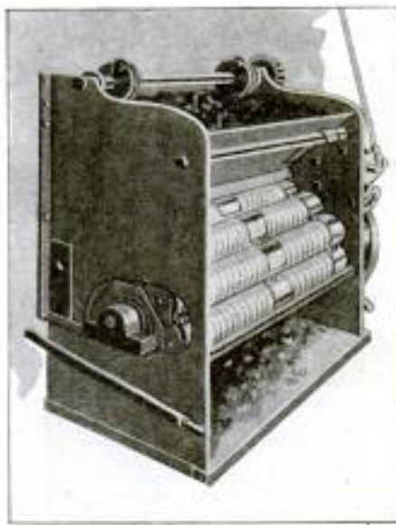
This Stoker Works Like an Ordinary Chain-Grate Stoker but is Made Up of Closely Spaced Disks Mounted on Rotating Bars
