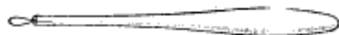
The Horsehair, Being Smooth, will Not Injure the Eye as It is Moved over the Surface
