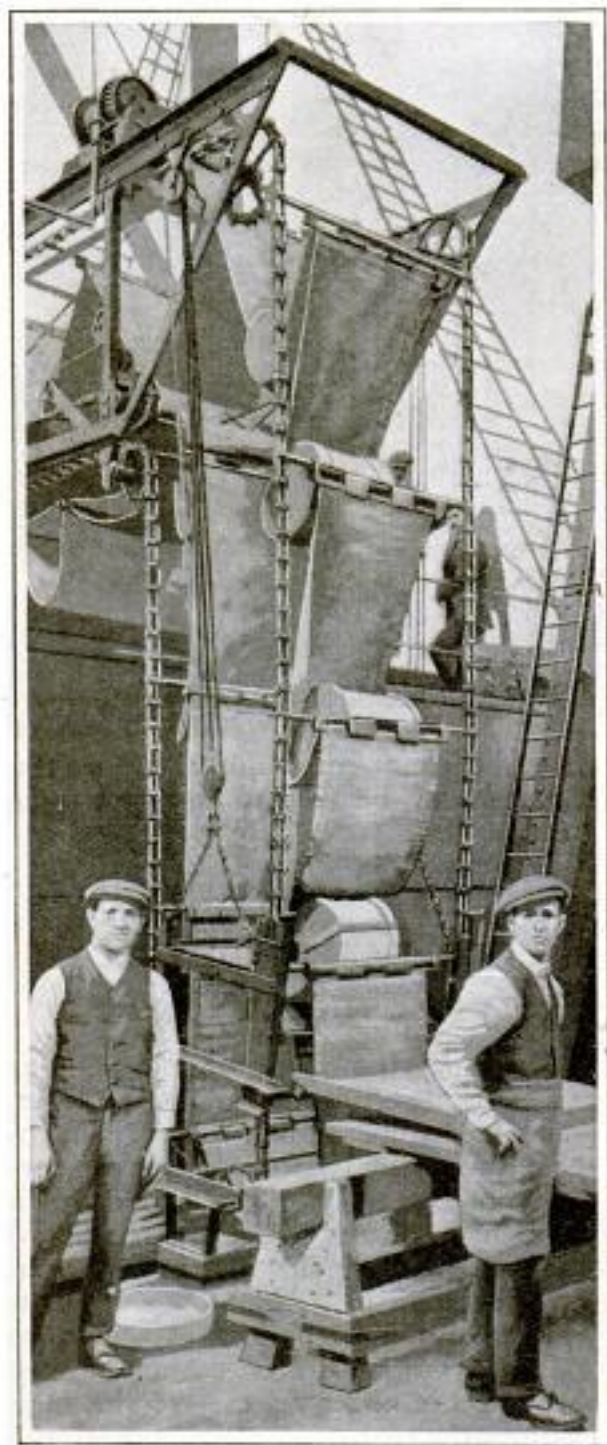
Combined Elevator and Conveyor at Work at a Liverpool Dock
