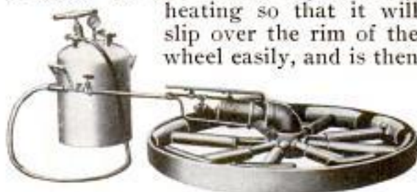
This Heater Uses Kerosene as a Fuel and Heats and Expands the Tire Evenly
