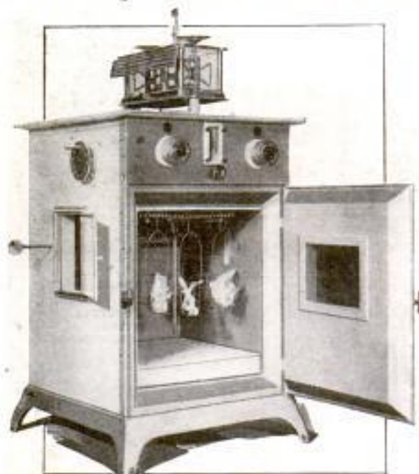
This Oven is Used by the Custom Inspectors in Determining the Duty to be Placed on Imported Cotton Yarns
