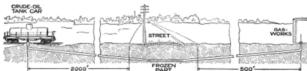
Heating a Long Underground Pipe Line with Electricity to Melt Out Ice Frozen at the Lowest Point under a Street Where It Was Impossible to Get At without Considerable Expense
