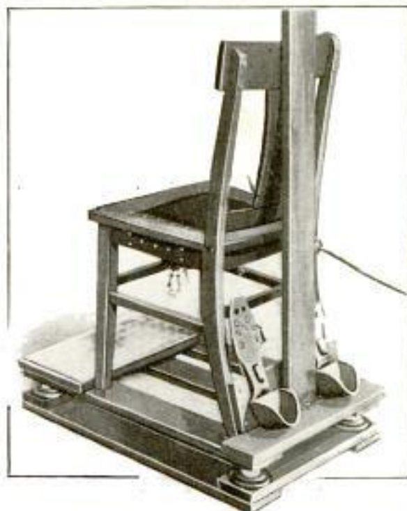
This Vibratory Chair is Mounted on Rubber Balls to Prevent the Communication of its Impulses to the Floor
