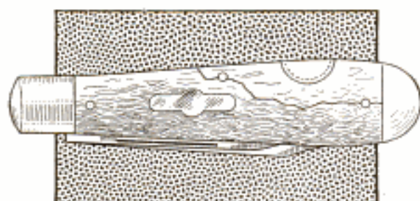
A Piece of Solder, Fastened to the Metal of the Knife, Holds the Broken-Off Horn in Place
