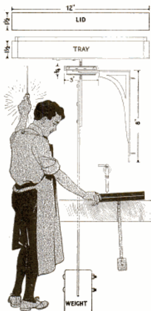
Developing-Tray Rocker to Keep the Liquid in Motion over the Plate Automatically
