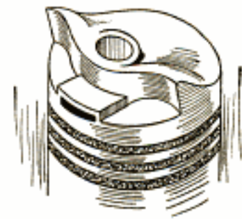
The Piston of This Two-Cycle Engine is So Designed That It Operates Efficiently with a Small or Heavy Charge, Making the Engine Suitable for Driving an Automobile
