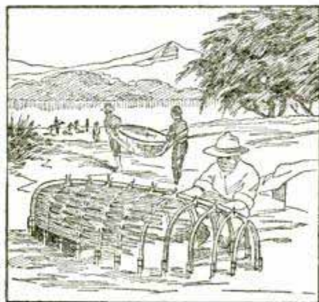
A Boat Made by an Army Corps from Willow Branches and Covered with a Wagon Sheet in About One Hour and Used with Success to Carry 1,000 Pounds across a River
