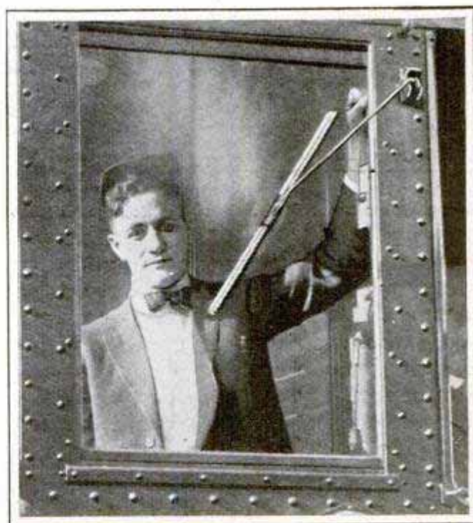
Device Which Prevents the Vision of a Motorman from being Obstructed during a Storm
