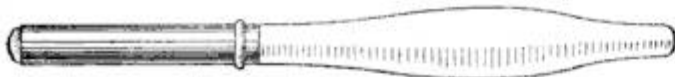
A Small Torch Made of a Penholder is Handy to Use in Soldering Electrical Apparatus
