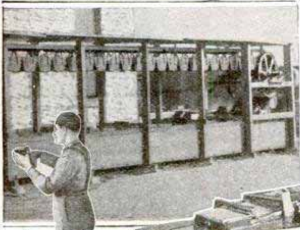
This Machine Arranges the Splints in Parallel Rows and Feeds Them into the Hoppers of the Match Machine, Where a Setting Head Drives Them into Perforated Steel Plates. At Right: Steel Plungers Push the Finished Matches Out of the Perforations
