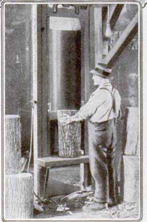
The Curved Blade of the Barking Machine Strips Off the Bark, Preparing the Log for the Peeler
