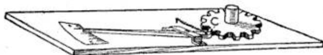
Revolving the Wheel with an Irregular Periphery Causes the Pointer to Indicate the Outline
