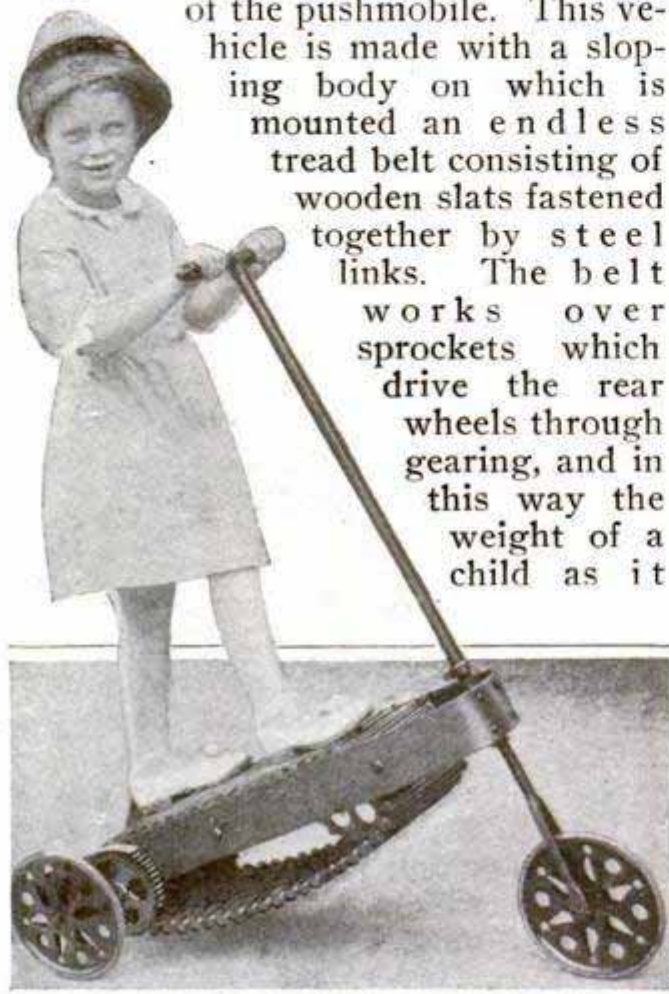
This Vehicle is Propelled by the Weight of the Child as It Walks on the Endless Tread Belt
