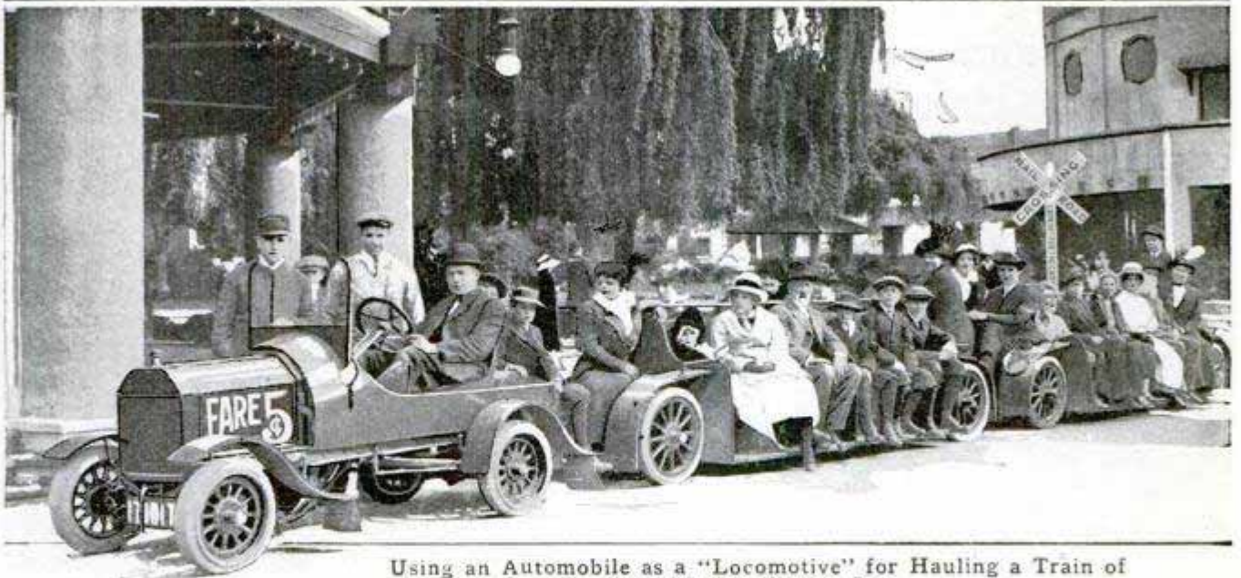
Using an Automobile as a "Locomotive" for Hauling a Train of Sight-Seeing Trailer Cars
