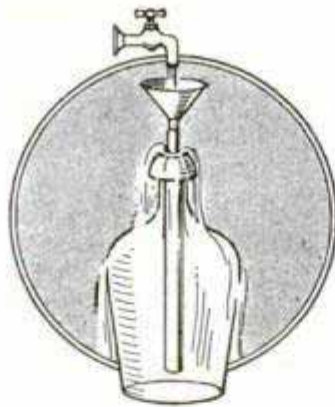
Apparatus Which Cools Liquids without Using Ice
