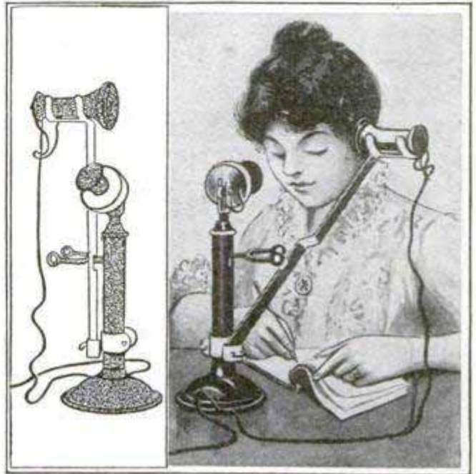
This Telephone Arm Automatically Opens and Closes the Connection and Leaves Both Hands Free
