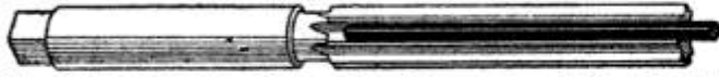
Small Rod in the Flute of a Reamer to Make it Cut Oversize
