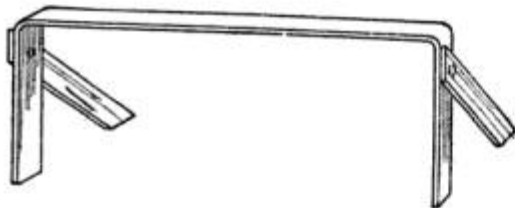
A Support to Keep the Weight of the Fuel from the Paper While Starting a Fire
