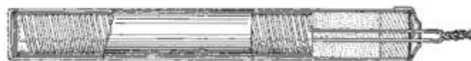
An Electric Heating Coil Made of Resistance Wire Placed in a Bicycle-Pump Barrel for Boiling Water
