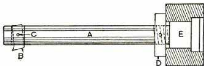
An Oscillating Cutter in a Bar to Provide Clearance for the Edge on the Back Stroke
