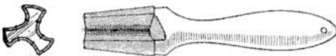
The Notches Catch the Dirt as It is Loosened from the Center Bore
