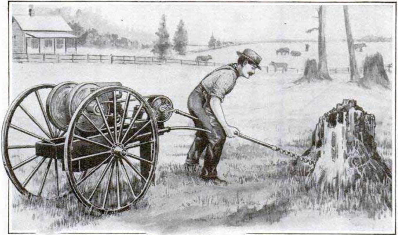
Portable Machine Which is Designed for the Quick Removal of Stumps
