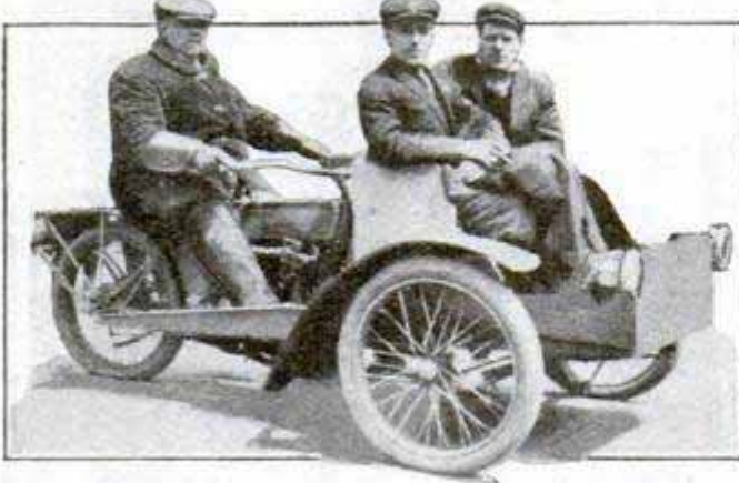
Passenger Body Attachable to Cycle Delivery Truck
