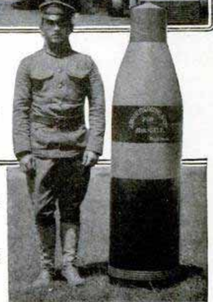
This Shell is Built for the 16-Inch Coast-Defense Guns Guarding Panama Canal, and Weighs 2,400 Pounds
