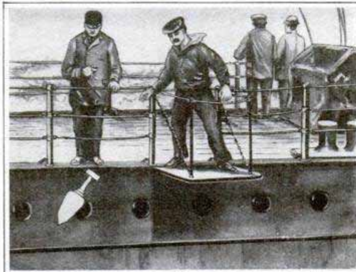
Sounding Bomb Which Explodes When Bottom of Ocean is Reached
