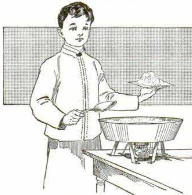
The Disk is Driven by a Small Battery Motor and Melted Sugar is Spun Out into Floss
