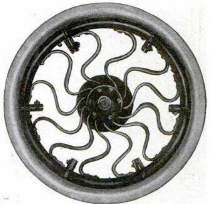
Automobile Wheel with Spring Spokes and Sectional Fellys That Move In and Out to Adjust the Tire to Irregularities in the Road
