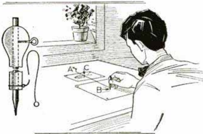
The Size of the Enlarged Picture Depends on the Length of the Elastic and the Spacing of Pencil and Pointer
