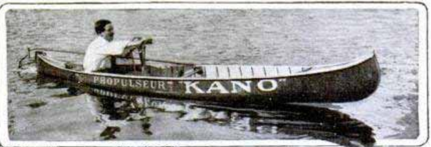
A Canoe Propelled by Hand-Operated Cranks Made Fair Speed
