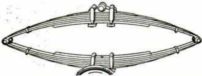
Curved Rigid Bar Clamped to Concave Side of Spring Prevents Rebound beyond Normal Position
