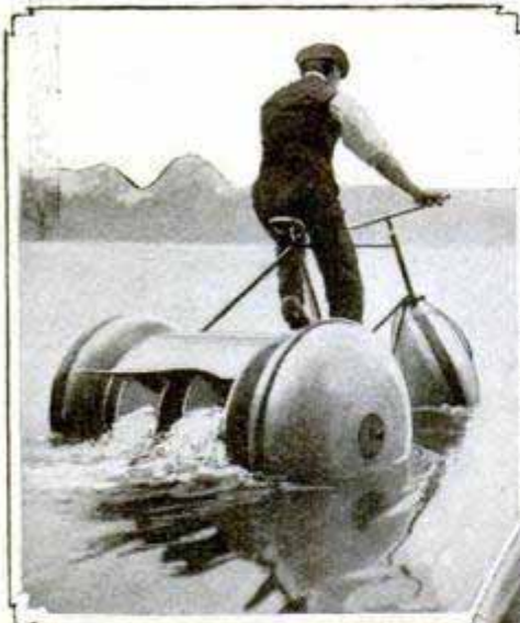
This Craft with Rotating Floats could Also be Driven by an Air Propeller
