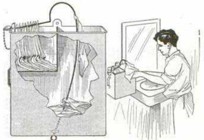
The Towels are Simply Lifted Out of the Reservoir at the Top of the Case and around the Wire Loop, and after being Used are Dropped into the Closed Receptacle Below
