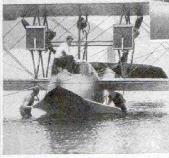
The Planing Fins, Affixed to the "America's" Hull, Which Help It Get Out of Water under Load
