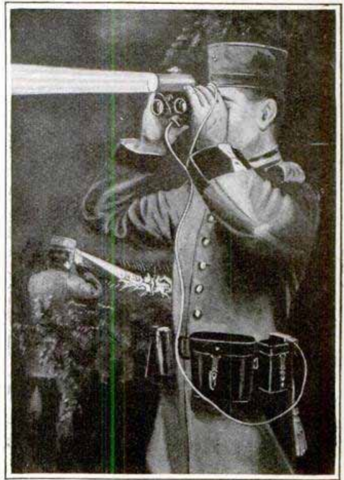
Electric Optical Apparatus Used at Night by German Army for Signaling
