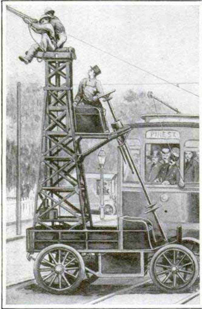
The Working Platform of This Tower Wagon is Easily Raised or Lowered, While the Driver is Provided with Two Seats, One at High and the Other at Low Level
