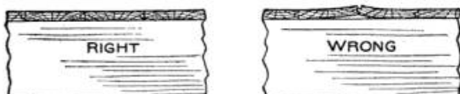
The Right and Wrong Way of Laying a Floor: The Former Prevents the Board from Warping
