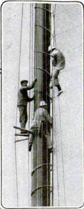
Trimming Sail on the "Shamrock IV" during Trial Run in the Solent Channel: This Hollow Mast, 160 Feet High, is Built of Strips of Fine Silver Spruce and Cost about $3,000
