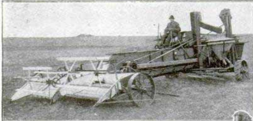
Side View of Machine Which Performs Every Operation Attending the Harvesting of Grain
