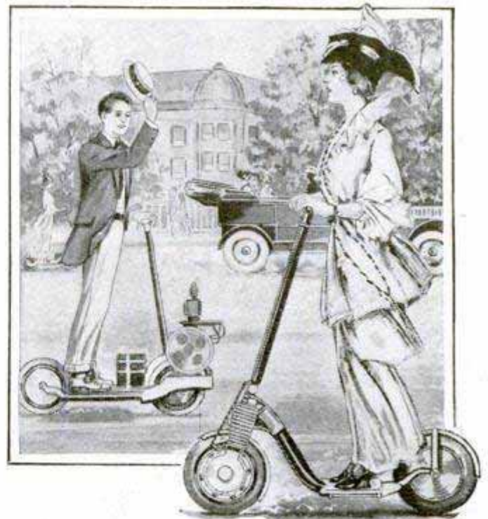
Pushing the Ground with One Foot will Spin the Motor of This Foot Automobile and Start the Machine
