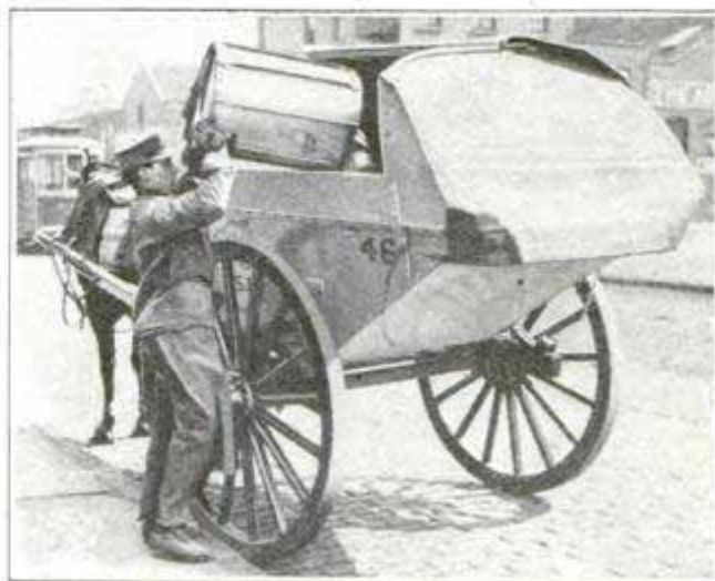
Copyright, American Press Association This Ash Cart Doesn't Scatter Dust in the Wind
