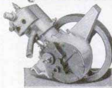
Same Motor after All Pieces had been Welded into Place by Gas Welding Machine
