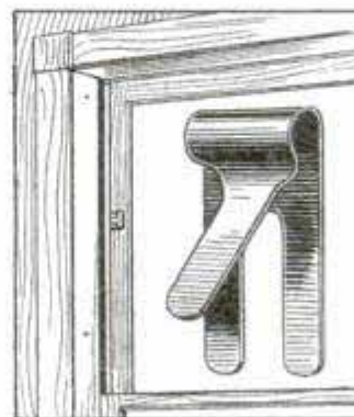
Spring Clip Keeps Sash from Rattling
