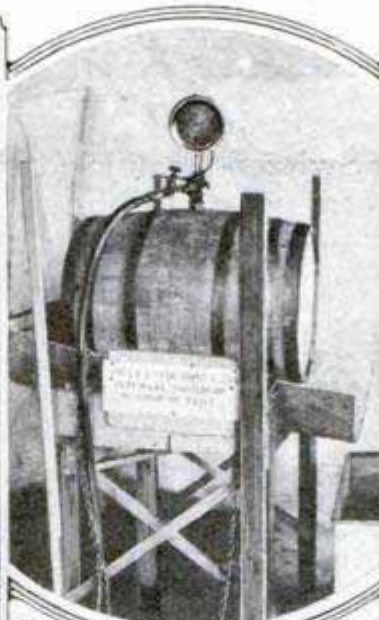
Testing a Barrel for Internal Pressure in the U. S. Forest Laboratory
