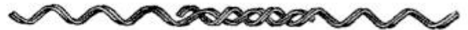
The Coiled Wires When Turning Give the Appearance of Coming Apart Where They are Joined
