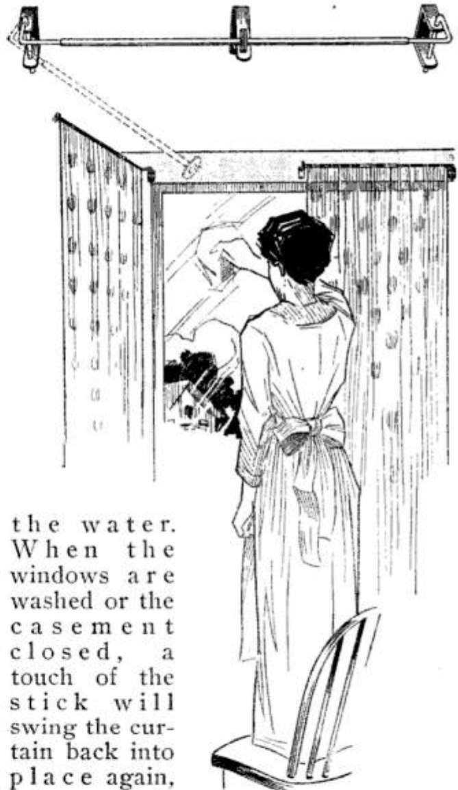
Novel Device Keeps Curtains Out of the Way When Washing Windows
