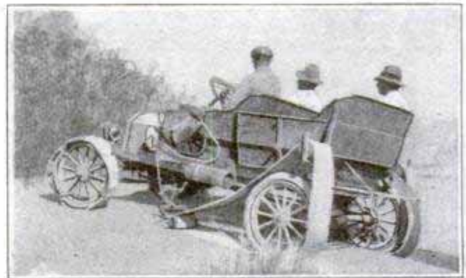
The Wide Belt Prevents the Wheels from Sinking into the Sand
