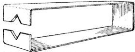
The Notched Ends of the Steel Cut and Remove the Insulation as the Wire is Drawn through Them
