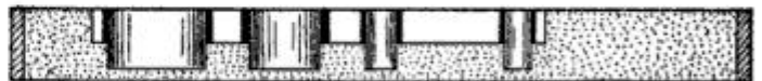
A Mold Made in Plaster without a Special Pattern and Run with a Soft Metal
