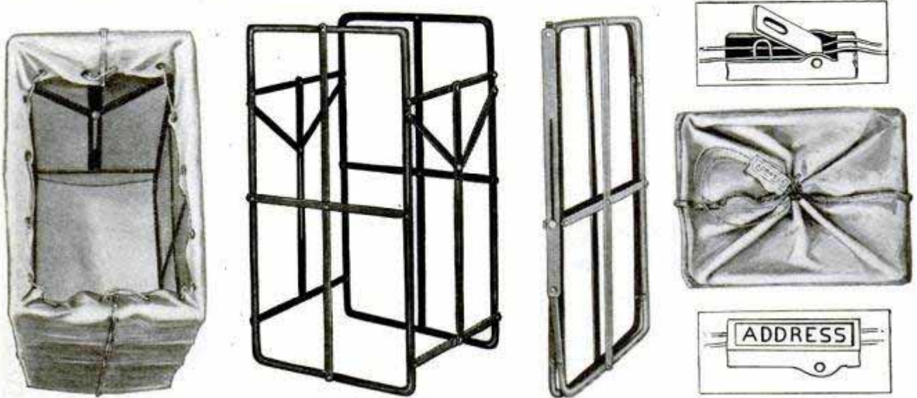
Convenient Carrier for Use in Big Stores may be Compactly Folded for Return
