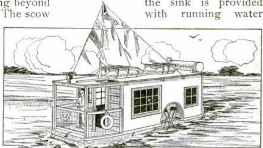
The Hull of the Houseboat is Built on the Scow Type so That It can be Run in Shallow Water without Danger
