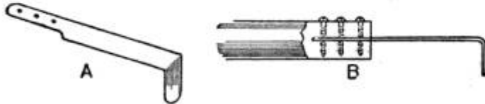
A Case-Knife Blade Bent and Fastened in a Broom Handle Makes an Excellent Weeding Tool
