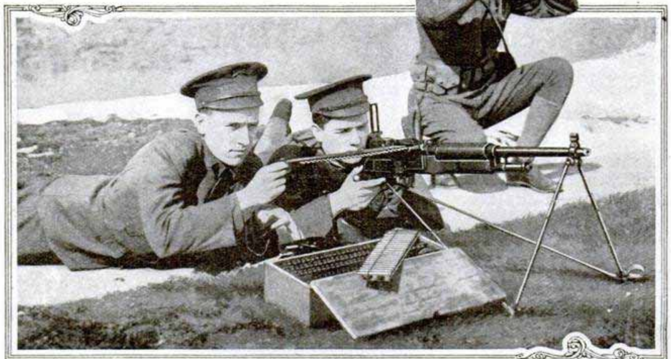
This New Machine Gun Rests upon a Low Tripod about a Foot above the Ground. It may be Made to Fire 300 Shots a Minute
