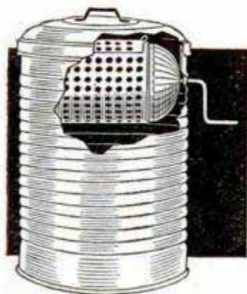
Rotary Ash Sifter Rendered Dustless by Cover
