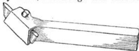
A Combination Tool Holder Using a Wedge Instead of a Screw for Clamping the Cutter
