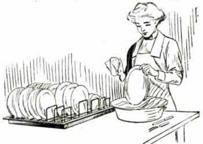
Dish Drier That Consists of Pan with Wire Rack for Holding Dishes on Edge
