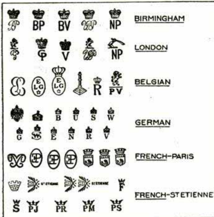
Proof Marks Used by European Gun Makers to Indicate the Quality of Their Guns
