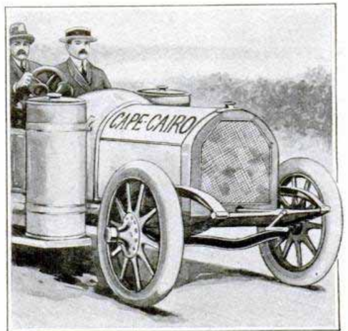
How an Extra Supply of Gasoline is Carried for Long Journey
