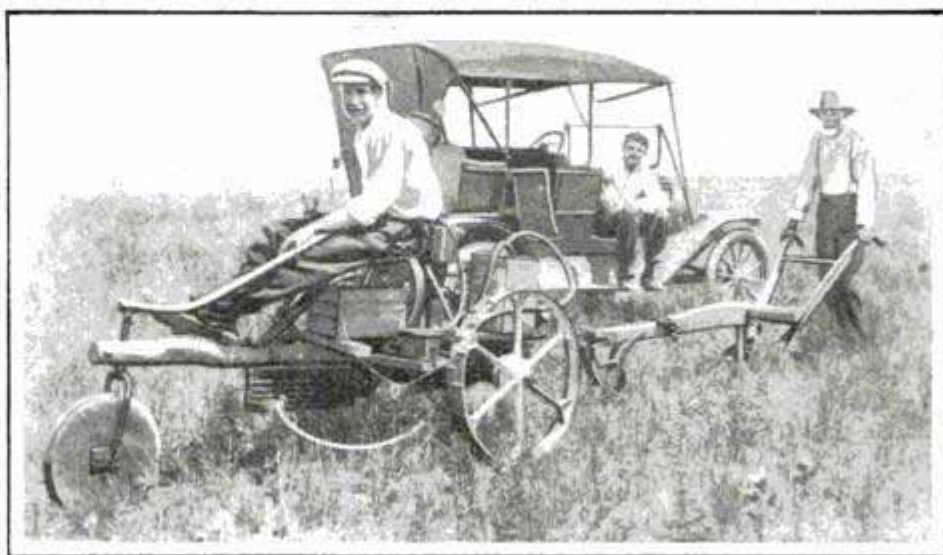
Homemade Farm Tractor Built of an Old Mowing Machine Plus a Marine Engine
