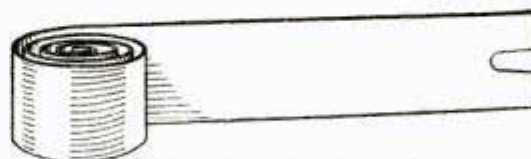
A Strip of Tin Shaped to Take the Place of a Rivet Set
