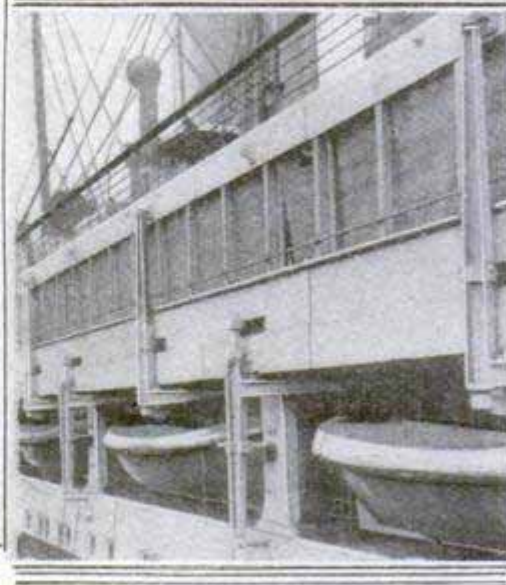
One of the Traveler's First Concerns is the Lifeboat Equipment. On the Left are Shown the Collapsible Boats and the Winch That Launches Them; on the Right, Other Boats, Lowered from Rotating Arms
