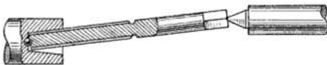
A Straight Reamer, the Shank of Which is Offset with the Tailstock, will Cut a Taper Hole
