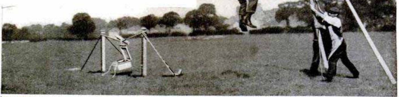
Bringing In a Man on the Breeches Buoy: For Test Purposes the Line was Fired over a Point 1,050 Ft. Distant and the Man was Brought In under the Same Conditions as would Prevail at Sea. The Equipment for Firing the Rocket is Shown at the Left
