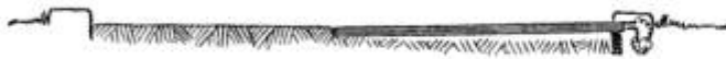
Trip Bar in an Entrance Runway to Make Connections for an Inside Electric Bell
