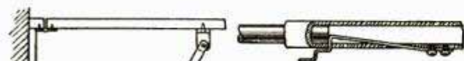
When the Shelf is Lowered the Support Telescopes and is Out of the Way
