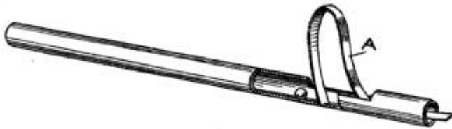
A Pea-Shooting Gun Made of a Piece of Alder and a Corset String
