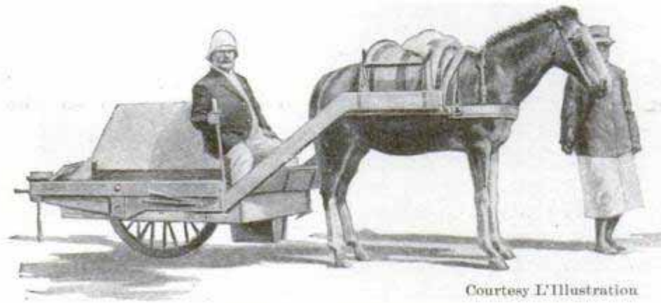
Courtesy L'Illustration Practical One-Wheel Truck for Use in African Brush
