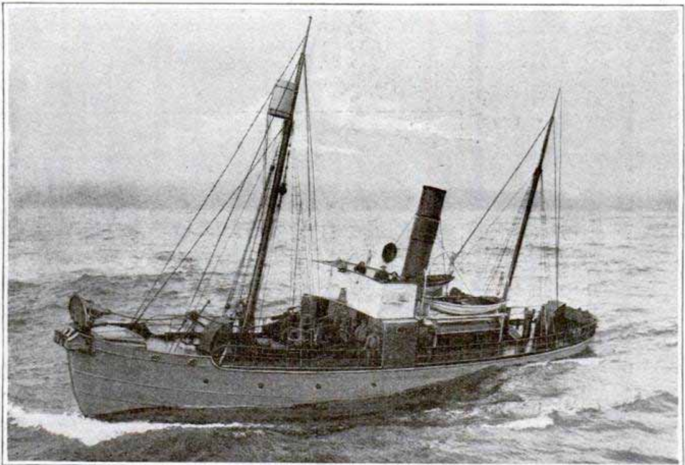
A Modern Steam Whaling Ship, with Harpoon Gun Mounted in the Bow
