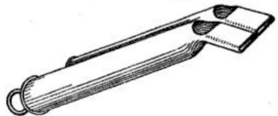
The Tapering End of a Cartridge Shell is Flattened and Bent to Make a Whistle
