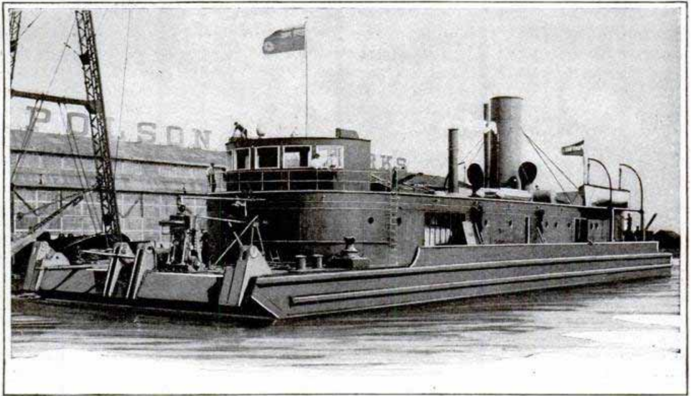
Seagoing Suction Dredge That will be Used for Excavating Harbors in Hudson Bay, in Connection with Short Route from Canadian Northwest to Europe
