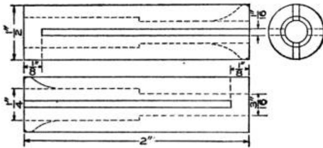
A Draw Collet Having a Different Diameter in Each End for Small Mills
