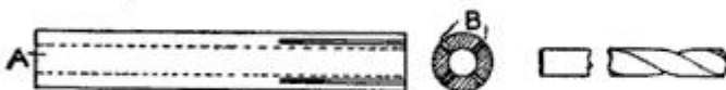
Each Small Drill was Supplied with a Chuck to Fit the Lathe Chuck
