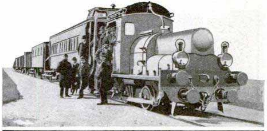
Internal-Combustion Locomotive That Uses Naphthalene as a Fuel
