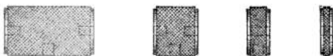
Gauges Cut from Tool Steel, Hardened, Then Their Faces Ground True to Size
