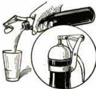
Device for Closing Bottles That Contain Effervescent Liquids
