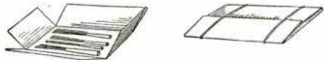
A Holder Made of a Match Box to Provide a Place for Keeping Striping Brushes
