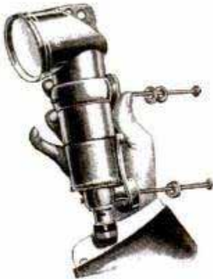
New Type of Automobile Headlight Which Throws Light Beams Forward and Downward Only
