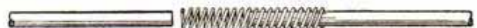
A Coil Spring Used for Splicing Sash Cords or Small Round Belts
