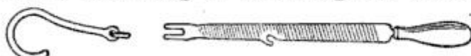
A Tool for Holding Springs While Valves are Being Removed for Repairs
