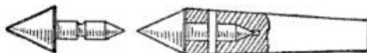
A Revolving Lathe Center That will Prevent Wear on Work Running at High Speed
