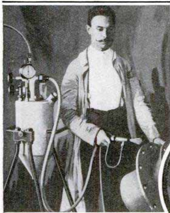
Apparatus Used in New Process of Plating with a Spray of Molten Metal
