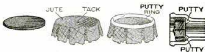
Series of Operations in Making the Parts to Plug the End of a Soil Pipe
