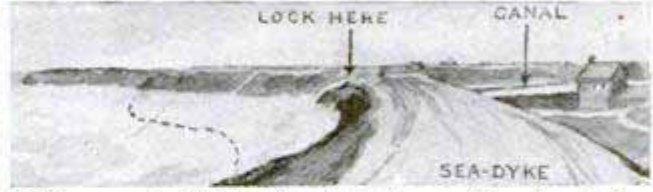
Difference in Water Levels between Canal and Sea
