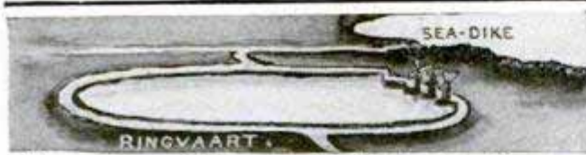
Water Pumped from Enclosed Lake into Canal
