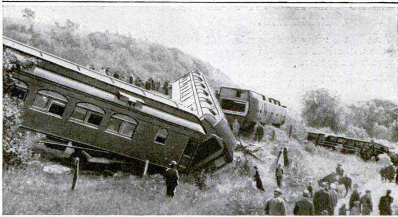
Only One Passenger Fatally Hurt in This Accident, Where Steel Cars Saved Many Lives
