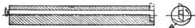
The Revolving Cutter will Easily Make the Recess without Springing Away from the Work
