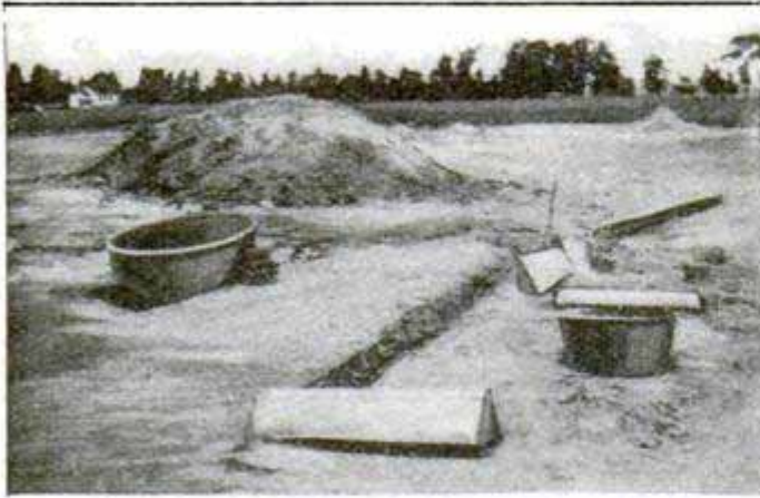
A Pile of "Ore" Harvested from a Gun Club's Grounds; Lead Mold at Left and Lead "Pig" in Foreground
