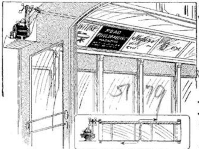
Moving Street-Car Signs Which Travel from One End of the Car to the Other, Driven by Electric Power
