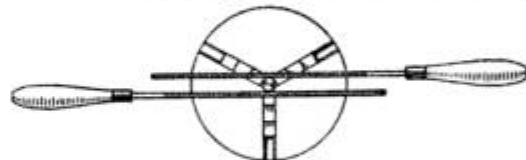
The Pressure of One File Against the Other Prevents the Rod from Bending
