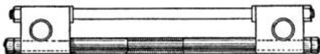
A Piece of Pipe and a Long Rod Taking the Place of a Broken Bar
