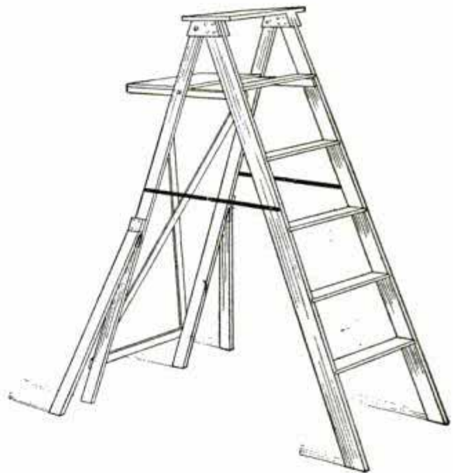
The Strips Hinged to the Back-Support Sides Prevent the Ladder from Tipping Over Sideways
