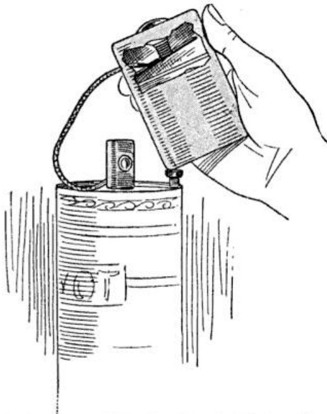
An Instrument Made of an Electrical Pocket Flash Light for Testing Circuits and Instruments
