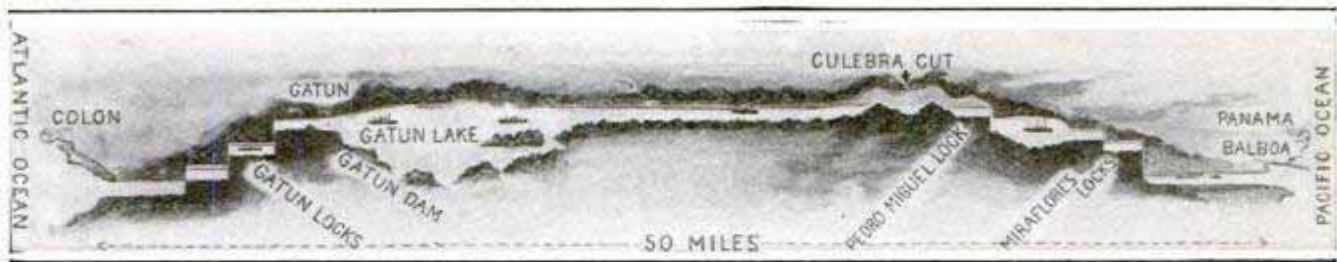
Profile of the Panama Canal, Showing the Different Levels from Ocean to Ocean
