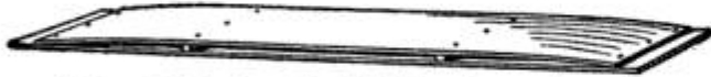
A Board Used on Scaffolding Strengthened to Prevent Sagging in the Center
