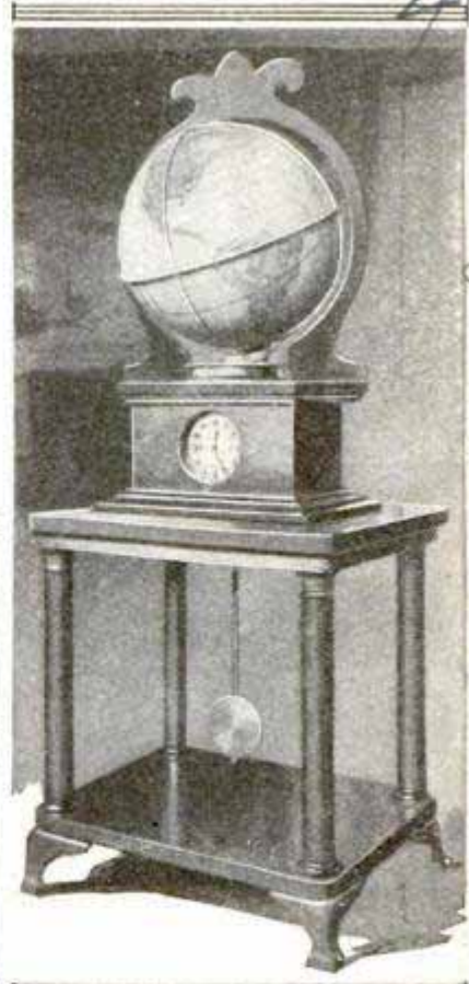
Sidereal Globe Which Indicates the Time in Various Parts of the World
