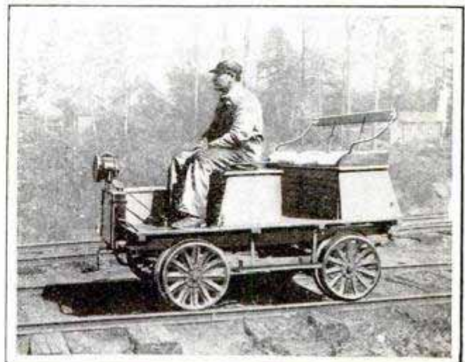
Handcar, Converted Into Track Automobile, Used for Branch-Line Service
