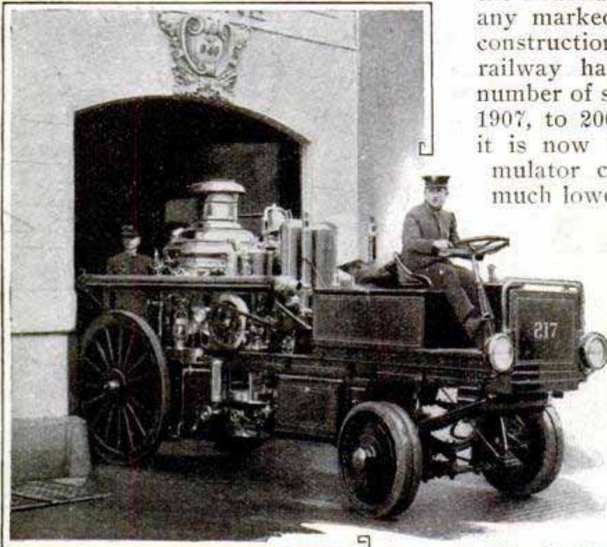
Courtesy The Edison Monthly Electrically Driven Fire Engine in Service in the New York City Fire Department
