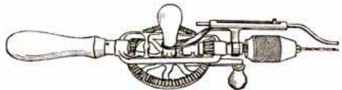
The Support on a Breast Drill for Preventing the Breaking of Small Drills
