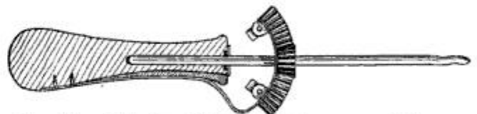
Revolving Spindle will Quickly Loosen and Remove Any Dirt or Caked Oil in a Hole
