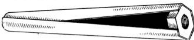
The Holder Made of Sheet Metal Grips a Nut to Start It on the Threads
