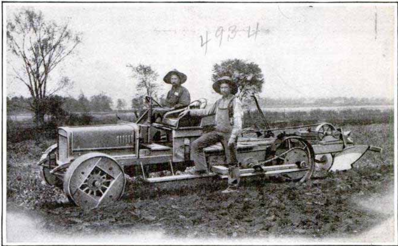
Homemade Power Plow Made of an Old Automobile
