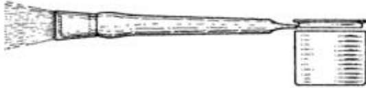
The End of the Paint-Brush Handle is Shaped to Insert under the Cover Edge
