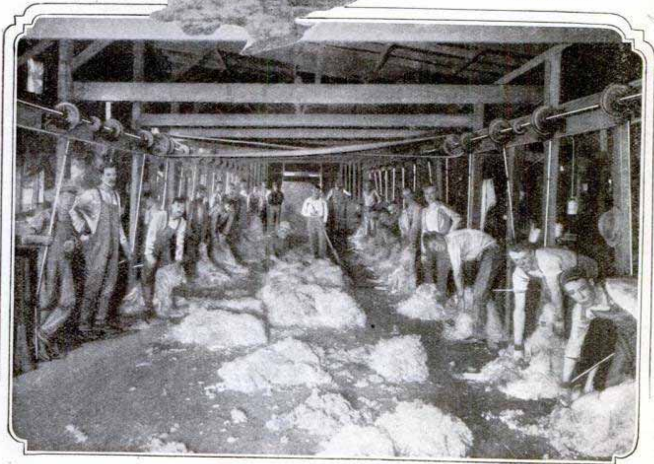
Below: Power Shearing Machines Used on a Large Sheep Ranch in Wyoming
