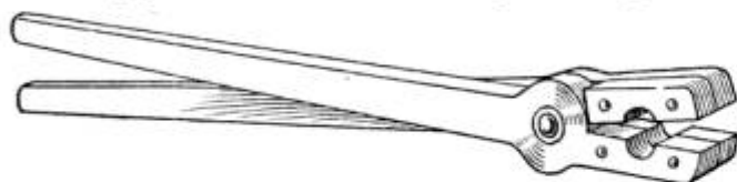
The Parts Forming the Handles and Jaws of the Pliers are Made of Heavy Sheet Fiber
