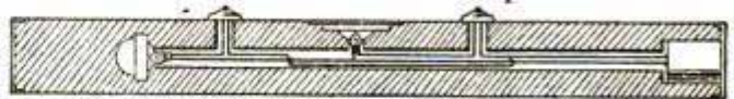
When the Level is Used in a Dark Place, the Light can be Flashed on the Bubble Glass
