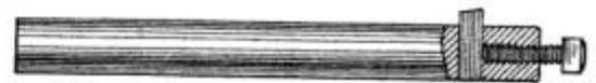
Tool to be Placed in a Drill-Press Chuck and Used for Cutting Keyways
