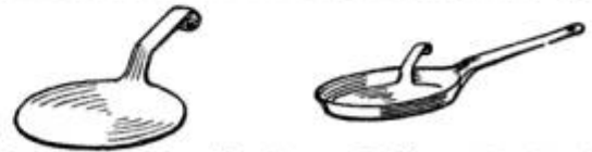
A Metal Plate for Use in an Ordinary Frying Pan to Cook Eggs without Scorching Them
