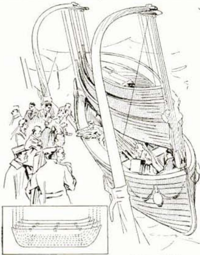
Steel Lifeboat with Inner and Outer Hulls
