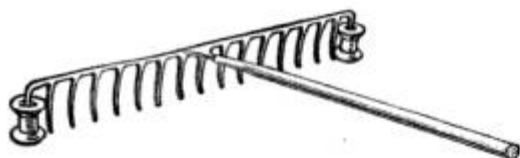
The Spools Prevent the Teeth from Injuring the Grass Roots as the Rake Passes over the Ground
