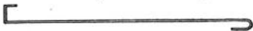
The Hook Prevents Making Holes in the Finished Roof, and the Staging is Much Easier Raised
