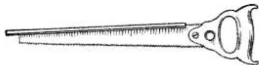
The Teeth on the Unused Edge are Covered with a Piece of Brass Curtain Rod
