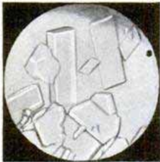
Fig. 1—Photograph of Nitroglycerine Crystals in Labile Form Which Experiments Show will Not Explode So Easily As in Other Form
