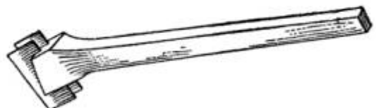
The Blades are Set in the Wood Handle and Spaced to Equal the Width of the Lacing
