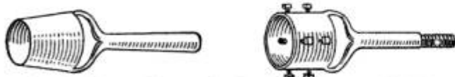
An Ordinary Cutter for Making Shotgun Wads Made into a Jumbo Chuck
