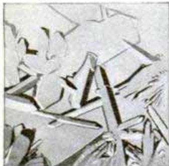
Fig. 2—Crystals of Nitroglycerine in Stable Form, Which Experiments Show to be Safer Than the Liquid
