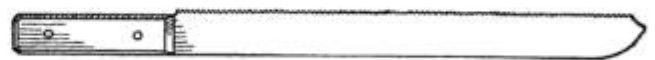
The Blade of the Knife is Cut from the Toothed Side of a Discarded Saw Blade
