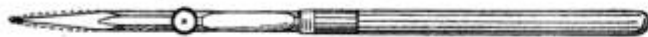
The Shape of a Ruling Pen to be Used in Writing or Making Letters on Tracing Cloth
