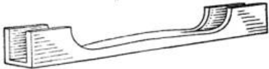
The Construction of the Jaws Makes a Side and End Wrench of One Piece
