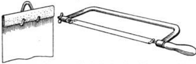
The Strip of Emery Cloth in the Saw Frame is Used in the Same Manner as a File
