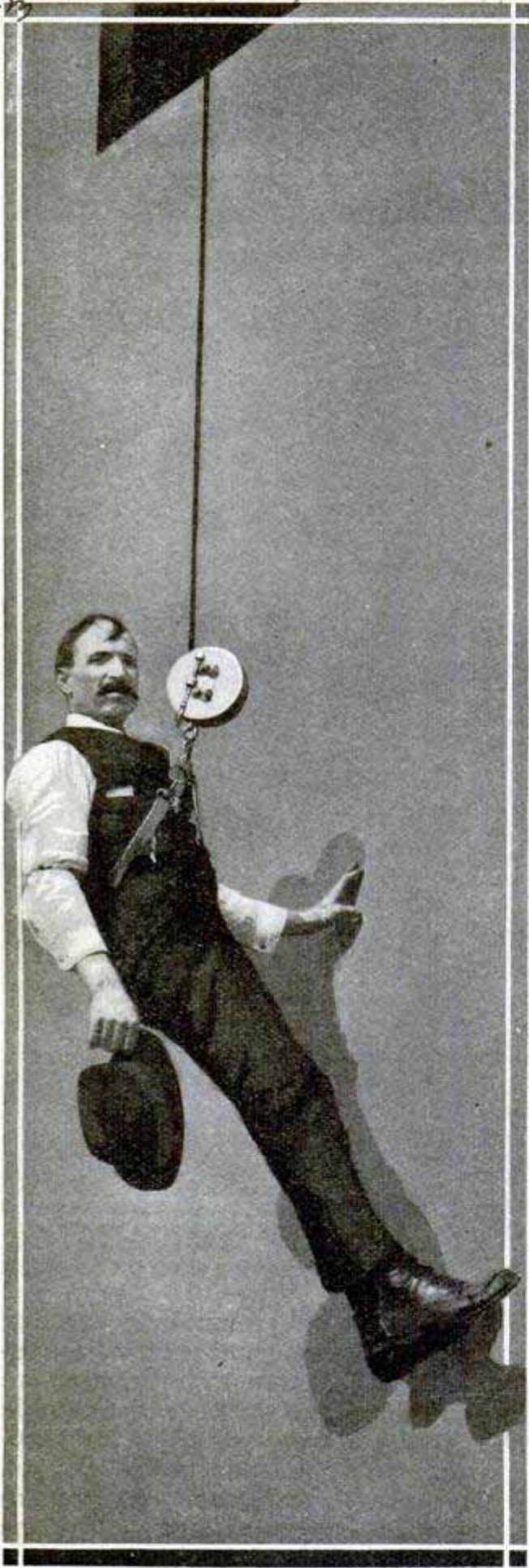
Escaping from a Building in the Same Way a Spider Drops by Its Thread
