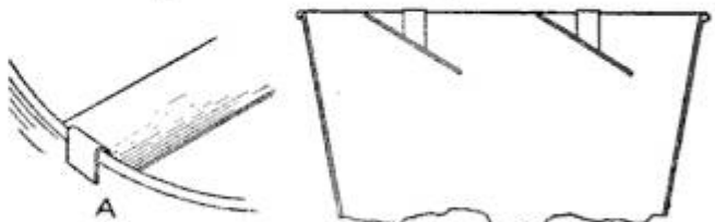
The Strips Allow the Liquid to Enter the Pail, but It cannot Splash over the Edge
