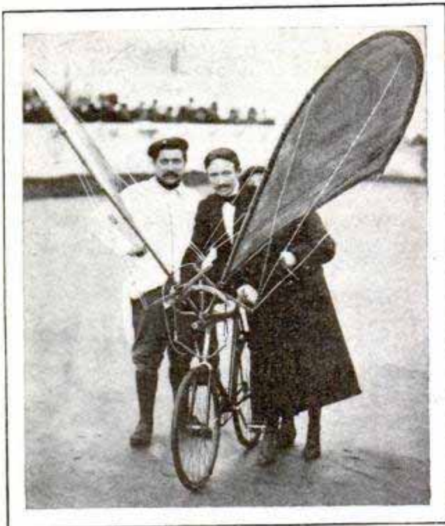
Aviette with Jointed Wings, the Wings being Lowered to a Flying Angle When Sufficient Speed has been Attained by Ordinary Bicycle Propulsion
