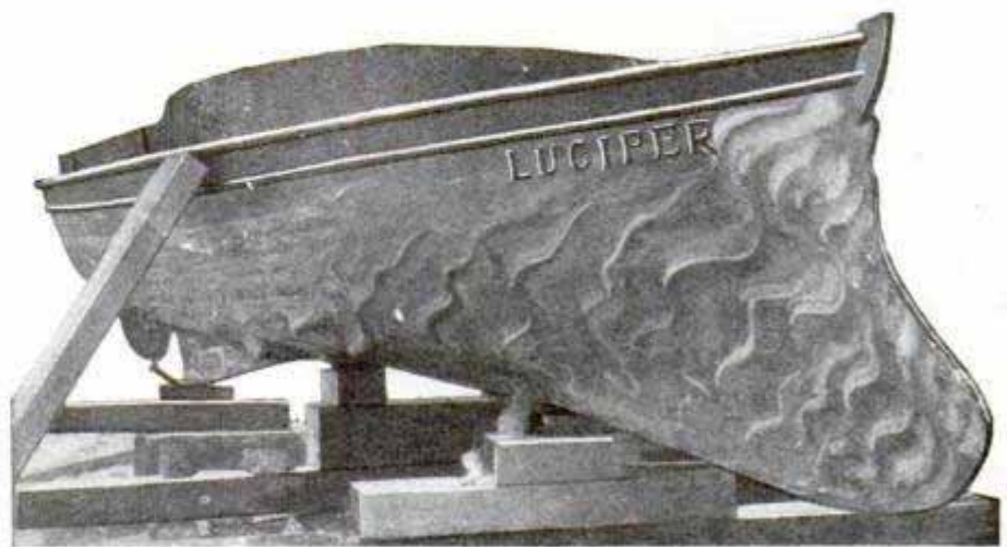
Humps Formed on the Bottom of a Motorboat, with the Idea of Giving Speed
