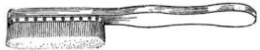
Brush Made of Strip of Upholsterers' Haircloth with the Warp Removed and Fastened to a Handle
