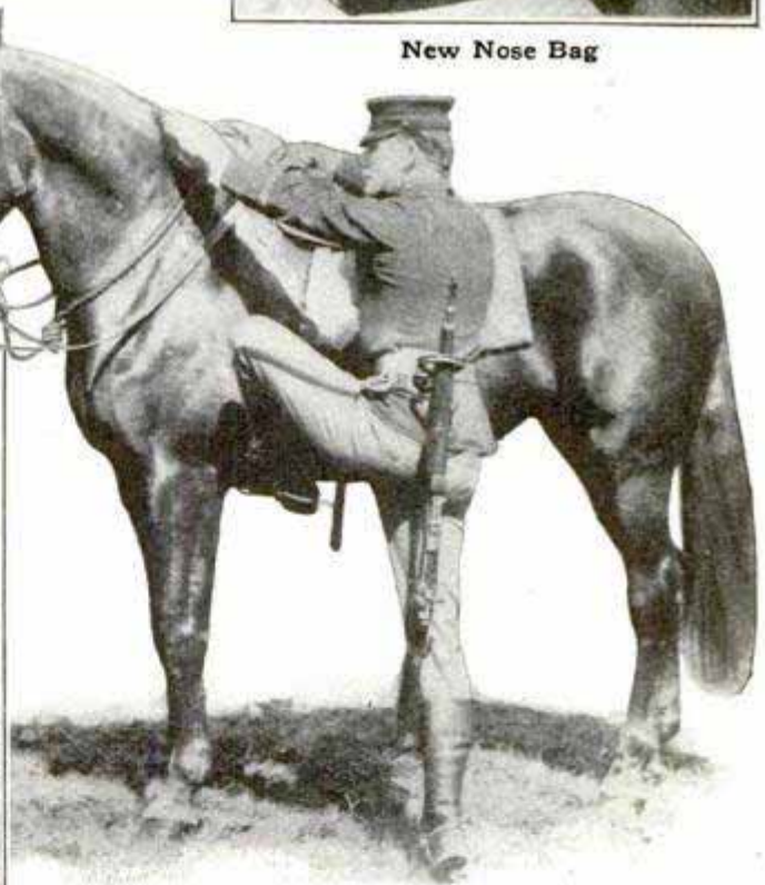
The Rifle Carrier. The Rifle is Hung from the Belt by a Strap, and Held Upright by a Steel Ring on the Belt
