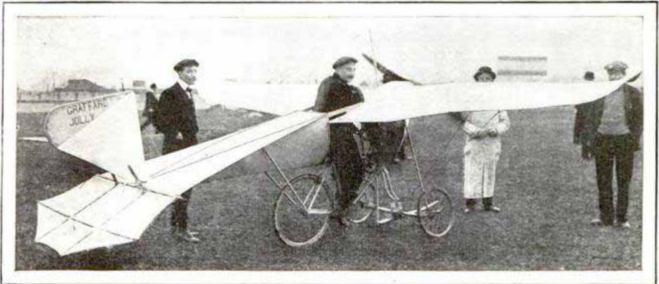
Aviette with Aeroplane Lines, with Power Transmitted both to the Rear Wheel and to a Propeller
