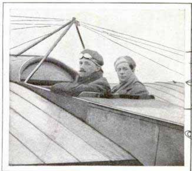
The New Seating Arrangement for Pilot and Passenger Developed in an English Military Aeroplane
