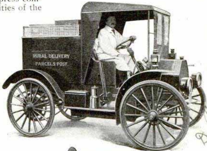
Light Parcel-Post Rural-Delivery Automobile, Designed for Postoffice Service
