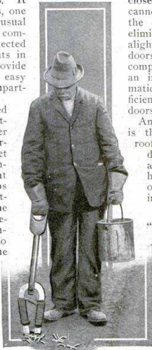
"Magnet Bill" is the Official Preventor of Tire Punctures and Cuts in the Plant of a Toledo Automobile Concern
