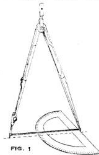
The Extension Marks can be Easily Read on the Protractor under the Elastic Band
