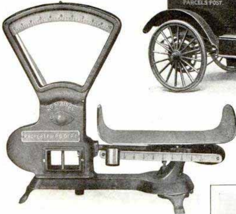
Automatic Computing Scale Bought by the Government for Parcel-Post Branch of the Large Postoffices
