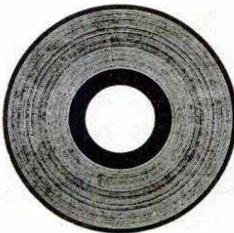
The Paper-Insulated High-Tension Cable Which Carried the First 10,000-Volt Current 23 Years Ago. The Picture Shows Actual Size of the Cable
