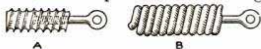
The Expanding Spring Tends to Close the Coils, Thus Gripping the End Piece Tightly
