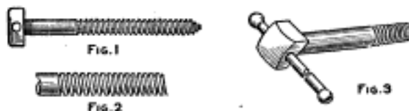
A Vise Screw Formed of an Ordinary Lag Screw, the Threads being Made Square and a Handle Attached
