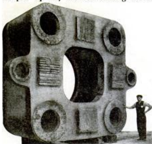
Casting for Cap of 10,000-Ton Forging Press Powerful Enough to Lift an Ocean Liner
