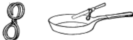
The Shape of the Clip and Manner of Attaching It to a Frying Pan
