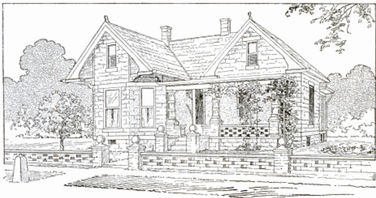
Front Elevation of Low-Price Concrete-Block Home
