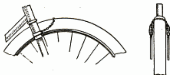
Particles of Glass are Removed from a Tire Casing by the Chain Before They Enter the Inner Tube
