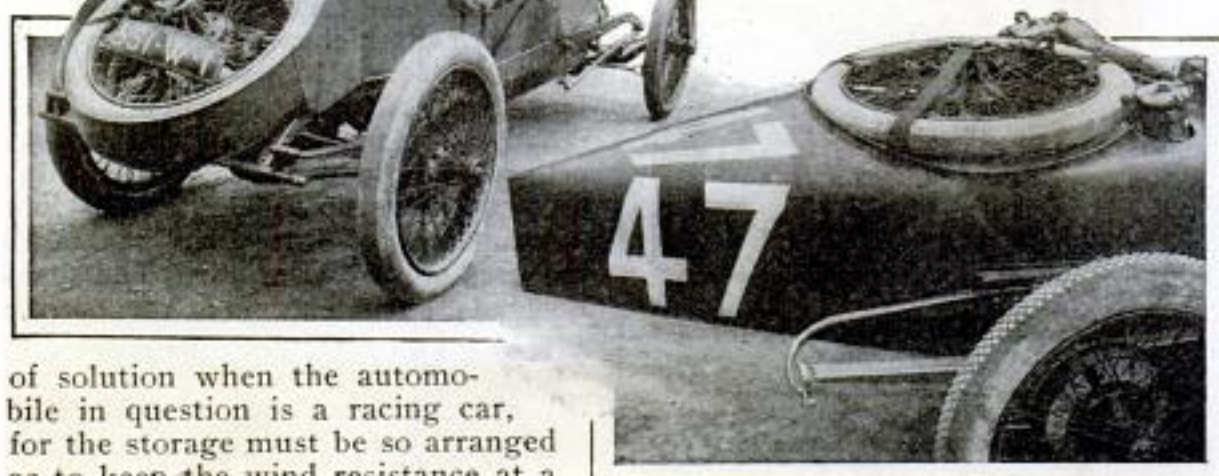
A Lion-Peugeot Racing Automobile, Showing Storage Place for Spare Wheel
