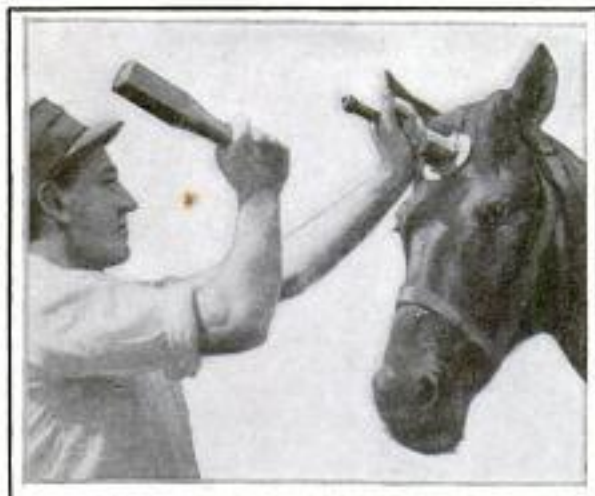
A Horse-Killing Gun, Discharged by Striking a Slight Blow with a Mallet, Which Kills Instantly and Noiselessly
