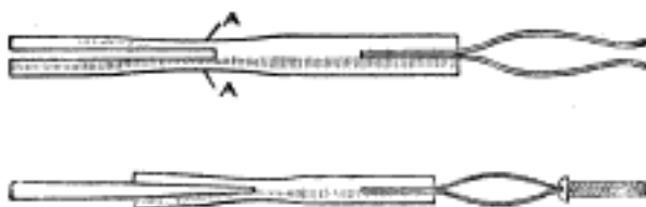
The Screw-Holding Attachment Slips on the Blade of a Screwdriver for Starting a Screw
