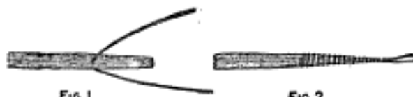
The Wire Prevents the Lace from Raveling and Makes a Tip for Easily Entering the Eyelets
