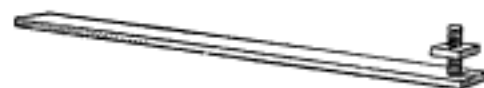
The Nut is Set to the Thickness of the Glass and Used to Break Pieces Away
