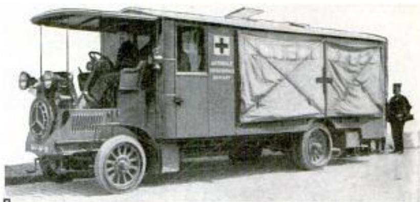
Motor Car in French Maneuvers Equipped with All Modern Appliances for a Surgical Operating Room
