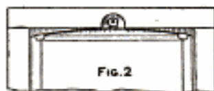
The Spring with Its Clips and Manner of Holding a Negative in a Printing Frame
