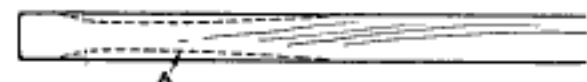
The Handles are Dressed to a Shape Similar to That of an Ax Helve, Producing a Knob on the End
