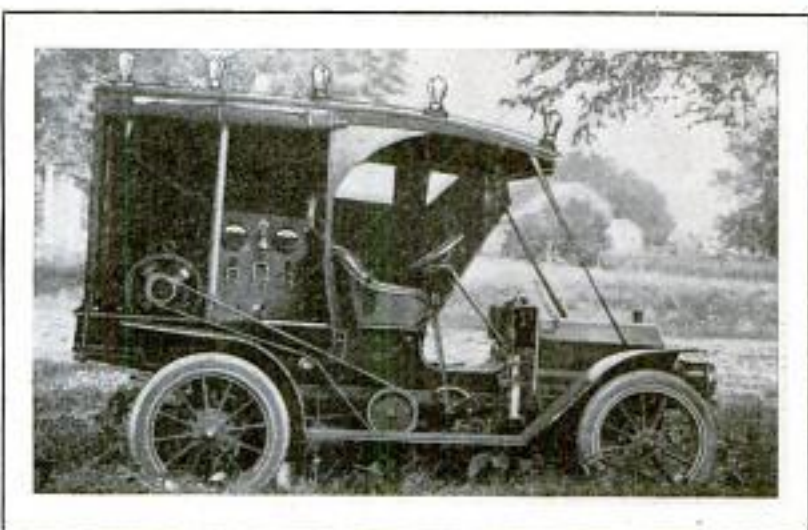
The Automobile Electric Plant Which Furnishes Current for a Traveling Motion-Picture Show
