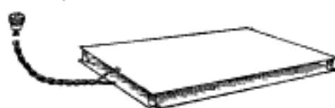
An Inexpensive Electric Water Heater Made of Two Copper Plates
