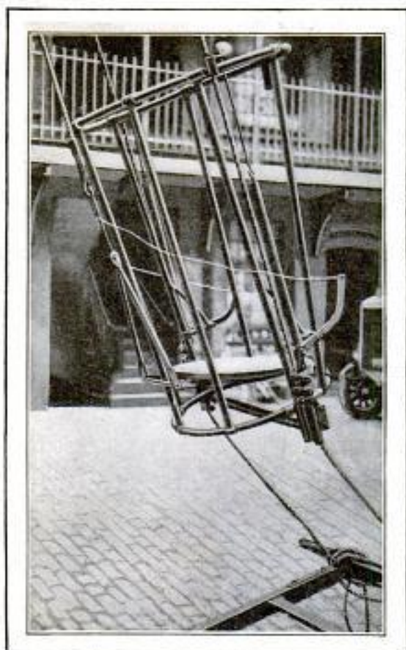
The Cradle or Cage of a New Type of Truck Fire-Escape Tested in England
