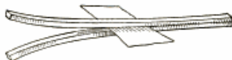
A Piece of Paper Placed between the Red-Hot Parts will Stop a Weld at Welding Heat
