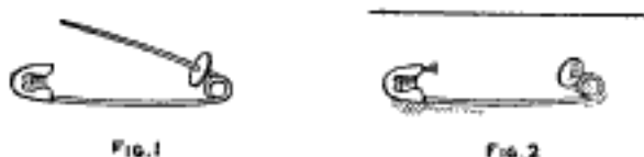
The Small Disk on the Pin Prevents the Goods from Becoming Tangled in the Coil
