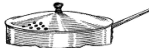
A Sufficient Number of Holes are Drilled in the Edge of the Cover to Make a Strainer
