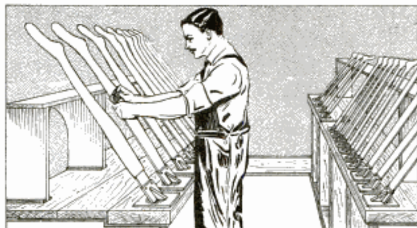
A Battery of Electrically Heated Forms for the Drying and Shaping of Stockings
