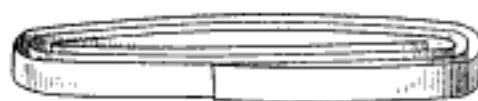
The Filed Edge on the Coiled Metal Retains the Sand Particles as It is Rubbed over the Glass Surface
