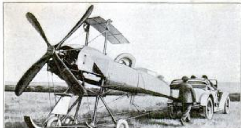
A French Military Aeroplane Whose Wings can be Folded When the Machine is being Hauled over Roads or Fields
