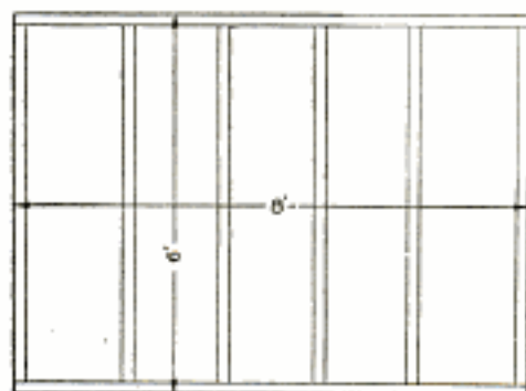
Floor Plan in Which the Two Sills are Shown Spiked to the Ends of the Joists
