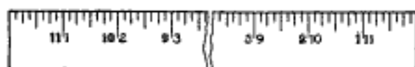
The Numerals Marking the Inches on a Rule Run Consecutively Beginning from Both Ends
