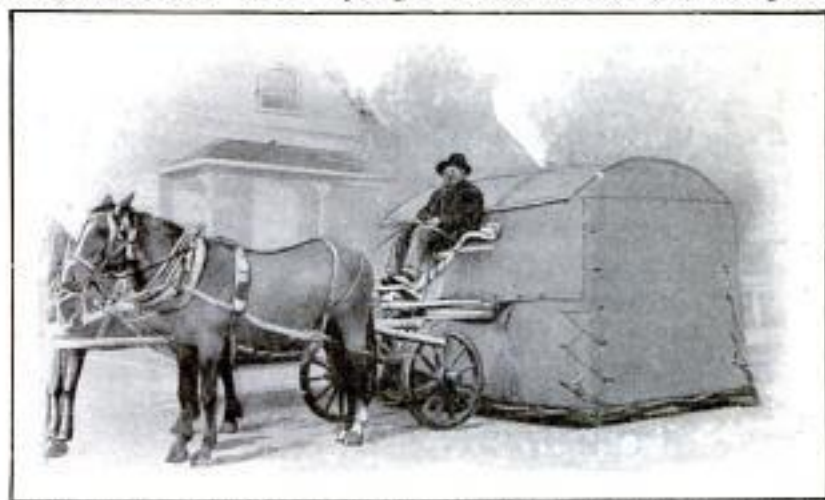
The Canvas Housing on the Rear of the Street Sweeper Keeps the Dust from Flying
