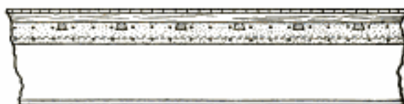
Wood Strips Molded in the Concrete to Make Holders for the Flooring Nails
