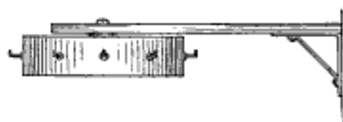
The Hook Support Revolves so as to Make Each One Readily Accessible for Hanging Utensils
