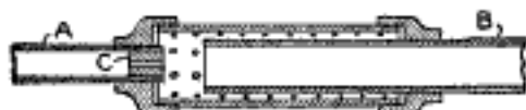
Cross Section of the Ejector Which is Made Entirely of Pipe and Fittings
