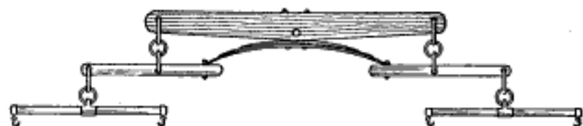
An Old Buggy Spring is Fastened to the Center of the Doubletree So That the Ends will Engage the Arms to Which the Singletrees are Fastened
