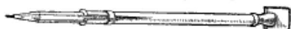
A Hollow Tube Receives the Whole Pencil, Which can be Used Up to the Last Bit
