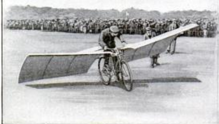
M. Moulin's "Flying Bicycle" in an Ineffectual Attempt to Leave the Ground. The Planes of This Machine are Mounted Exceptionally Low. No Amount of "Knee-Grease," would Raise the Machine into the Air
