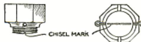
The Chisel Cut on the End of the Bolt Shows the Direction of the Hole
