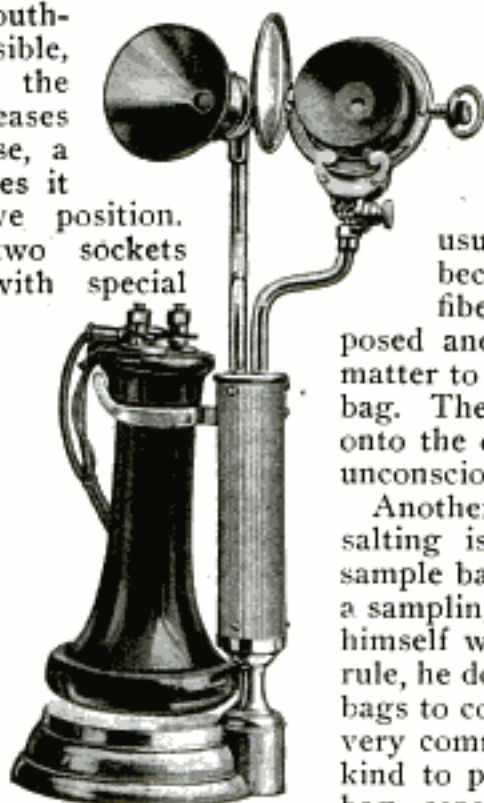
Watch-Case Telephone Transmitter Attached to Special Desk Phone
