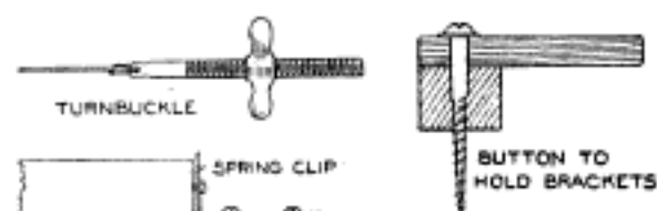
Detail of the Turnbuckle, Button to Hold the Brackets, and the Spring Clip for Holding the Legs on the Side of the Box
