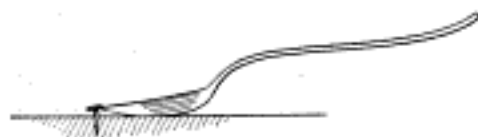
The Point of a Spoon will Easily Pull a Tack from Soft Wood
