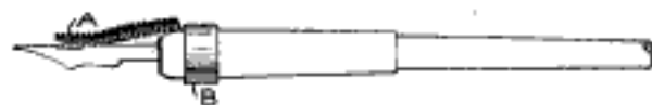
The Flow of Ink can be Regulated by Sliding the Wire on the Pen
