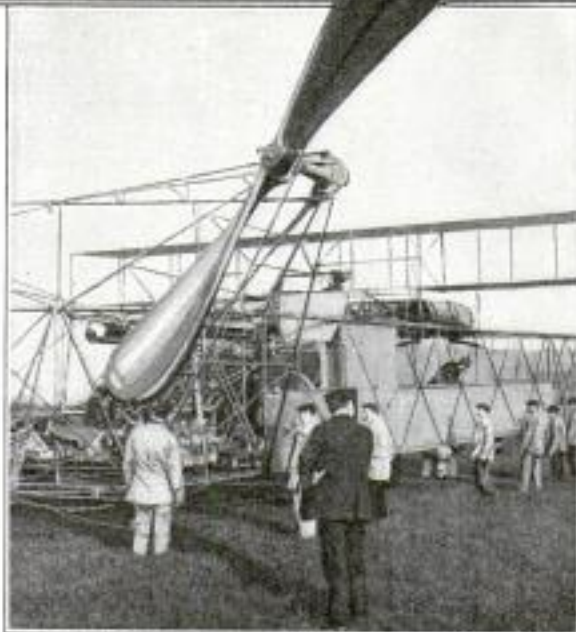
Carrying Portion of the Car, Showing One of the Propellers and the Motor Arrangement
