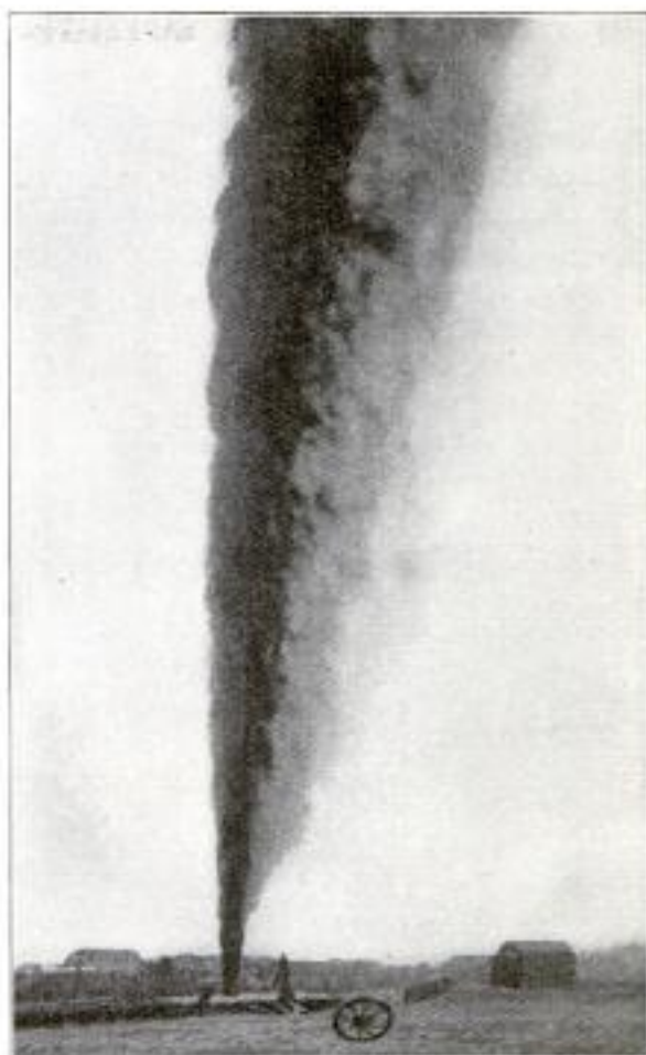
A Mexican Oil Well Which Has a Capacity of 110,000 Barrels per Day
