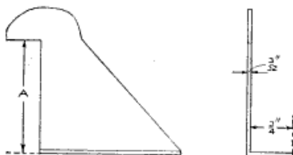
The Gauge is Used on Top of the Tool-Post Slide, to Set the Lathe Tool
