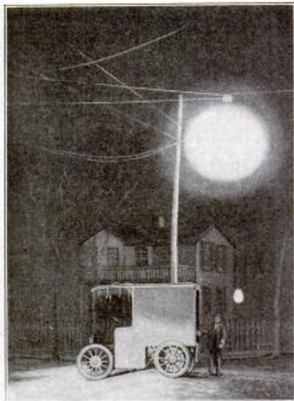
Electric Truck Feeding a Street Lamp with Current as a Means of Demonstrating Electric Street Lighting to an Ohio Community
