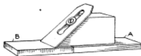
Plane Iron on a Block Having the Proper Slope for the Angle of the Edge
