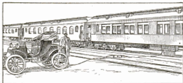
An Electric Automobile Furnishing Current to Light a Special Train, Side-Tracked at the Savannah Automobile Races
