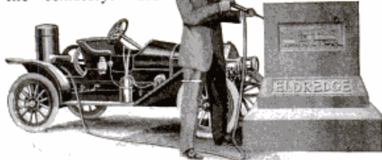
Chiseling a Monument by Means of an Automatic Tool Driven by Air Compressed by the Automobile Engine
