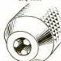
Chuck body is steel, polished and nickel plated. Jaws of steel, drop forged and hardened. Capacity 3-16 in.
