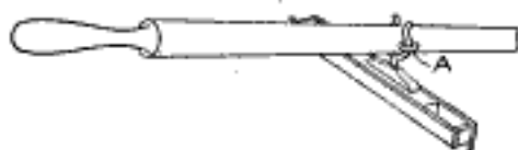
The Screweye in Position on the Oar and over One Prong of the Oarlock
