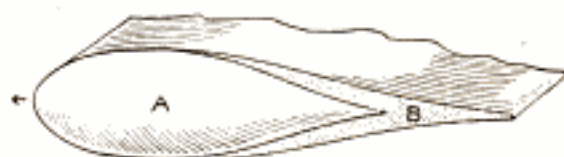
Fig. 5—Side view of streamline body A compared with streamline section B, showing the shortening of the former to secure equivalent effects.
