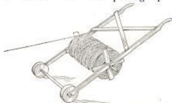
Fence-Wire Truck, Similar to a Baggage Truck with a Rod between the Handles for the Spool
