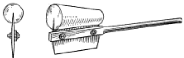
The Wafer Blade Attached to the Handle, the Top Edge being Protected with a Cork
