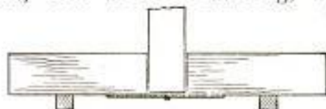
The Weight of the Door Causes the Holder to Grip the Edge Firmly
