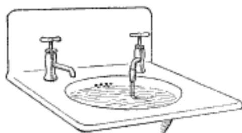
A Medicine Dropper on a Faucet Produces a Whirling Motion of the Water in the Bowl
