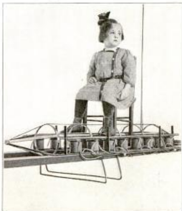
This Illustration Shows the Type in Which a Double Row of Electromagnets is Utilized. The Child is Seated in a Chair Placed on an 18-Foot Model Car, the Whole Being Suspended in the Air by the Action of the Electromagnets. Notice Space between the Tops of the Electromagnets and the Aluminum Plates
