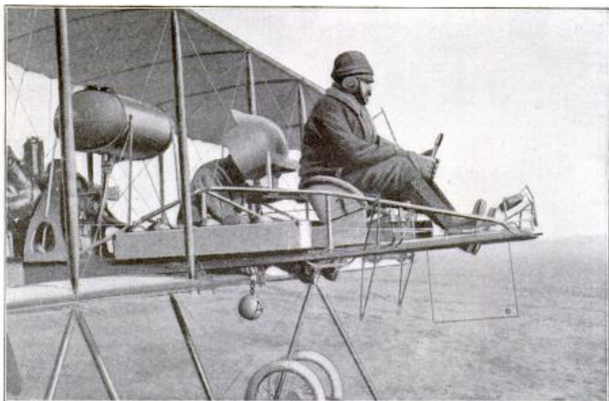
Lieutenant Bousquet in His Biplane. The Officer Who Drops Bombs is Protected by a Windshield, and on Each Side of Him are Ammunition Boxes
