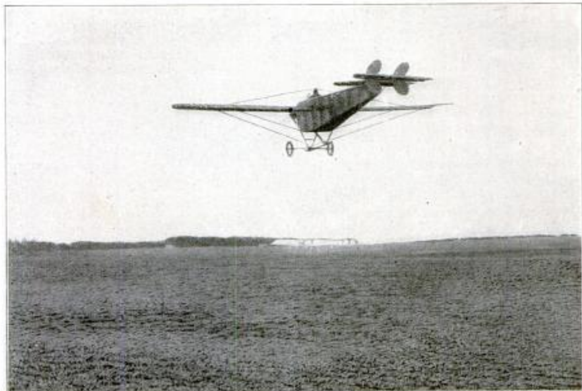
Fig. 2—The "reaction impulse" made visible on a Nieuport 20-hp. monoplane in the air, with the body fabric deeply sagged under the pressure that is the heretofore undiscovered secret of the efficiency of the streamline form.
