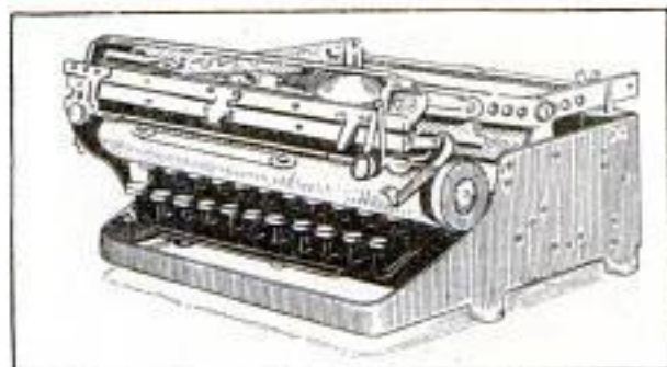
A French Visible Typewriter, the Carriage of Which Folds Forward over the Keyboard for Carrying
