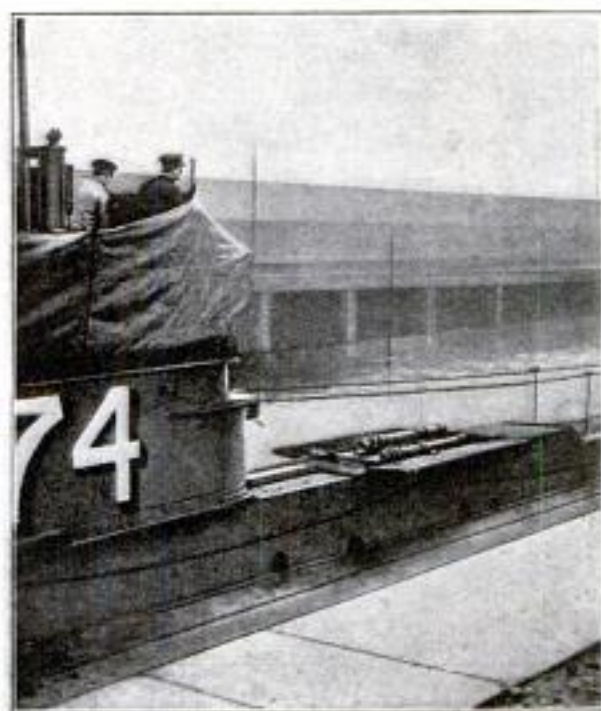
The Disappearing Quick-Firing Gun of Great Britain's Most Powerful Submarine being Raised through the Deck
