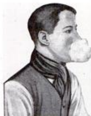
Courtesy Cassier's Magazine Simple Cotton Respirator Used for Many Years by Lancashire Cotton Workers
