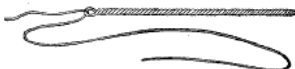
Needle of Twisted Wire
