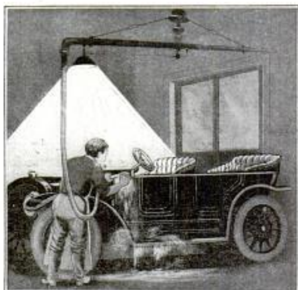
Revolving-Arm Automobile Washer with Electric Light
