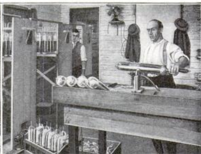
Glass Blower at Work Placing Samples of Standard Cotton in Vacuum Tubes
