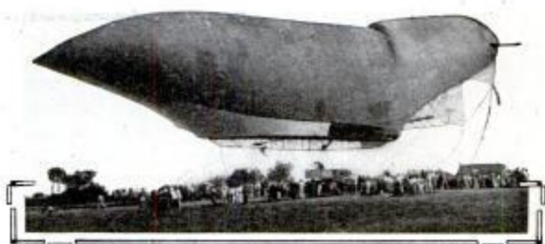
The French army dirigible "Republique" in incipient collapse because of the deflation of the interior ballonets which maintain tautness of the envelope by having air pumped constantly into them.
