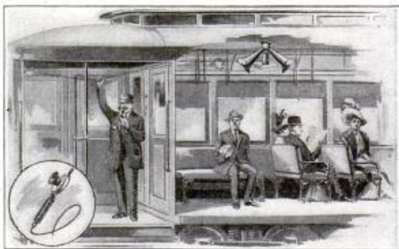
By Calling the Names of Streets through a Loud-Speaking Telephone Outfit, the Necessity of the Conductor Opening and Closing the Door as Each Street is Approached is Done Away With
