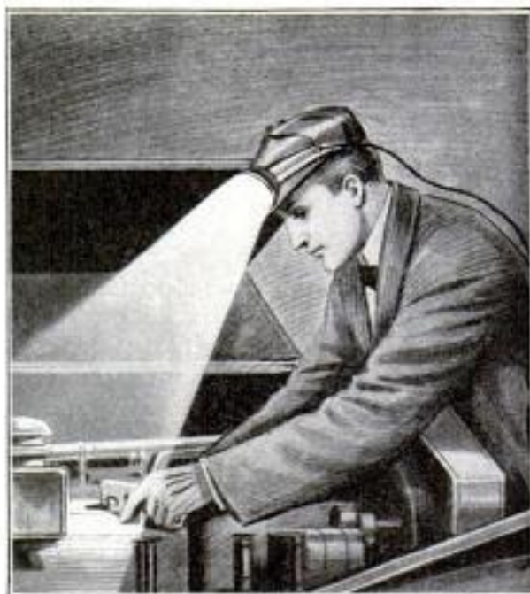
Working on the Engine under Illumination from the Head Lamp Leaves Both Hands Free for the Task
