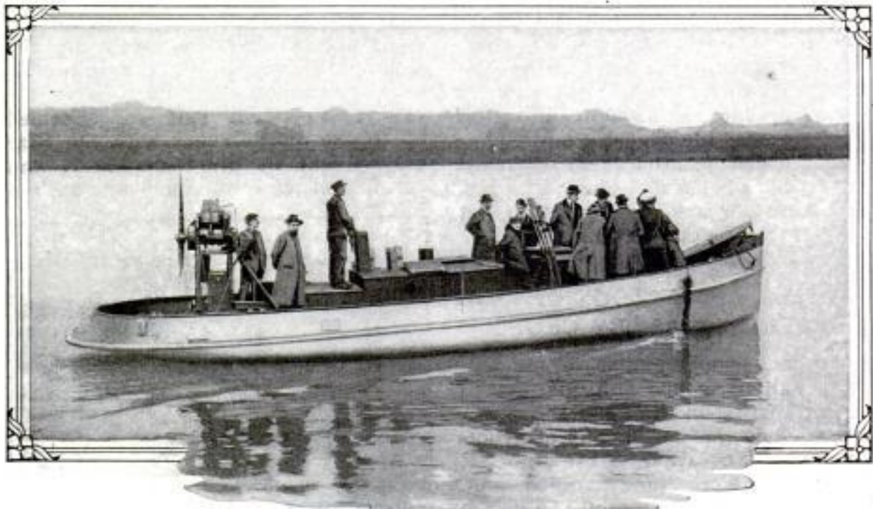
Shallow-Draft River Boat Driven by Aeroplane Propeller in Tests being Made in France
