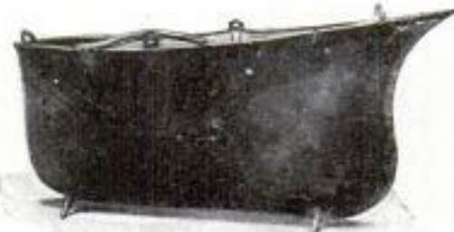
The first attempt at a dirigible. The car of the balloon used by Blanchard and Jeffries, in their crossing of the English Channel on January 7, 1785, in a favoring wind. It was attempted to propel this balloon by the use of large fan-like oars but this expedient naturally proved a complete failure, and the wind became the sole means of propulsion.
