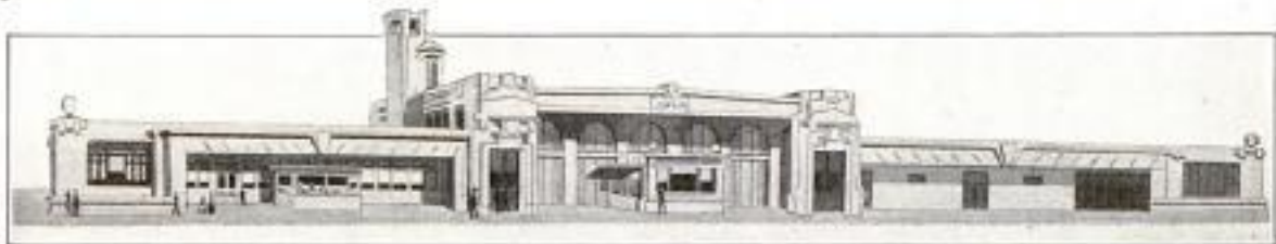
Waste from the Zinc and Lead Mines of Joplin, Mo., Went into the Construction of This Reinforced-Concrete Union Station
