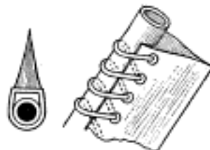
Suggested Method of Building up Aeroplane Struts to Secure Streamline Reaction against the Latter
