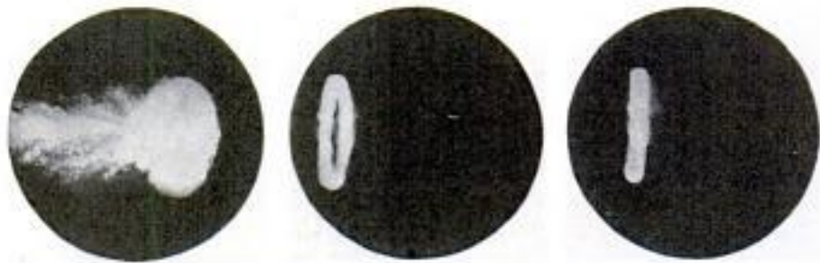
Projecting the Fluid Rings—The Drawing on the Left Shows the Operation of the "Gun," and Manner in Which Rings are Formed: Box A, Containing Colored Solution, is Struck by Hammer at Diaphragm B, and Fluid is Forced Out of Opening C, with Whirlpool Motion, Which Creates Ring—Other Views Show Progress of Ring
