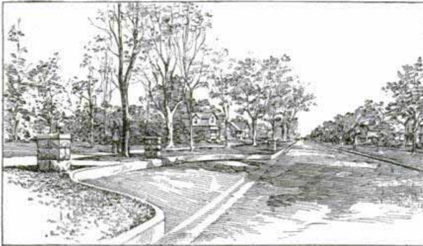
Inset Section of Roadway to Prevent Obstruction of Traffic by Vehicles Stopped before Houses
