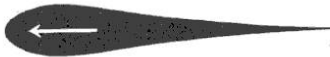
Fig. 1—Streamline Form Best Adapted to Movement through a Fluid with a Minimum Resistance
