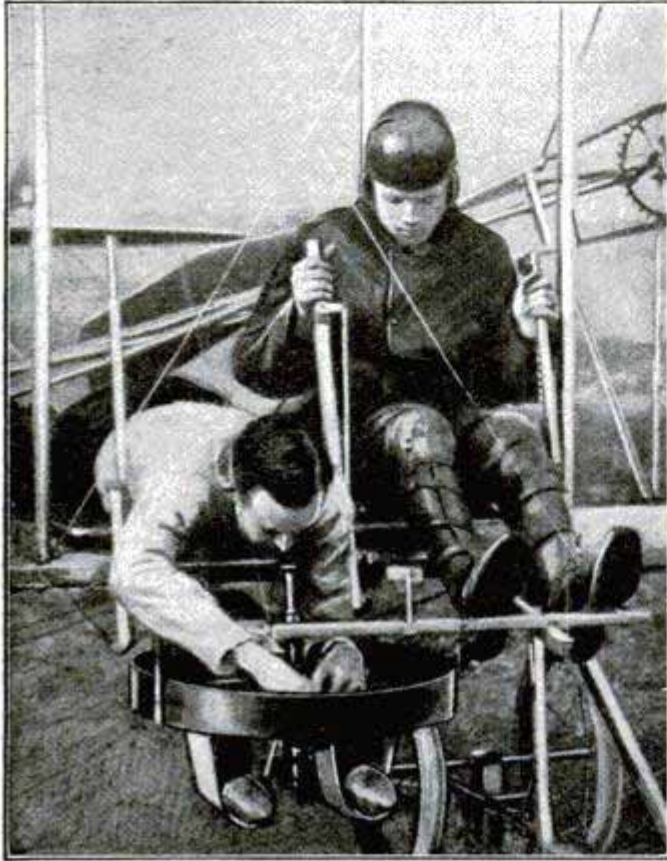
Starting on a Test Flight with Bomb-Dropping Device which Takes Scientific Consideration of All the Factors Such as Height, Speed, Etc., Necessary in Determining at What Moment a Bomb should be Dropped to Strike the Desired Object
