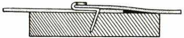
Manner of Using New Roofing Nail
