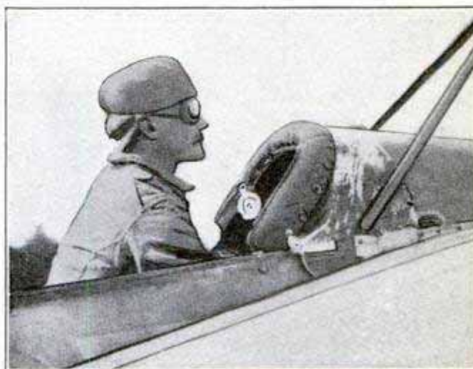
Pneumatic Buffer Immediately in Front of Driving Seat of M. Vedrines' Monoplane
