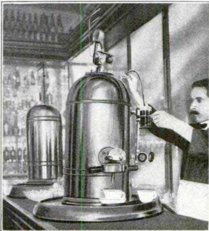
A Restaurant Coffee Device by Means of Which the Coffee is Not Heated until Ordered, and Then Only a Cup at a Time
