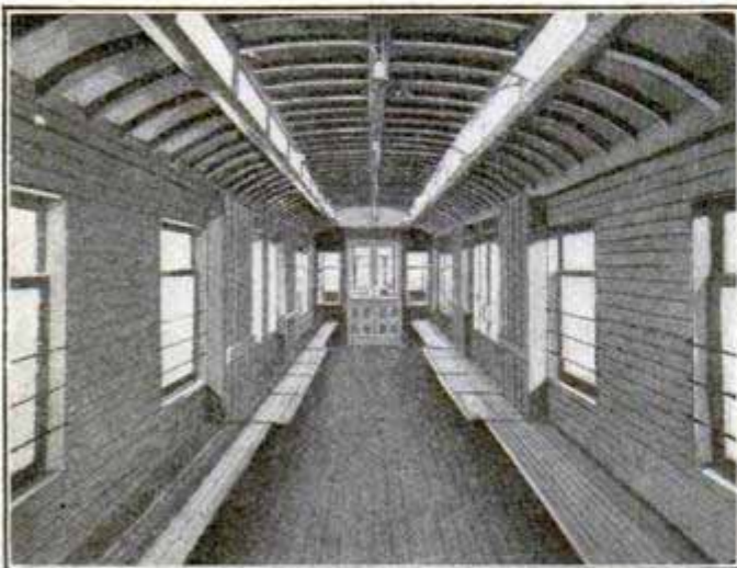
An Electric Car Which may be Used for Either Freight or Passengers, the Seats Folding against the Walls When It is to be Used for Freight
