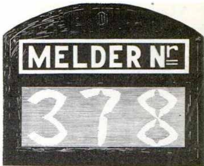
Indicates that Fire-Alarm Box No. 378 Has Been Rung in the City
