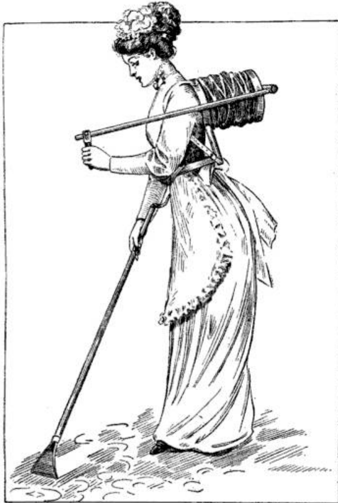
A Vacuum Cleaner Operated by Means of a Bellows Attached to the Back
