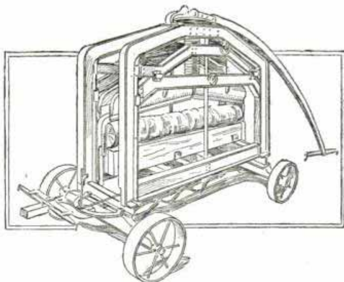
Portable Railroad-Tie Cutting Machine
