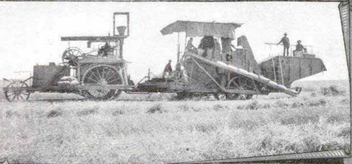
The Highest Development of Agricultural Machinery—the Traction Reaper-Threshing Machine Which Takes the Grain from the Ground and Threshes It, Getting Both Locomotion and Power from a Gasoline Engine
