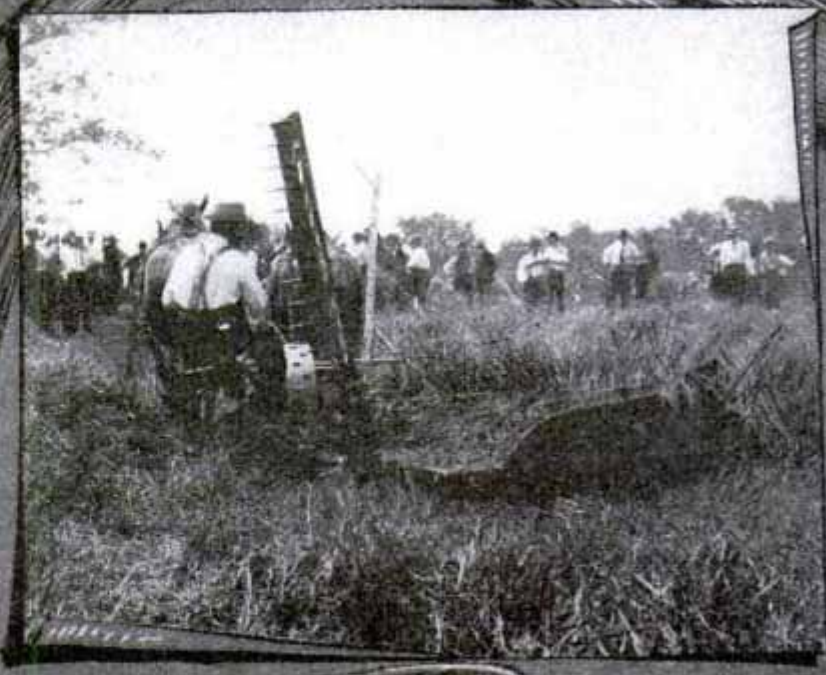
The First Horse-Drawn Reaper, Which Simply Cut the Grain
