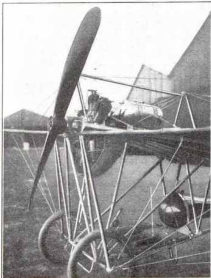
The Gnome Motor Fitted on "Demoiselle" for First Time, Replacing Horizontal Opposed Motor
