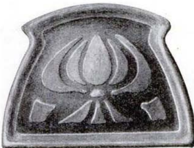
Conventional Designs for Book Ends — The Lower Design Requires Considerable Hammer Work, as the Outer Edge is Bent Over and Hammered Down Around the Top and Sides, and the Center Portion is Beaten Out
