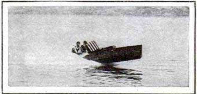
PRONTO III AT 28.07 M. P. H. WITH HER 6 CYL. 60 H. P. ROBERTS
