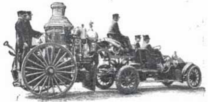
Ordinary Automobile Used in Converting Horse-Drawn Fire Engine into Motor-Driven Machine
